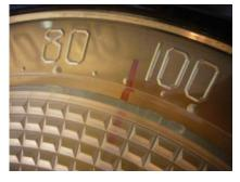
where the antenna really resonates. The rightmost mark is 1600kHz, but that's odd, because you trim the oscillator at 1620. Then you back down to about 1500 to trim the antenna and mixer.
