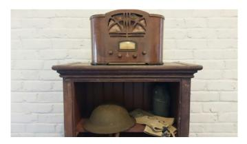
This set was an Emerson 107 U6F, also interestingly the same year as the Airline, and both found in Rider volume 6. This three band AC-DC 6 tube, not counting the ballast to reduce line voltage, was advertised as the "Duo-Vox". The model number is the 3 letters before the dash in the serial number.
