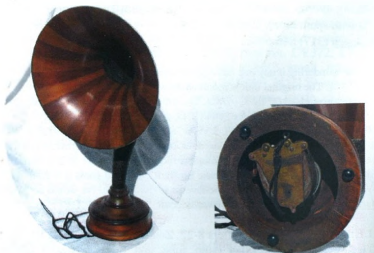
A thick base version using a large driver arm reproducer. No manufacture's name on the reproducer. Horn is identified as manufactured by the Radio Cabinet Company, Indianapolis.
