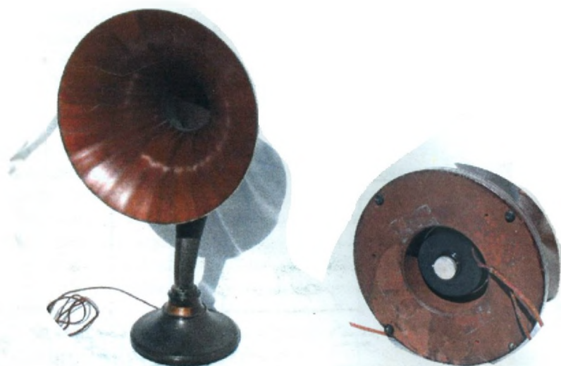
A shallow base version using a smaller driver arm reproducer, manufactured by J. S. Timmons, Philadelphia. Horn is identified as manufactured by Bremerman & Son's, Indianapolis.
