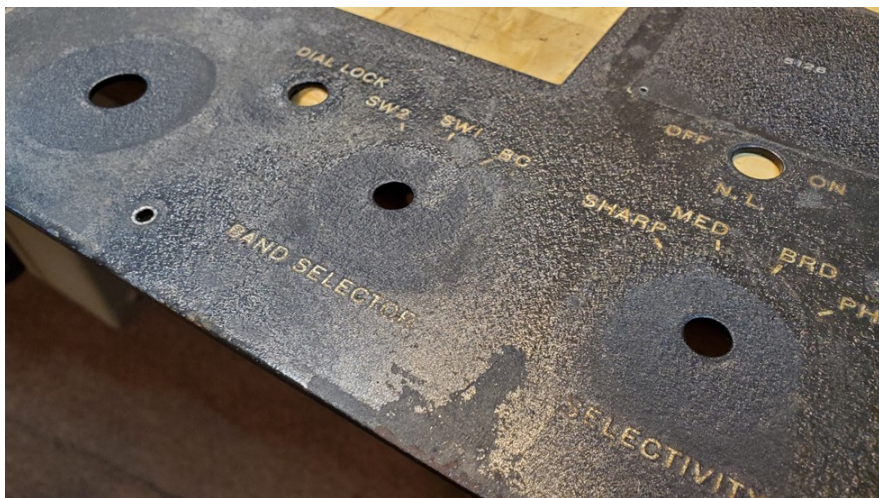
The faceplate, showing a well preserved original black texture paint with a yellow MFP like film over it.
