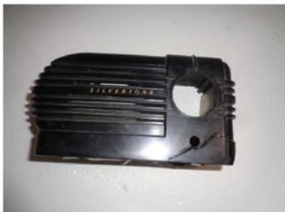
The next step was to super glue the pieces back in place and make sure they were properly aligned. After that I put quick-set JB Weld underneath and along the cracks. I let it set for a couple of hours and allowed the JB Weld to fully cure. I created a valley along the cracks on top of the cabinet with a Dremel tool's pointed grinding bit.
