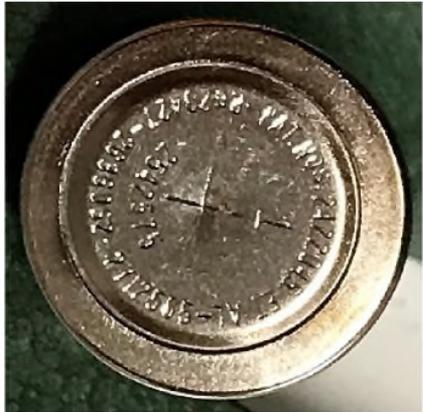
One of the audio transistors had been replaced at a later date with a (1954 date code) 2N35.
