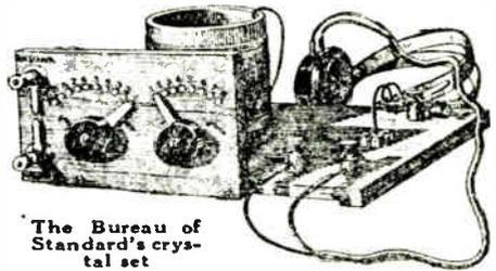
post—the lower one—to the left-hand switch arm, and connecting the upper binding post—the aerial—to the right-hand switch arm. All that now remains are the detector, condenser, and the binding posts for the telephone.
