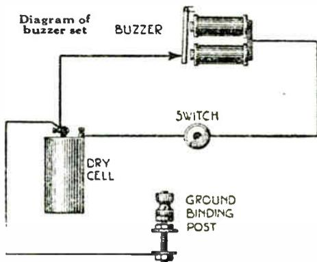
the crystal is in good adjustment, a loud buzz will be heard in the phones when the buzzer is operated. If the buzz is heard in the set, then wireless signals within the range of the set will also be heard.
