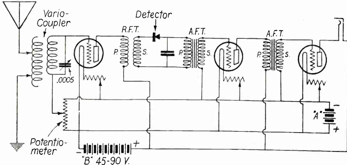
CIRCUIT NETWORK of a high-quality receiver, comprising a stage of RF, crystal detector and two stages of AF. Its tone quality on a speaker is superb and it is one of the most satisfactory receivers that can be built. It is not a great DX-getter.
