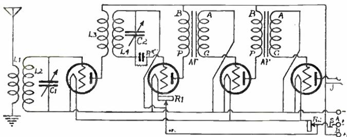
FIG. 3.—The wiring diagram for Caldwell's 4-tube set, consisting of one stage of radio-frequency, detector and two stages of audio-frequency. Radio-frequency transformers are basket-wound, low-loss type. The use of low-loss condensers increases the efficiency to make this set almost the equal of a 5-tube receiver.
