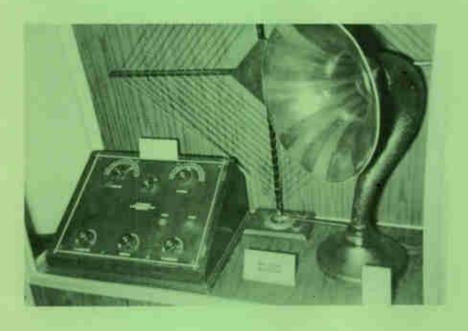
A 5 tube Lyradion Loop receiver made in Mishawaka, IN in 1925, very rare, two stages of RF, a detector, and 2 audios.
