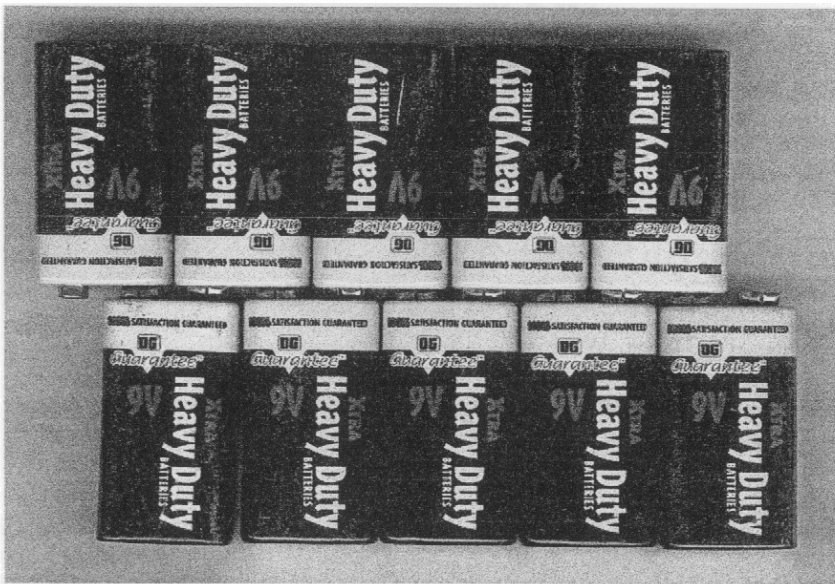
10 inexpensive 9 volt batteries make up this 90 volt battery pack.
