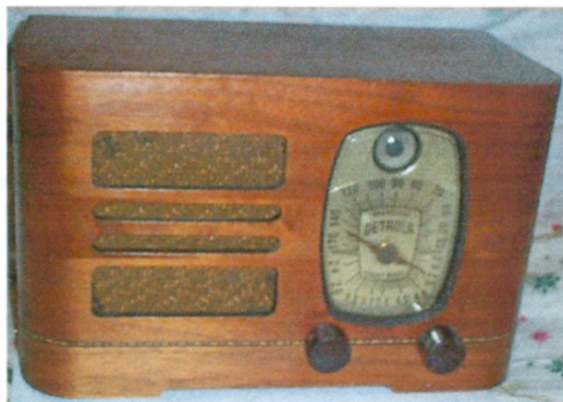
Front and rear views of the Detrola 212 with the 1629 tuning eye.
