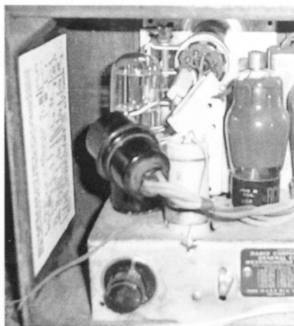
Front and rear views of the Detrola 212 with the 1629 tuning eye.
