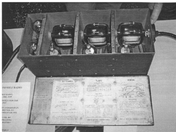
Interior view of Joe Scott's 1930 Delco Cadillac car radio
