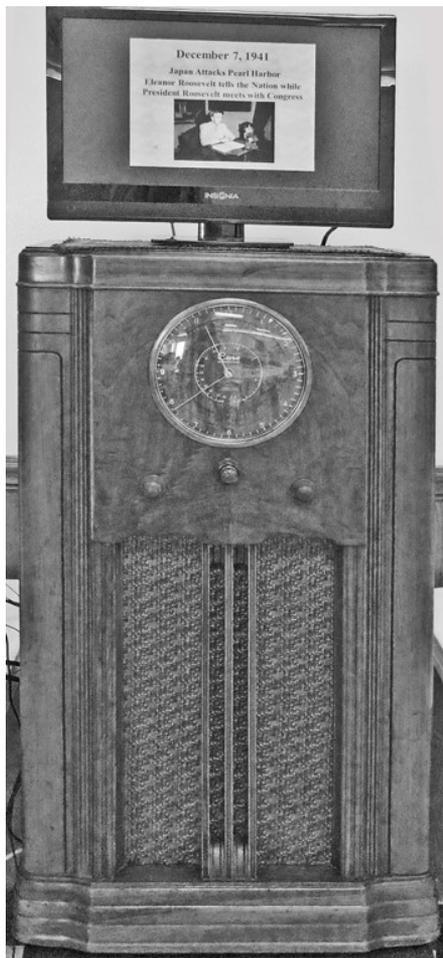
The CASE entered in the IHRS 2018 Spring Meet Old Equipment Contest is identified as a Marion, Indiana radio product. This Case is model 722, chassis 17 with a “Tell Time Tuning” dial. This is a seven tube multiband receiver.
