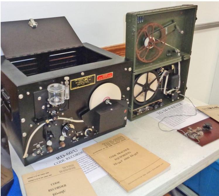
Bill Smith entered an operating RD-60/U Recorder and TG34A Keyer in the Open category. The RD-60/U is a paper tape recorder of radio signals used in conjunction with code practice equipment and training equipment. The TG-34-A is an automatic unit for reproducing audible code practice signals previously recorded in ink on paper tape.
