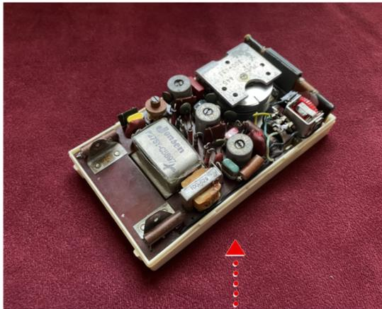
The TR-1 used many new miniature components ranging from Vokar 262kHz IF transformers, R/C tuning capacitor and a Jensen 3" speaker.
