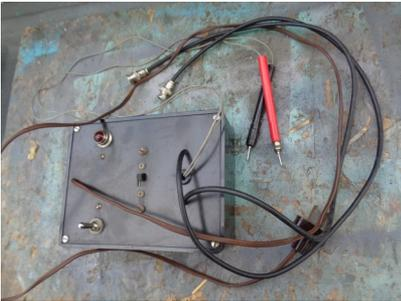
The power cord is one lead. Another lead goes to an oscilloscope's vertical input and another lead goes to the horizontal input. The two remaining leads are the test leads that are applied to the semiconductor or part under test. When I worked for Heath, they introduced me to the octopus and they gave me the parts to build one. I was told it would speed up servicing equipment and it did.
