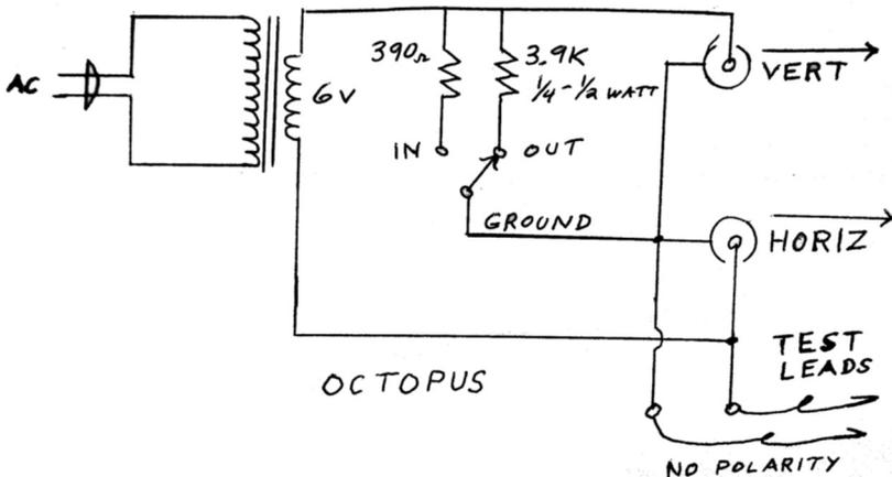
in the out of circuit position with the higher resistance. Components that I do not test out of circuit are static sensitive parts such as IC's and transistors. At Heath, I was testing circuit boards so all of my testing would be in-circuit tests that could include static sensitive parts. Since 1979, I never had a problem with the octopus killing static sensitive components. In fact, I have never had it destroy ANY components .
