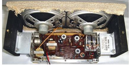
The battery holders had some serious areas of crusty corrosion residue on the aluminum which had to scraped off. After removal, polished those spots the best I could with fine Scotchbrite and Windex. Turned out pretty well... Neat that they still had the manufacturer's stickers on them---ACME of Brooklyn, NY. Replaced the wiring which had been "modified" at some point in past.
