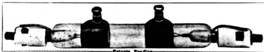
Fig. 1 The Tigerman detecto-amplifier tube.
