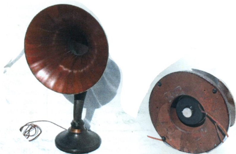
A shallow base version using a smaller driver arm reproducer, manufactured by J. S. Timmons, Philadelphia. Horn is identified as manufactured by Bremerman & Son's, Indianapolis.
