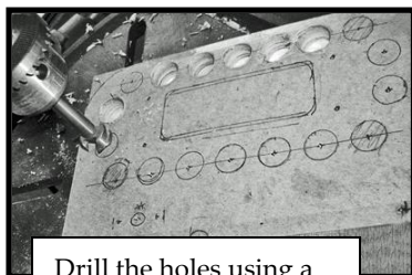
Drill the holes using a Forstner bit.
