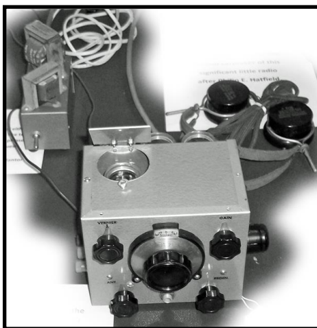
The original Hatfield one tube regenerative receiver used in the January 1963 issue of Popular Electronics. Upper left is the power supply, the frequency tune coils are stored on the back of the receiver.
