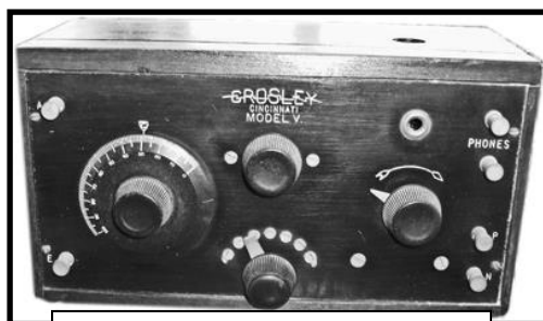
The 1922/23 Crosley Model V – A Regenerative receiver – licensed under the Armstrong patent. This set uses a variocoupler with a cylinder tuning coil.
