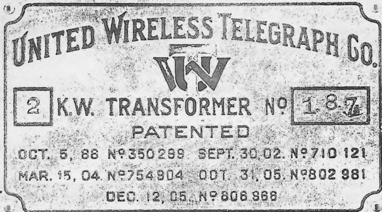
YOU REAL OLD-TIME COMMERCIAL OP'S SHOULD RECOGNIZE THIS ONE! REMEMBER HOW YOU HAD TO PRY THE LID FROM THE 2 KW "COFFIN" AS IT WAS DUBBED, WHEN AN INTERNAL FLASH-OVER IN THE 20,000 VOLT SECONDARY BURNED OFF A CONNECTING WIRE IN ONE OF THE SECONDARY 'PIES'?
