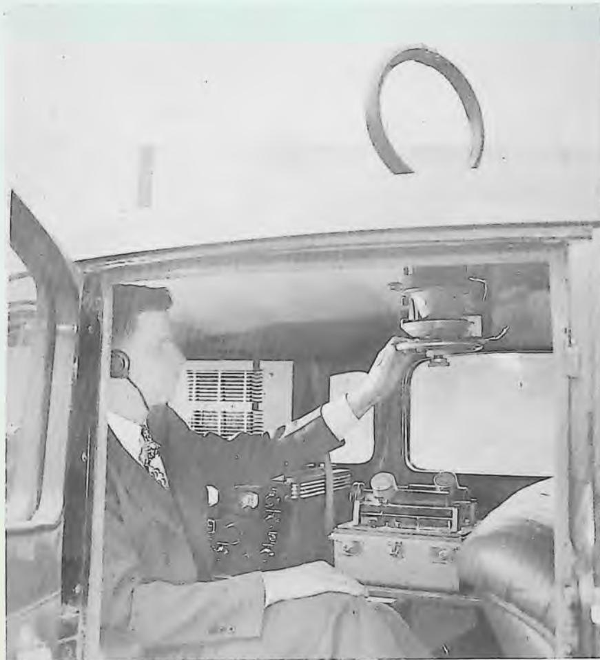
AN INTERIOR VIEW OF AN RID PROWL CAR USED TO INTERCEPT SIGNALS AND LOCATE SOURCES OF INTERFERENCE. LOOP DOES NOT SHOW WHILE CAR IS CRUISING BUT ONLY WHEN TAKING A BEARING. NOTE SX28 RECEIVER AND DICTAPHONE RECORDER; OTHER RECEIVERS IN CAR COVERED 75 KC TO 300 M.
