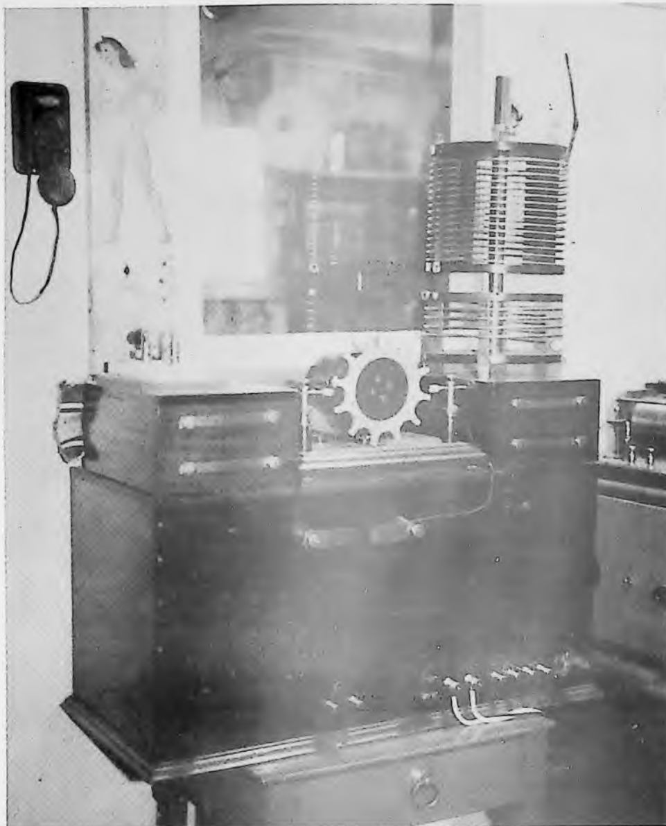
1½ K.W. SPARK TRANSMITTER VINTAGE OF 1912
