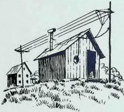
Overhead we can look up and see long, gleaming strands of copper wire hung between wide spreaders on huge poles. A fan-lead-in comes down and connects to the wall insulator in professional fashion.
