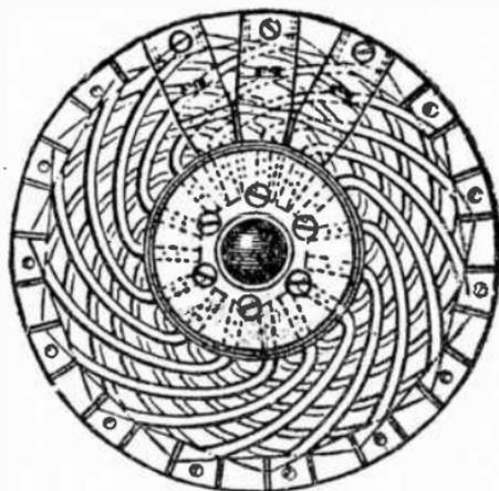
FIG. 806.—Siemens' bar armature; end view. *Each inductor* in the form of a bar is connected to the next by means of two evolute spiral copper strips, one bending inwardly, the other outwardly, their junction being in some cases secured to a block of wood upon the shaft. Their outer ends are attached to the bars by rivets or silver solder.
