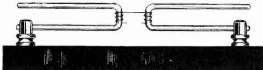
FIG. 4,020.—Action of flat horns neutralized.
