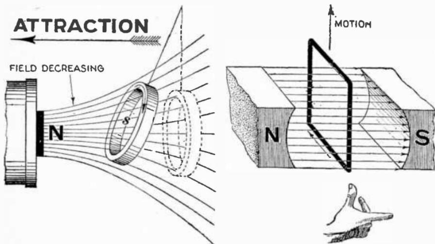
FIG. 2,923.—Repulsion motor principles 5. A copper ring is attracted to a magnet pole when the number of lines of force passing through the ring is decreasing. See fig. 2,920.
