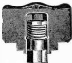
FIGS. 4,071 to 4,073.—Diamond snap switch handle. Fig. 4,071 external view of handle; fig. 4,072, spring in normal position; fig. 4,073, spring compressed.
