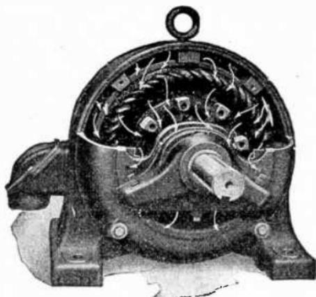
FIG. 2.815.—Sectional view of Wagner internal resistance motor showing directed draught ventilation.
