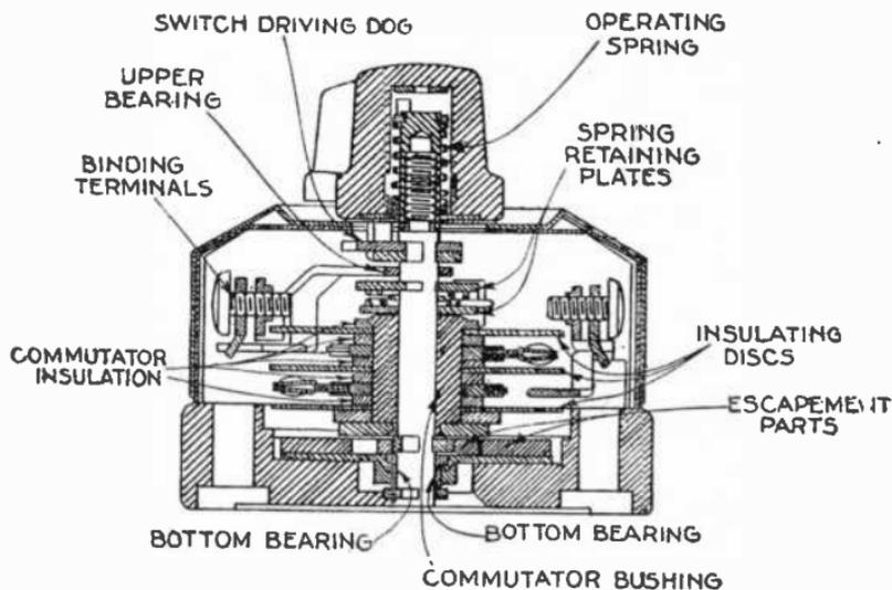
FIG. 4,082.—Sectional view of Bryant heater switch.
