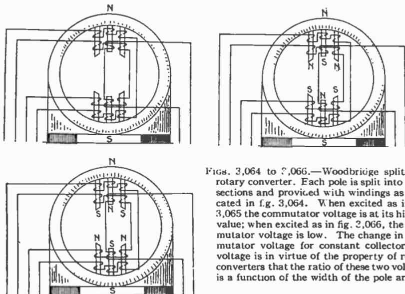
Figs. 3,064 to 3,066.—Woodbridge split pole rotary converter. Each pole is split into three sections and provided with windings as indicated in fig. 3,064. When excited as in fig. 3,065 the commutator voltage is at its highest value; when excited as in fig. 3,066, the commutator voltage is low. The change in commutator voltage for constant collector ring voltage is in virtue of the property of rotary converters that the ratio of these two voltages is a function of the width of the pole arc.
