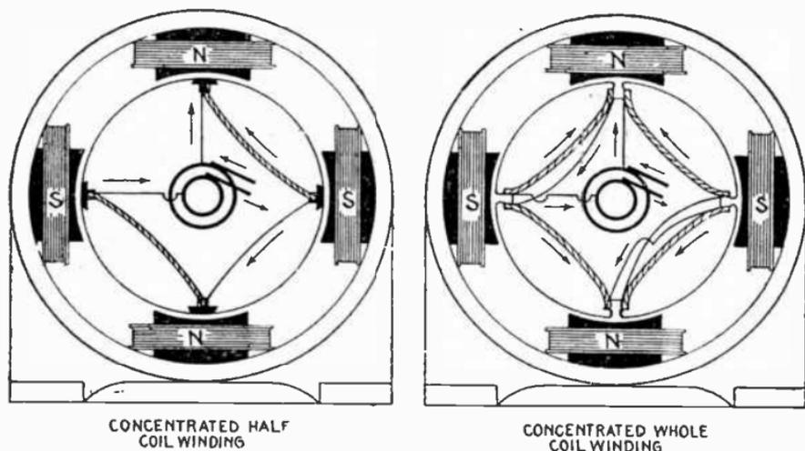
**Figs. 3,104 and 3,105.**—Concentrated windings. A concentrated winding is one in which the armature has only *one tooth per phase per pole*, that is, the number of teeth equals the number of poles. A concentrated winding of the half coil type has only one side of a coil in each slot as in fig. 3,104. In the whole coil variety, each slot contains neighboring sides of adjacent coils, as in fig. 3,105.
