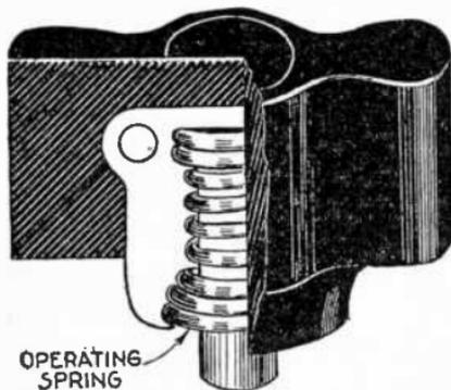
FIG. 4,058.—H & H switch self adjusting handle.
