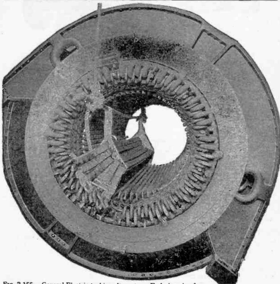
FIG. 3.155.—General Electric turbine alternator. End view showing end of armature winding and method of raising coils for inserting fast coil.
