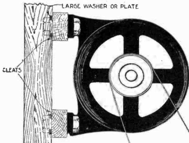
FIG. 3,938.—Method of mounting motor on wooden wall.
