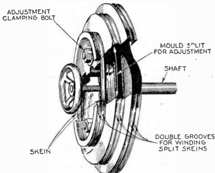
FIG. 3,178.—Winding head for winding skeins. The double grooving permits winding two skeins of the same size or one split skein. When the skein is over  $\frac{1}{4}$  in. square and of wire larger than No. 19, it should be wound in two sections. Note that the winding mould is split through the center so as to be adjustable for different sizes of skeins.
