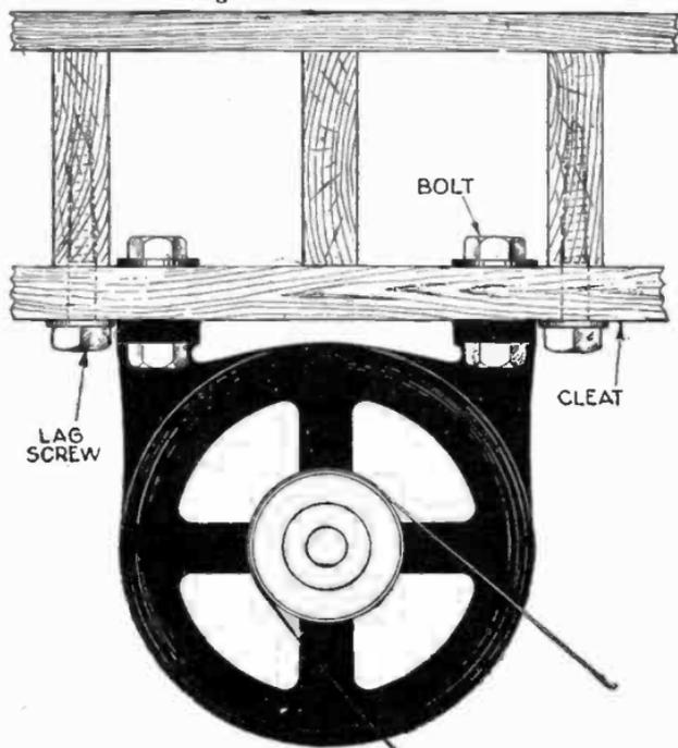
FIG. 3,939.—Method of mounting motor on wooden ceiling.
