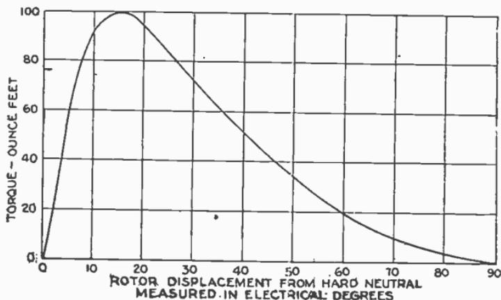
FIG. 3,003.—Locked torque of repulsion motor.
