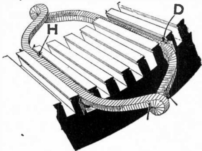
FIG. 3,216.—Coil grounded on core. Should two grounds occur simultaneously, as for example at H, and D, a short circuit would be formed in the loop, and if the normal voltage remained on the motor, this short-circuited turn would immediately become hot enough to destroy the insulation on the complete coil.
