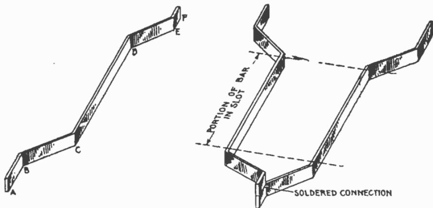
FIGS. 3,126 and 3,127.—Bent bar inductor and method of connection with soldered joint. Fig. 3,126 shows one bar and shape of bent ends. The portion from C, to D, is placed in the slot; B, to C, and D, to E, bent or connector sections; A, to B, and E, to F, ends bent parallel with slot for soldering. Fig. 3,127 shows two bar inductors connected.
