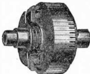
FIG. 2,991.—Baldor fractional horse power single phase repulsion start induction motor commutator showing sectional view of the short circuiting switch. This switch is designed for rolling contact to render it self-cleaning.
