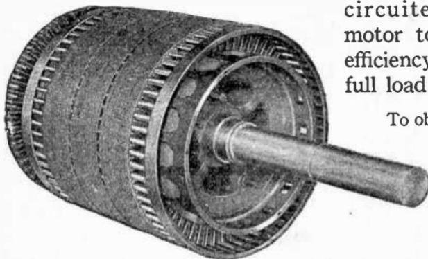
To obviate the complications of the external resistance motor, the double squirrel cage motor is used. The maximum torque and the starting current in all squirrel cage motors bear a more or less definite relation to each
