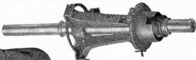
FIG. 2,849.—Century split phase induction motor governor weights which operate cut out switch.
