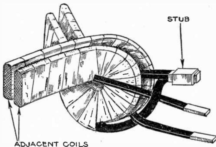
FIG. 3,224.—Stub or connection between adjacent coils.
