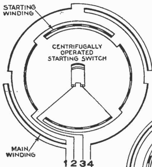
FIG. 3,197.—Diagram showing series connections of four pole motor. *Clockwise rotation:* Connect 1 and 2 to one line; connect 3 and 4 to other line. *Counter clockwise rotation:* Connect 1 and 3 to one line; connect 2 and 4 to other line.
