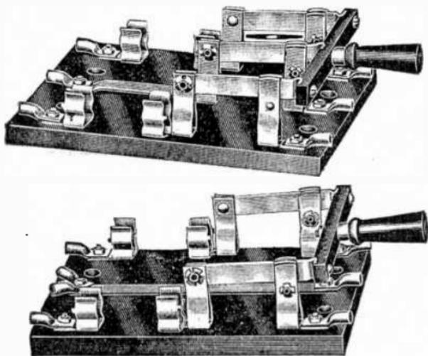
FIGS. 4,053 and 4,054.—Lyons solid neutral type switches. In fig. 4,053 a removable solid neutral bar is used in place of the usual fuse connections. This construction permits removal of the solid neutral bar and replacing in its stead the regular fuse clips, if desired. In the construction shown in fig. 4,054, a solid strap is used terminating at both ends in a line parallel with back and front connections. This permits somewhat easier handling because of the omission of one working pole.
