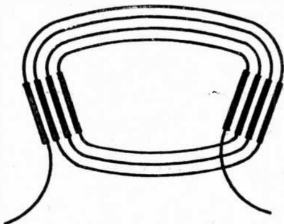
FIG. 3,149.—Diagram showing a spiral coil. This type of coil is one in which each successive turn lies entirely within the previous turn, starting with the outermost turn of the coil. The successive turns of a spiral coil are thus not of the same size, and are not overlapping as in a "lap" coil.
