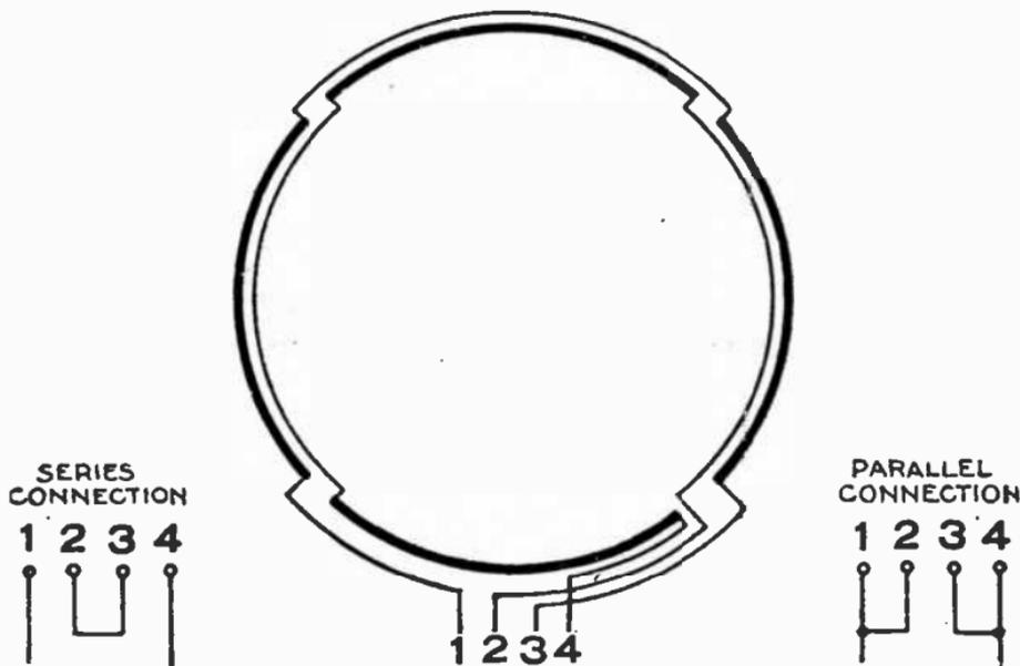
FIGS. 3,193 to 3,195.—Diagrams showing connections for winding in fig. 3,202.
