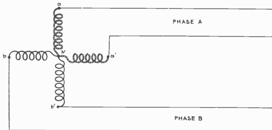
FIG. 3,158.—Diagram of two phase star grouping.
