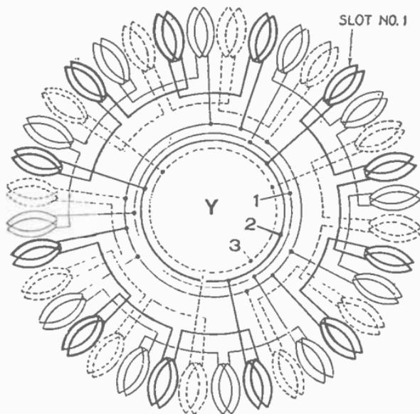
FIG. 3,282.—2 phase, 12 pole, 3 circuit Y.
