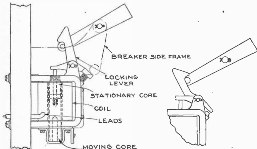
FIGS 4,173 and 4,174.—Westinghouse carbon circuit breaker electric lockout attachment. There are times when it is desired to lock a breaker in the open position when certain conditions exist. For this purpose a lockout attachment is provided which either latches the breaker open or else interposes an arm which opposes the movement of the brush. Depending upon requirements the coil may lock the breaker open when energized or it may be so arranged as to lock the breaker open when de-energized.
