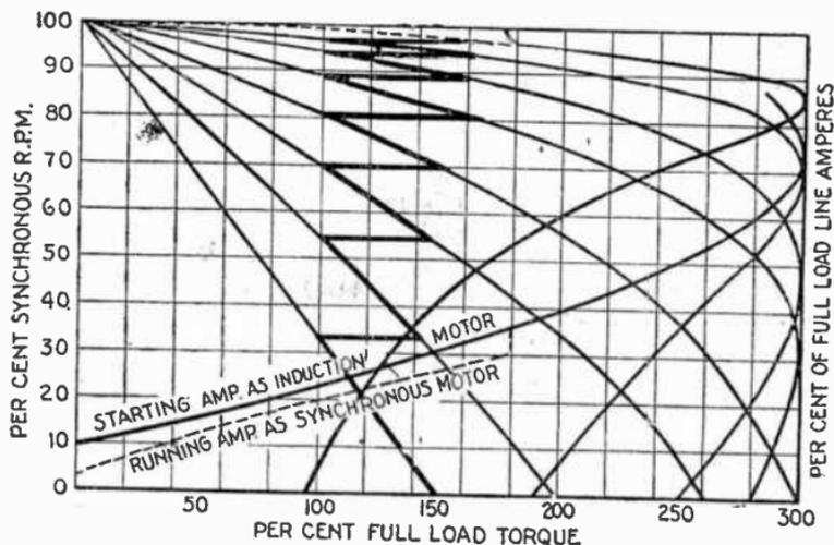
FIG. 3,016.—Fynn-Weichsel motor starting characteristics. *It will be noted* that the average current required during the starting period at full load torque is equal to 1 to 1.5 times normal full load running current.
