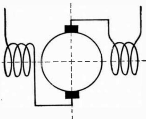
FIG. 2,899.—Diagram of single phase series commutator motor. It is practically the same as the series direct current motor, with the exception that all the metal of the magnetic circuit must be laminated.
