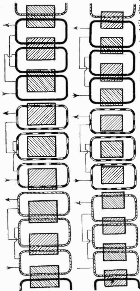
FIGS. 3,150 and 3,151.—Diagram of creeping windings. Fig. 3,150, nine coils subtending ten poles; fig. 3,151, nine coils subtending eight poles.
