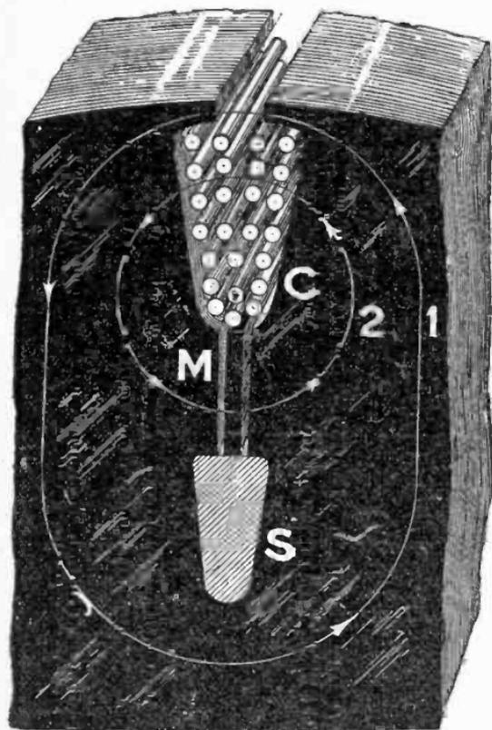
The cage winding is located in slots below those which contain the commutated winding. The slots which contain the two windings may or may not be connected by a narrow slot. Usually there are the same number of slots in the two windings. It is not, however, absolutely essential that they be the same, as before stated.
