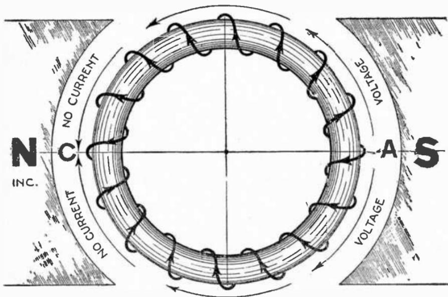
FIG. 2,969.—Wound ring in *a.c.* field showing direction of pressures induced in the inductors by transformer action. In this and accompanying cuts, induced pressures and currents are assumed to be in phase with the field flux. As shown, the induced pressures starting from A, traverse both halves of the winding to the point C, indicated by the arrows. Since the pressures induced in one half of the winding are equal and opposite to those induced in the other half, no current will flow.
