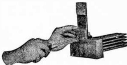
FIG. 4,131.—*How to assemble an air circuit breaker 2.* Attaching stationary contact plate to bracket.
