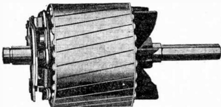
FIG. 2,858.—Domestic split phase induction motor armature complete.
