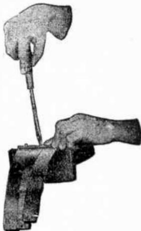
FIG. 4,133.—*How to assemble an air circuit breaker 4.* Method of attaching the laminated connection to the lower stud.
