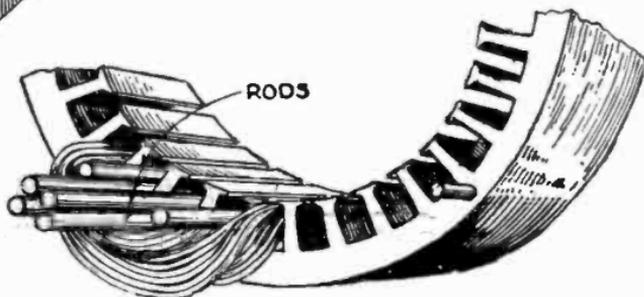
wound main windings are generally skein wound, although they too may be mould wound, but they should not be hand wound because the resistance of the starting winding is very important, and in the case of a hand winding, would vary too much.
