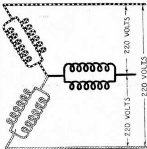
FIGS. 3,928 and 3,929.—Winding diagrams illustrating a 440 volt series star connected motor and reconnection for operation at 220 volts as described in the accompanying text.
