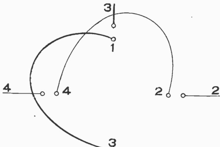
FIG. 3,243.—2 phase, 2 pole, 1 circuit.
