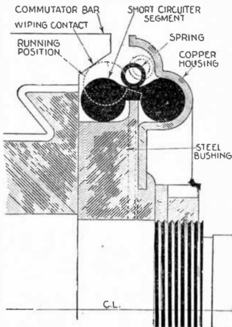
FIG. 2,993.—Master single phase repulsion start induction motor short circuiting centrifugal starting switch; built as a unit.
