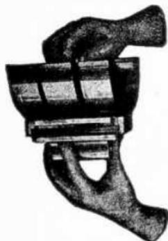
FIG. 4,140.—How to assemble an air circuit breaker 7. Method of fastening the brush support to the brush.
