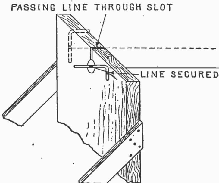
FIG. 3,941.—Method of securing wire center line.
