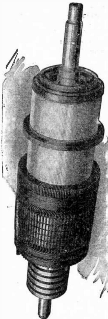
FIG. 3.072.—Armature of Allis-Chalmers 500 kw. 275 volt, 750 r.p.m., 6 phase, 25 cycle synchronous converter.
