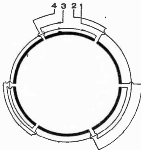
FIG. 3,207.—Diagram showing connections for a 2 pole repulsion-induction motor.
