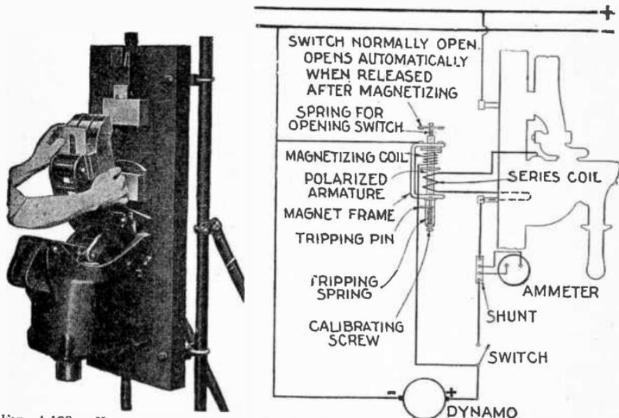
FIG. 4,190.—How to assemble an air circuit breaker 29. Adjusting brush for perfect contact condition.
