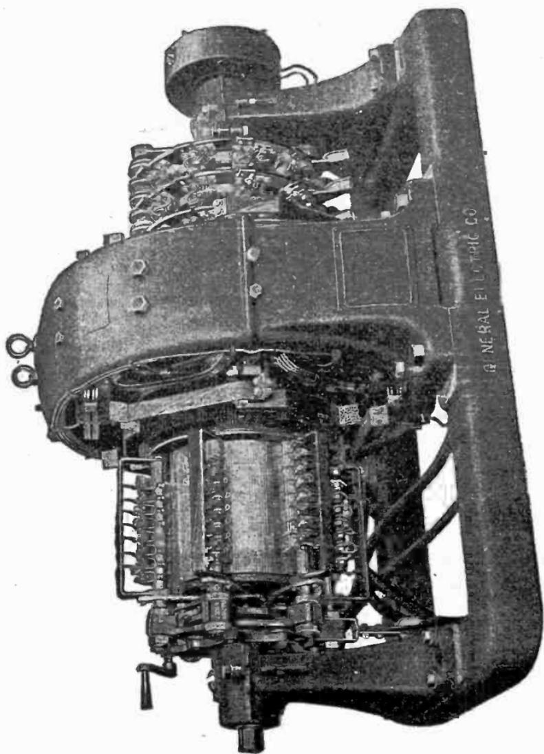
Fig. 3,096.—General Electric 300 k.w. synchronous converter for mining service. 275 volts. *d.c.* compound wound; 60 cycles 2,300 volts *a.c.*
