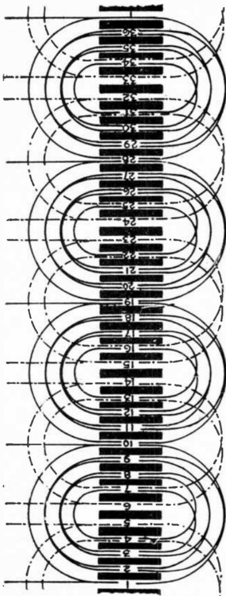
FIG. 2,196.—Diagram showing completed main and starting windings.
