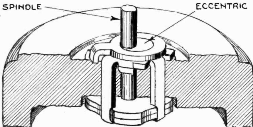
FIG. 4,057.—H & H snap switch shock resisting release parts mounted on porcelain base.
