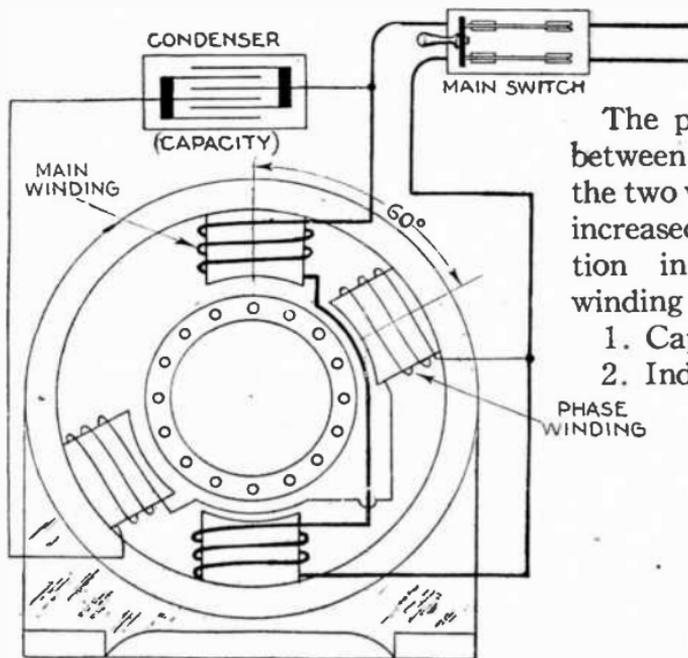
The phase difference between the currents in the two windings can be increased by the insertion in the starting winding circuit of
