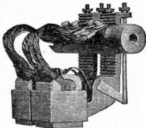
FIG. 3,050.—*Westinghouse synchronous converter construction 10. A.C. brush holder.* They are of the sliding shunt type arranged for mounting on a stud. The spring and tension adjusting mechanism being similar to that on the *d.c.* holder except that a thumb nut micrometer adjustment is employed, which gives an accessible and ready means of adjustment of brush pressure.
