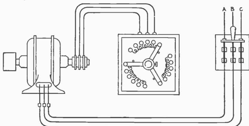
FIG. 2,795.—External resistance or slip ring induction motor connections. The squirrel cage armature winding is not short circuited by copper end rings, but connected in Y grouping and the three free ends connected to three slip rings, leads going from the brushes to three external resistances, arranged as a triplex rheostat having three arms rigidly connected as shown, so that the three resistances may be varied simultaneously and in equal amounts.
