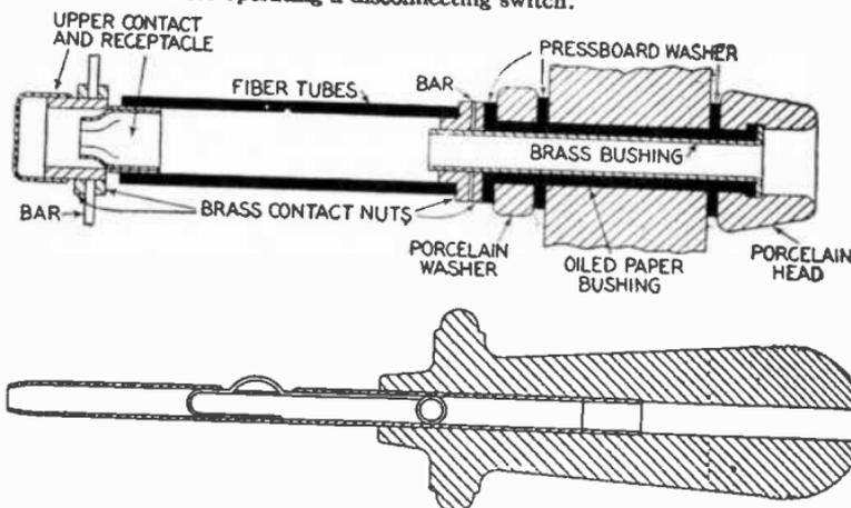
Figs. 4,045 and 4,046.—*Bus transfer plug switch.* The method of supporting the contact farthest from the panel consists of a porcelain pillar of the same height as the receptacle, clamped to a brass connecting or bus bar which in turn is fastened to the receptacle.
