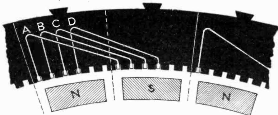
FIG. 3,130.—Diagram of single phase multi-coil or distributed winding to show characteristic differences in construction and action from single coil or concentrated winding.
