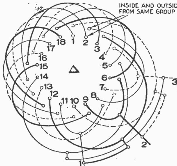
FIG. 3,263.—3 phase, 6 pole, 2 circuit Delta. Connections between coil groups only.
