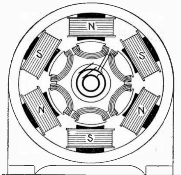
FIG. 3,134.—Diagram of six pole single phase revolving armature alternator, with monotooth or concentrated whole coil winding. For 2,300 volts at 1,200 revolutions per minute, 720 inductors per slot are required. In the case of a concentrated or monotooth winding they may be arranged in "whole coils" as above or in "half coils" (hemitropic) as in fig. 3,135.
