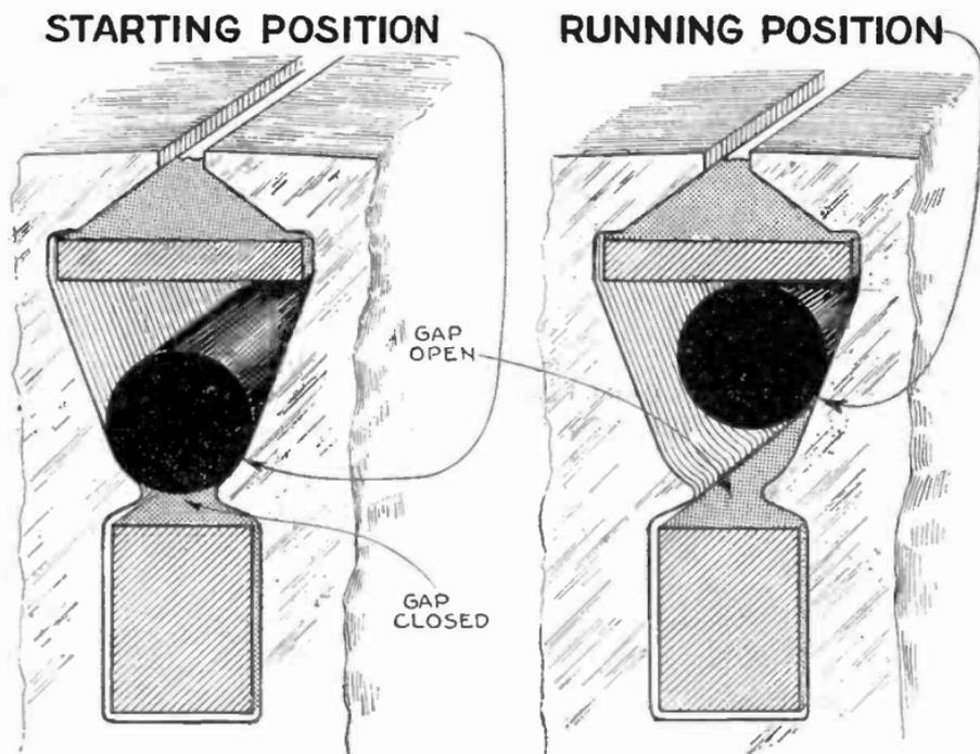
FIGS. 2,771 and 2,772.—Operation of choker rod of Fairbanks Morse choker type double squirrel cage motor. Fig. 2,771, armature at rest, choker rods held in *closed position* by magnetic attraction; fig. 2,772, armature nearly up to running speed, choker rods thrown out by centrifugal force to *open position*, opening the leakage gaps.
