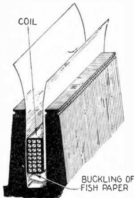
To guard against bending of the straight part of the coil, avoid driving the coil into the slot with the face of the mallet directly.
