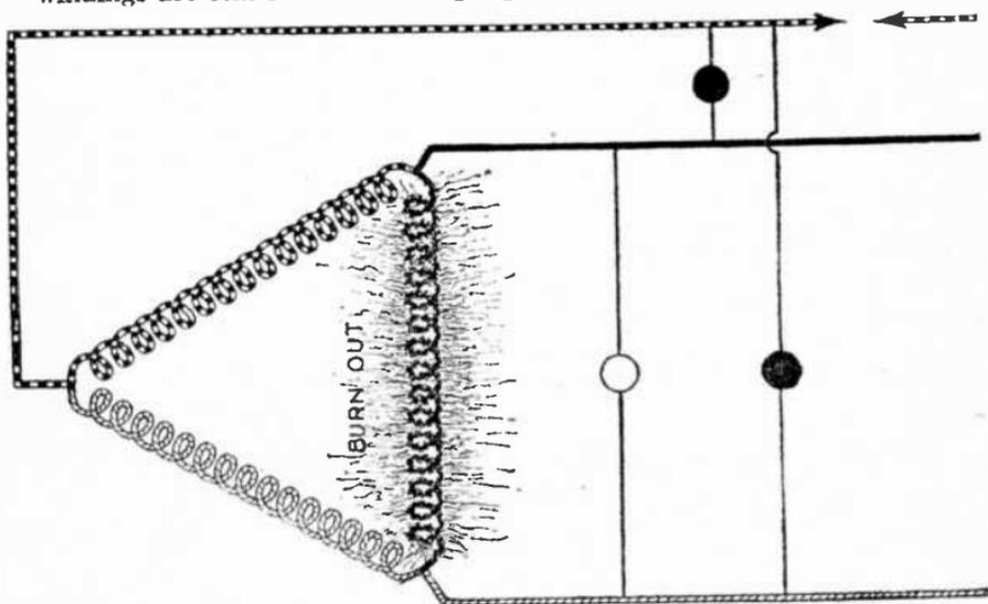
FIG. 3,972.—Single phasing of delta connected motor.
