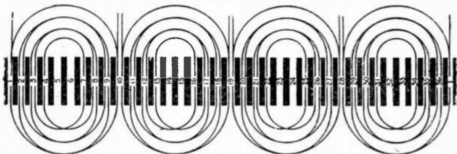
FIG. 3,202.—Diagram of main winding for mould or hand winding.
