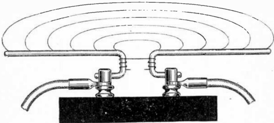
FIG. 4,019.—Flat horizontal horn break fuse.
