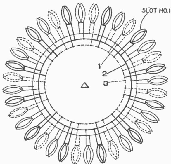
FIG. 3,288.—3 phase, 12 pole, 12 circuit Delta.
