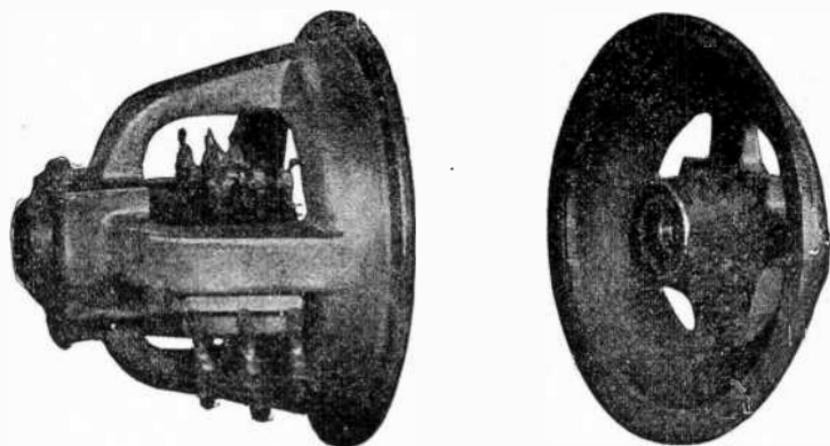
FIGS. 2,803 and 2,804.—*General Electric slip ring motor construction 7.* End shields. Shields interchangeable, end for end. Rabbit fits prevent misplacement. Plenty of heavy cap screws hold shields firmly to field frame. Fig. 2,803, collector ring end shield with brush rigging assembly; fig. 2,804, pulley end shield.
