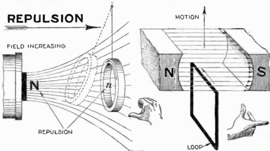
FIG. 2,921.—*Repulsion motor principles 4. A copper ring is repelled from a magnet pole when the number of lines of force passing through the ring is increasing. See fig. 2,919.*
