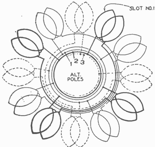
FIG. 3.259.—3 phase, 4 pole, 2 circuit. alternate poles.
