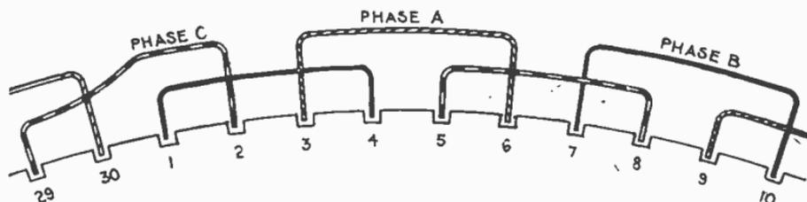
FIG. 3,141.—Three phase, 10 pole, 30 slot winding in two ranges. In this winding perfect symmetry occurs after every four poles. Accordingly in the case of an odd number of pairs of pole, one of the coils must necessarily be askew going from the inner to the outer range as shown at the left.
