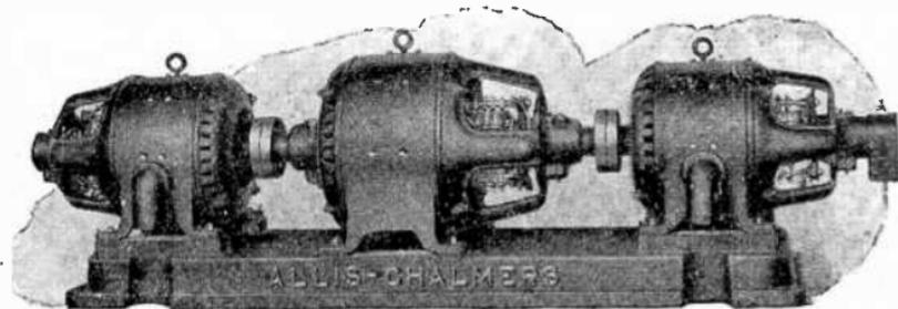
FIG. 3,093.—Allis Chalmers 55 h.p. motor driving two  $17\frac{1}{2}$  k.w., 250 volt, 1200  $r.p.m.$  generators.
