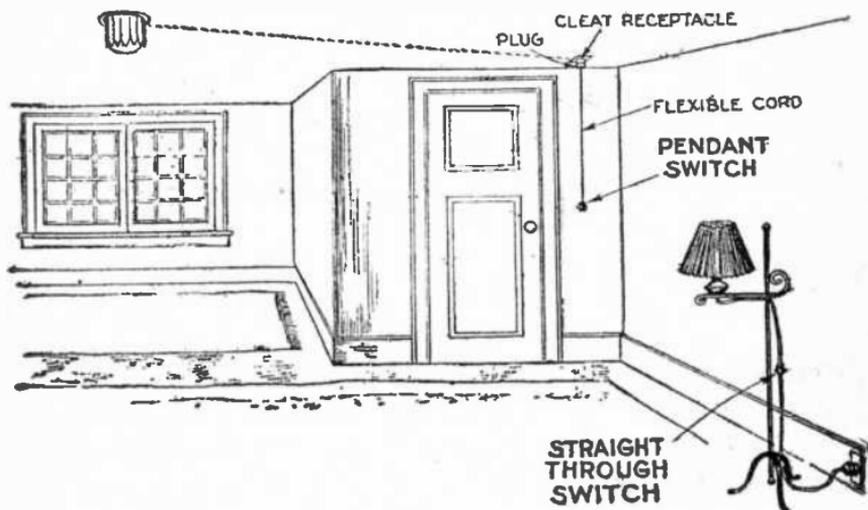
FIG. 4,037.—Interior of room illustrating the installation and use of pendant switch and straight through switch.
