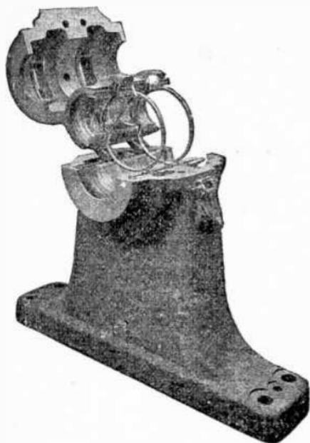
FIG. 3,757.—Westinghouse synchronous converter construction 15. Pedestal bearing. All converters are equipped with bearings which are horizontally split. The lower half of the bearing housing is cast integral with the pedestal.
