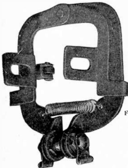
FIG. 2,850.—Century split phase induction motor cut out switch. It is adjusted for a predetermined speed. The governor fig. 2,849 which actuates the cut out is positive in action and opens the starting or phase coil circuit with a rapid break of silver contacts
