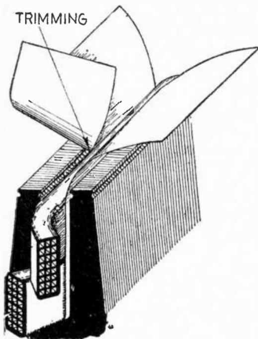
FIG. 3,211.—Slot with coils inserted showing trimming of slot cell.
