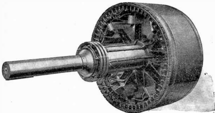
FIG. 2,814.—Allis Chalmers slip ring armature as used on external resistance or slip ring motors. The armature is of the phase wound type having the terminals brought out to three slip rings.
