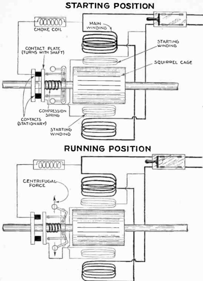
**Figs. 2,846 and 2,847.**—Elementary split phase induction motor *with cut out switch*. Fig. 2,846, cut out switch closed at start; starting winding in circuit; fig. 2,847, motor speeded up to point where centrifugal force acting on governor weights has overcome the tension of spring and opened switch cutting out starting winding.
