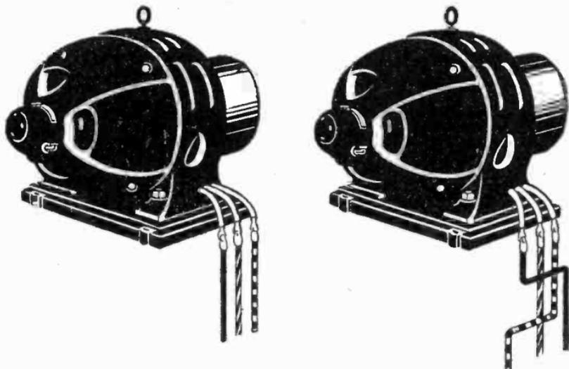
FIGS. 3,932 and 3,933.—Reversing two phase three wire motor; *Interchange the two outside leads.*
