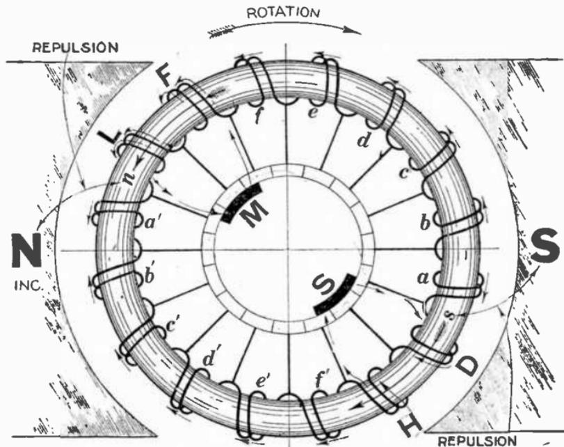
FIG. 2,972.—Ring armature in *a.c.* field with two thick brushes placed to short circuit two pairs of coils L,F, and H,D. *With this arrangement*, clockwise rotation will result due to repulsion by the two pairs of short circuited coils. The resultant effect of the other coils is zero as may be seen from the diagram.
