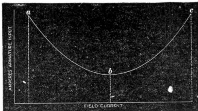
FIG. 3.958.—Curve for synchronous motor showing effect of varying the field current on the armature current required for a given output.
