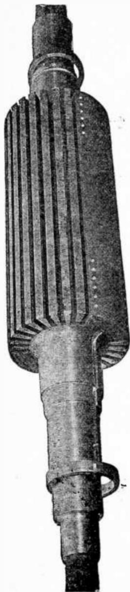
FIG. 3,154.—Westinghouse field core ready for winding. It is made from a solid steel forging and has machined radial slots for the field winding. The slots and field winding are distributed so that the flux distribution of the field poles will be such that the generated voltage wave of the armature winding will be practically free from harmonics of an appreciable magnitude.
