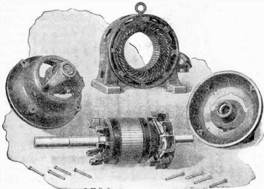
Figs. 2,710 to 2,721.—Wagner internal resistance motor construction 5. Disassembly of motor showing assembled armature, field and end plate.
