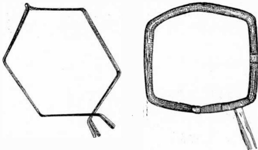
FIGS. 3,144 and 3,145.—Nested, basket, or mush coil and a diamond winding coil showing difference between the two types.
