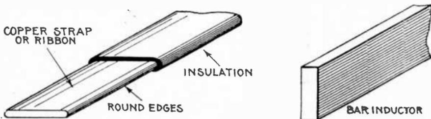
FIG. 3,122.—Copper strap or ribbon with insulation. These are generally from  $\frac{1}{16}$  to  $\frac{1}{8}$  inch thick with rounded edges as shown to avoid cutting the insulation.
