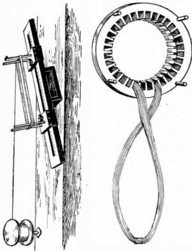
FIG. 3,174.—Adjustable shuttle or skein winder showing operation of winding a skein corresponding to fig. 3,175.
