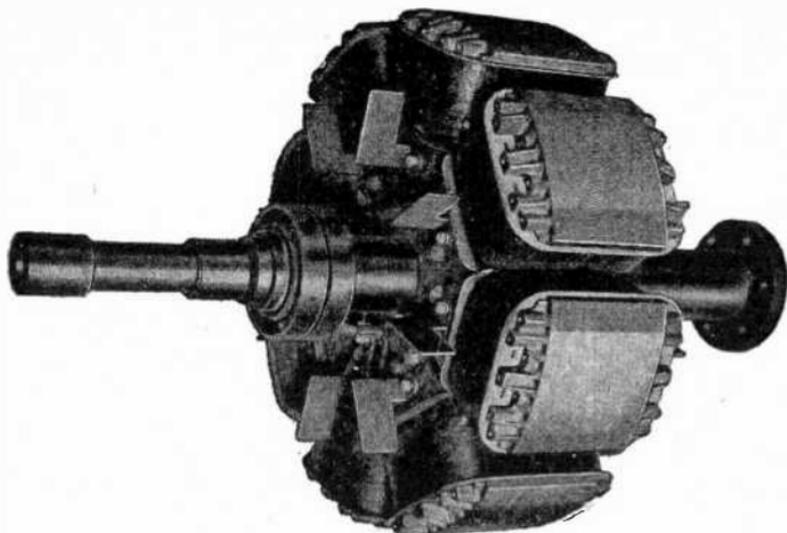
FIG. 3,156.—Westinghouse general turbine alternator field.
