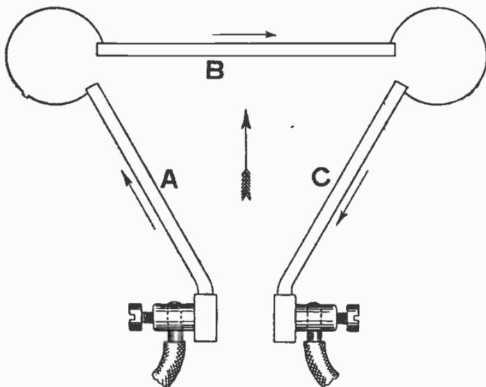
FIG. 4,018.—Experimental circuit, illustrating the action of horn break switches.
