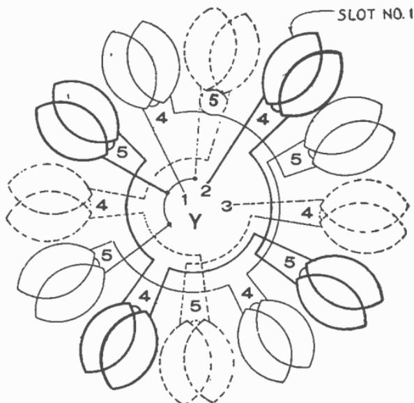
FIG. 3,276.—3 phase, 4 pole, 1 circuit Y, irregular.
