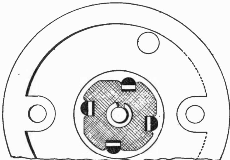
FIG. 4,059.—H & H snap switch method of attaching mechanism to base. *In construction*, metal plates on top and bottom of the porcelain base, riveted together, form the supports for the spindle and act as bearings for it. No matter how the spindle is yanked or wrenched in service these plates hold the spindle and mechanism in alignment.
