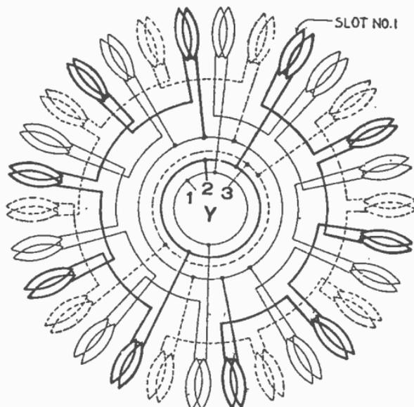
FIG. 3,270.—3 phase, 12 pole, 2 circuit Y, regular.
