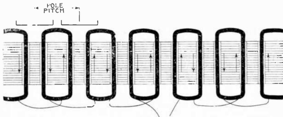
FIG. 3,112.—Developed diagram of single phase concentrated whole coil winding in two slot stamping for six pole alternator. If the sides of adjacent whole coils be slightly separated by placing the winding in a two slot stamping the electrical result will not differ materially from the monotooth whole coil winding.
