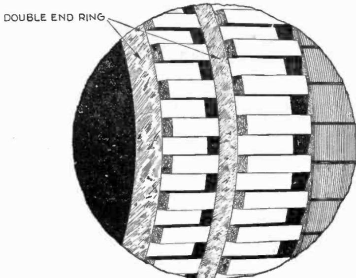
FIG. 2,764.—Westinghouse *double end ring* construction for double squirrel cage armature.
