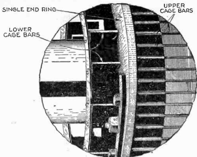
FIG. 2,763.—Westinghouse *single end ring* construction for double squirrel cage armature.
