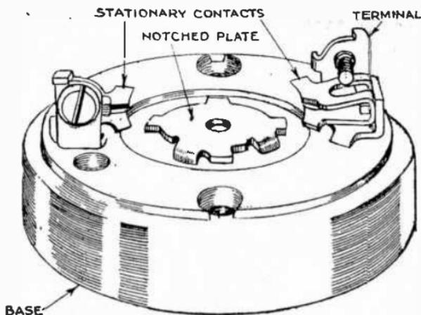
FIG. 4,055.—H & H snap switch porcelain base showing stationary contacts (jaws) terminals and notched plate.
