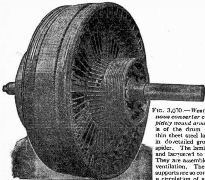
**FIG. 3,070.**—*Westinghouse synchronous converter construction 5. Completely wound armature.* The armature is of the drum wound type having thin sheet steel laminations supported in dovetailed grooves on a cast steel spider. The laminations are annealed and lacquered to reduce the iron loss. They are assembled with air ducts for ventilation. The front and rear coil supports are so constructed as to set up a circulation of air through the front
