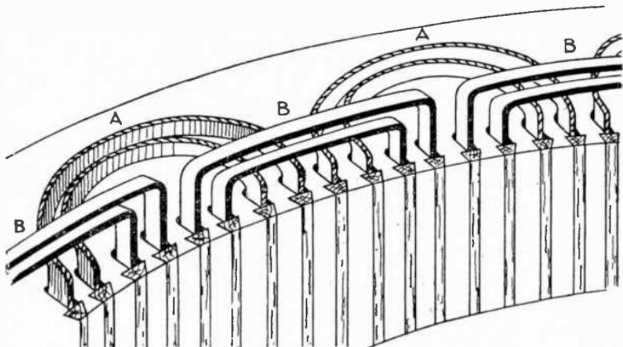
FIG. 3,138.—Treatment of coil ends in two phase, two range concentric chain windings. In this arrangement *straight out B* and *bent up A* coils are used which are placed on the armature as is clearly shown in the illustration.
