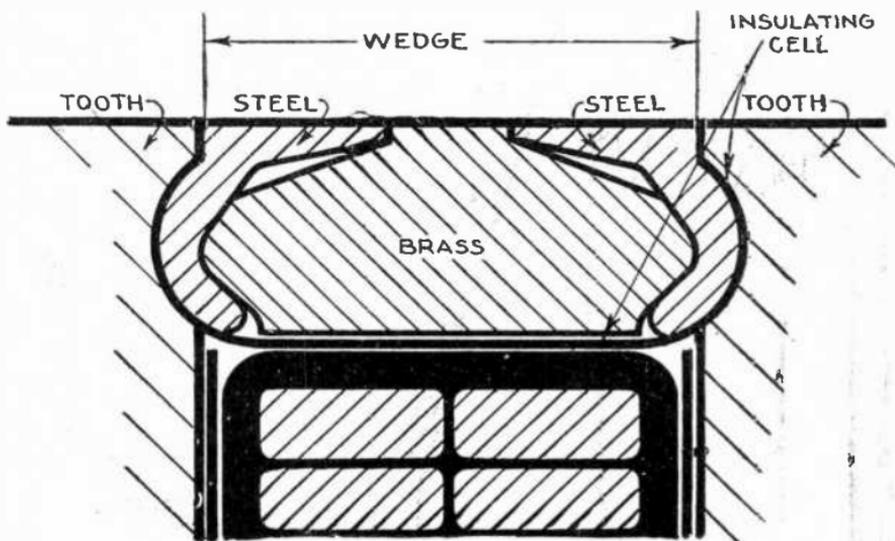
FIG. 3,214.—Cross section through a magnetic wedge.
