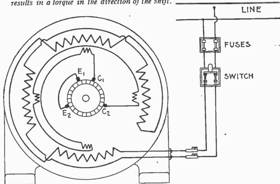
FIG. 2,979—Diagram of connection of Sprague single phase compensated repulsion motor. *To reverse direction of rotation interchange leads C<sub>1</sub> and C<sub>2</sub> and slightly shift the brush holder yoke. Brushes E<sub>1</sub> and E<sub>2</sub> are permanently short circuited. This diagram of connections applies also to fig. 2,981.*
