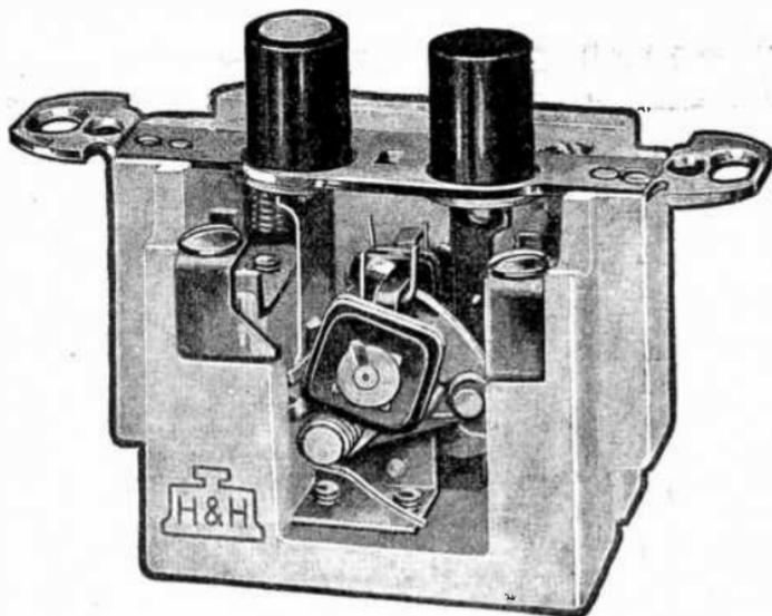
FIG. 4,031.—Hart and Hegeman momentary contact switch. Pressure on the button closes the circuit as long as the button is held in. Releasing the button opens the circuit. Quick make and break. The two circuit type has two separate single pole switches, each controlling a separate circuit. Both buttons cannot be operated at the same time.
