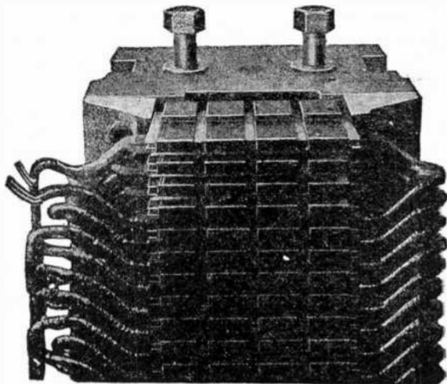
FIG. 3,942.—Detail of joint showing split stator construction of Ideal 600 h.p., 2,200 volt, 3 phase, 25 cycle, synchronous motor.
