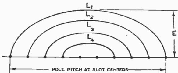
FIG. 3,179.—Diagram illustrating method of determining length of loops.
