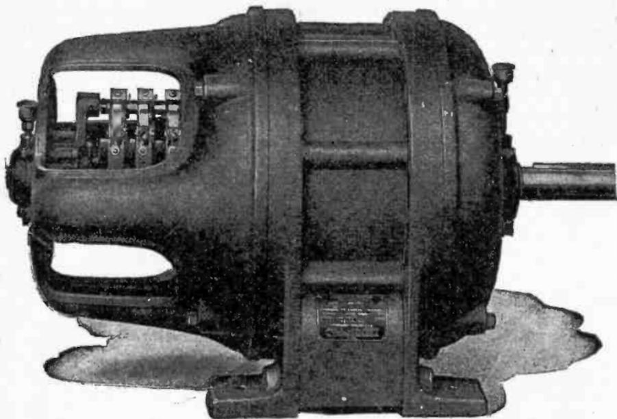
FIG. 2,805.—Allis Chalmers type ARY external resistance or slip ring motor. This type motor is adapted to keep the starting current within limits, or where a large starting torque is required, the slip ring or wound rotor type is used. This type requires a smaller current to develop a given starting torque, and is therefore used where frequent starting is necessary.
