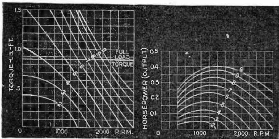
torque curves of a  $\frac{1}{4}$ -h.p. motor with the brushes set a distance corresponding to 2,3,4 etc. bars from neutral, as indicated by the numerals. However, it should be understood that the brush positions are not limited to these settings. Fig 3,013 gives speed output curves at the same brush settings. By the aid of these curves the load on the motor can be found. While these curves are accurate only for one rating, they indicate the general characteristics of all type L.K. motors.
