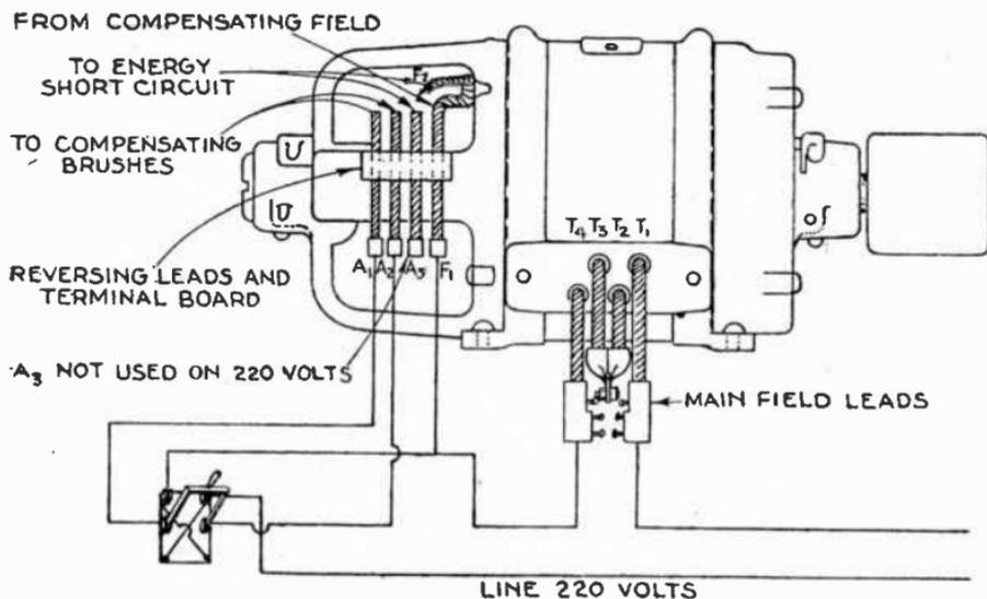
FIG. 3,970.—General Electric type R1 motor connected for 220 reversing operation, with double pole, double throw switch.
