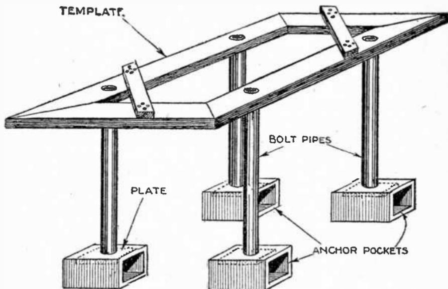
FIG. 3,936.—View showing template for locating anchor bolt centers, pipes through which the bolts pass, and bolt boxes at lower end of bolts. The completed foundation is shown in fig. 3,937, with template removed. The template is made of plain boards upon which the center lines are drawn, and bolt center located. Holes are bored at the bolt centers to permit insertion of the pipes as shown.
