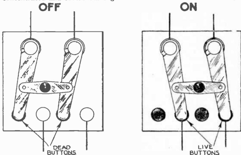
Figs. 3,991 and 3,992.—Double pole lever switch showing essentials and operation. Fig. 3,991, off position; fig. 3,992, on position.
