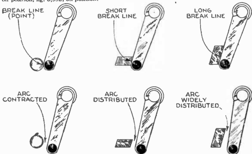
Figs. 3,993 to 3,998.—Various break forms and results obtained as explained in the text. The illustrations show blade and different shaped contacts of lever switches.
