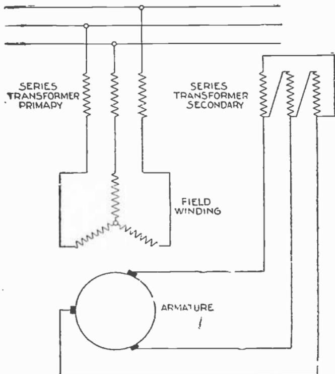
FIG. 3,010.—Connections of a three phase brush shifting series motor. A series transformer is generally used to step down the voltage for the armature as low voltage is necessary to good commutation. The secondary of this transformer is connected for three phases and the armature has three sets of brushes per pole pair. The transformer, by its ability to become saturated, limits the no load speed of the motor to a safe value, which is usually about 150 per cent normal.
