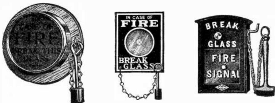
Figs. 8,517 to 8,519.—Partrick & Wilkins break glass fire alarm signal boxes or open circuit, with vibrating bells. Fig. 8,517, No. 1 signal, breaking of glass automatically closed circuit. For low voltage only; fig. 8,518, flush type for low voltage; fig. 8,519, type for 110 volts or less.
