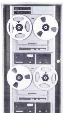
The system provides for automatic transfer to second deck at the end of the reel, or in the case of a tape break or time recording malfunction. Models include 1 channel 4 pass for up to 153.6 hours unattended at 5/16 ips; 2 channel 2 pass
