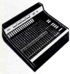
The BC-5 includes a five-year warranty, four outputs with individual VU's and monitors, Cue, foldback and equalizers, flexible-up to 16 low-level inputs or 28 high level inputs, echo send on all inputs, and echo return on all masters.
