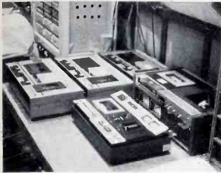
Audio cassette decks were used to play sample portions of nominations for 'Song of the Year.' Due to wow & flutter and hiss inherent in cassettes, 7 1/2 ips, 1/4" cartridges may be used next year.
