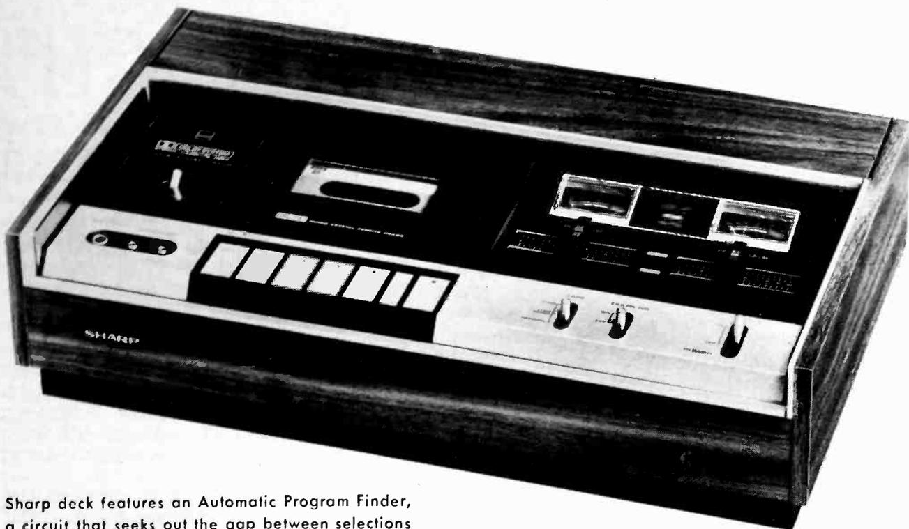
Sharp deck features an Automatic Program Finder, a circuit that seeks out the gap between selections on a cassette.
