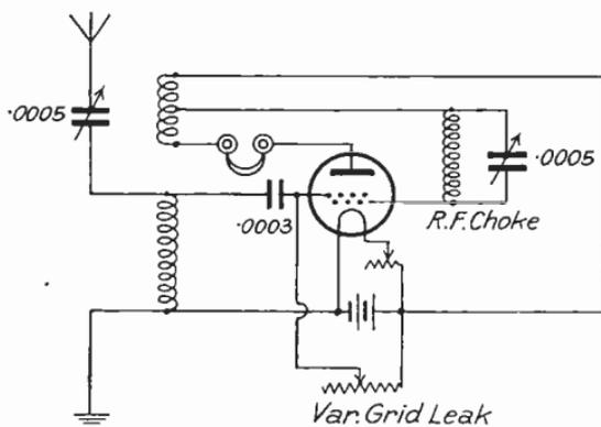
FIG. 1.—THE UNIDYNE CIRCUIT FOR H.T.—LESS RECEPTION
