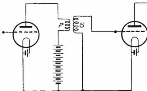
FIG. 2.—TRANSFORMER COUPLING
