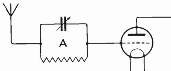
FIG. 4. LODGE "N" CIRCUIT. THEORETICAL DIAGRAM
