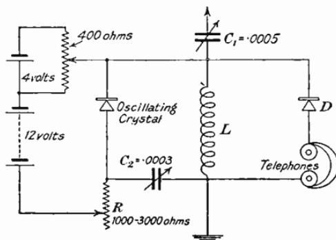
FIG. 7. A PRACTICAL OSCILLATING CRYSTAL CIRCUIT
