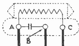
FIG. 29. CONNECTIONS OF THE T.C.C. SERIES—PARALLEL CONDENSER
