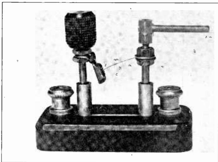
FIG. 2. THE "MILLER" CRYSTAL OSCILLATOR. (PAT. 17767)
