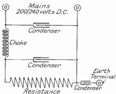
FIG. 4. RADIAC HIGH-TENSION MAINS UNIT
