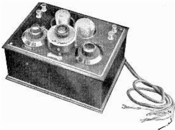
FIG. 33. THE B.T.-H. TWO-VALVE L.F. SET
