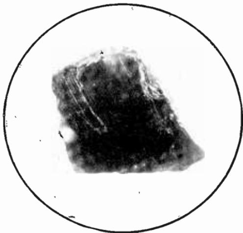
FIG. 1. A ZINCITE CRYSTAL POSSESSING GOOD OSCILLATING PROPERTIES
