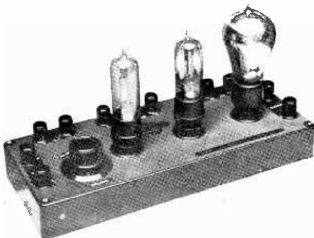
FIG. 34. IGRANIC 3-VALVE RESISTANCE CAPACITY AMPLIFIER
