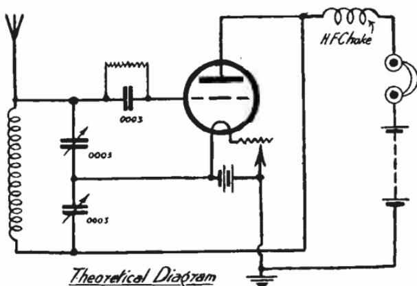
FIG. 5. COLPITTS ONE-VALVE CIRCUIT
