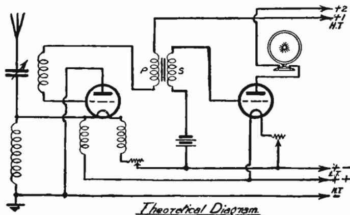
FIG. 3. FILADYNE TWO-VALVE CIRCUIT
