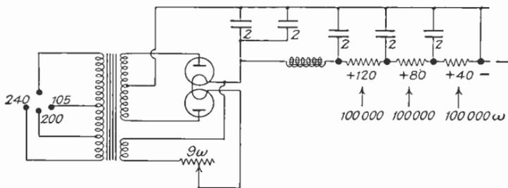
FIG. 3. INTERNAL WIRING OF THE ELVEN MAINS HIGH-TENSION UNIT
