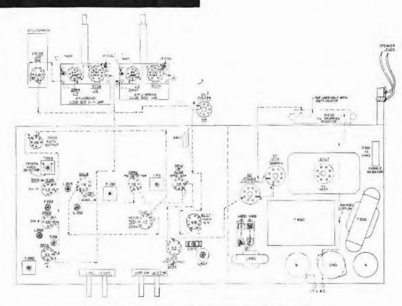
Tube location, heater string, and adjustments. Top view of chassis.
