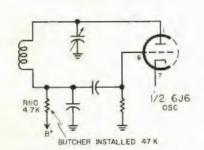
Fig. 2—Oscillator failed on high end due to low plate voltage.
