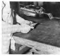
A king-size magnifying glass mounted on the workbench with a swivel arm makes easy, the minute examination of small parts.
