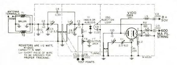
Schematic Diagram for UHF Tuner, RUX-023
