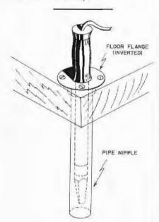
Store a hot soldering iron safely out of the way, but handy for use, by dropping it into a pipe nipple set in the workbench. Fit the neck of a floor flange in a hole in the bench; mount the flange upside down, then, from beneath the bench, turn a pipe nipple into the threaded flange.
