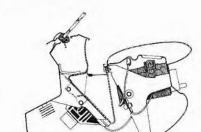
SECTION THRU INSTRUMENT PANEL SHOWING SPEAKER INSTALLED
