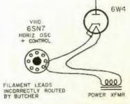
Fig. 1—The damper filament leads upset oscillator sync.
