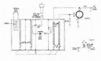
472V024H04 UHF tuner schematic diagram.
