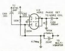
Fig. 1—Partial schematic of the horizontal afc system used in the Sportan 15V215 TV set.
