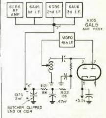
Fig. 3—Partial schematic of the RCA KCS-48 agc circuit.
