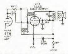
Fig. 2—Audio output stage of the GE ST line. Defect in R308 or R309 could couse distortion.
