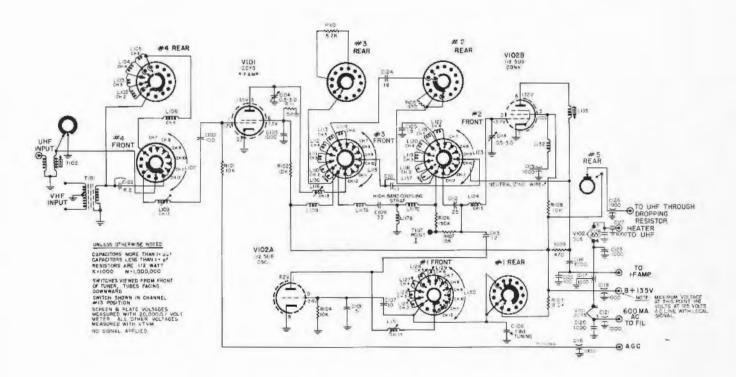
Schematic Diagram VHF Tuner RJX-100
