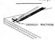
Cutting out a rivet is easier, especially if it's in close quarters, by first using the chisel to crosscut the head. Each quarter of the rivet can then be knocked off with less effort, and less danger of flying fragments. Very handy on chassis work.
