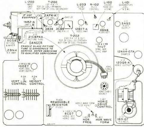
Chassis Tube Layout and Trimmers
