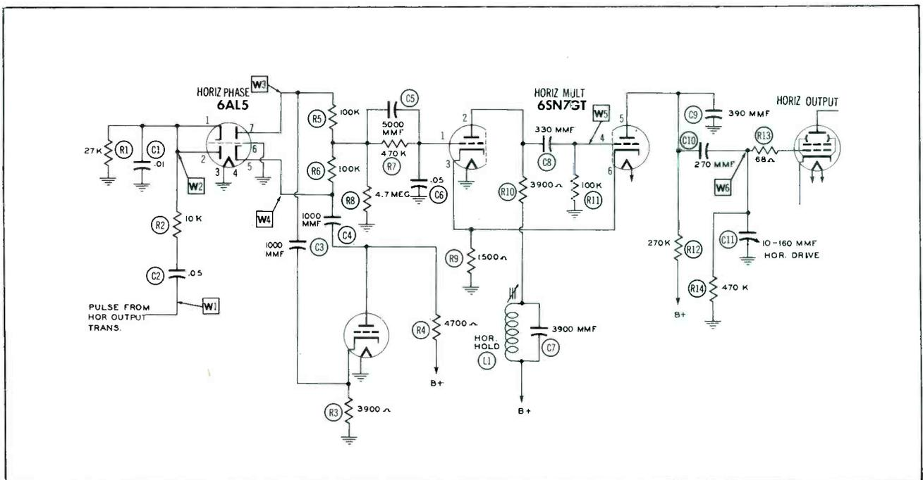
Figure 4. Schematic of Typical Horizontal AFC System Using Phase Detector and Multivibrator.
