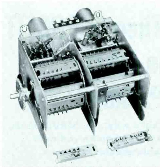
Figure 7. Turret Drum of Zenith Tuner With a Pair of Strips Removed.
