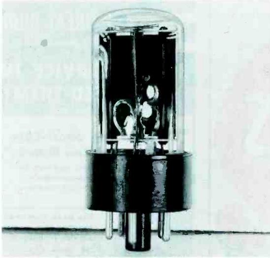
Figure 3. A Photo of a Rectifier Tube Damaged as the Result of Warped Plates.
