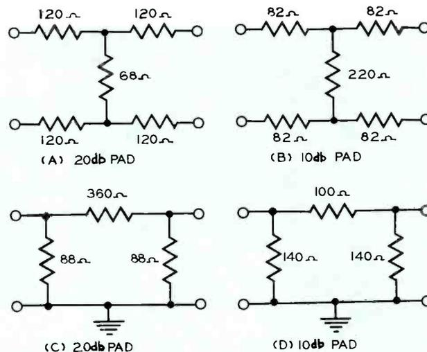
Figure 4. 10 and 20 db Pads for 300 Ohm Balanced Lines (A and B) and 72 Ohm Unbalanced Lines (C and D). COURTESY RCA and DuMONT.
