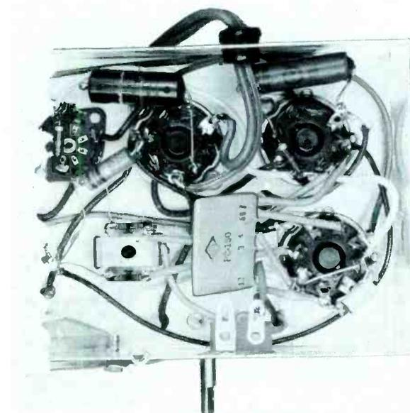
Figure 7. Coupling Circuit Wired Into Small Radio.
