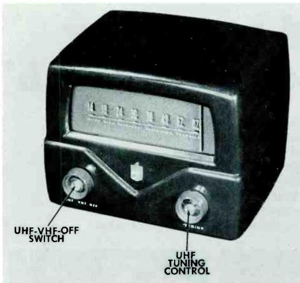
Figure 6. Mallory UHF Converter Model TV-101.
