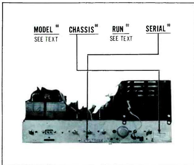
**MODEL NUMBER:** No definite pattern is used in assigning model numbers, other than the fact that the first two digits signify in what year the set was manufactured. This number is found on a sticker placed on the back of the safety cover of the cabinet.
