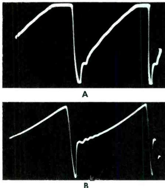
Figure 2. Waveforms Typical of Those Found on the Control Grids of Horizontal Sweep Amplifiers.
