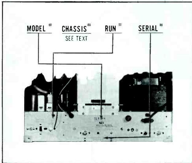
the left side of the rear chassis apron is used as a reference as to the time various production changes have been instituted. A typical number is "51-16-3" where the "51" stands for the year of manufacture, the "16" for the week and the "3" for the day of the working week.
