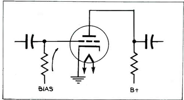
Figure 2. Direction of Grid Current Flow When the Grid Emits Electrons.
