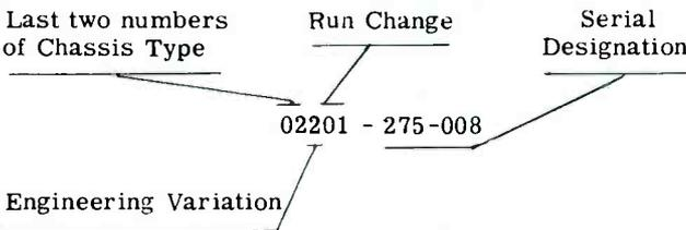
In the example above the serial number represents a 1-502-2 chassis incorporating run change C 01. The engineering variation number identifies major variations, such as a different tuner unit or picture tube, from chassis of the same general type.
