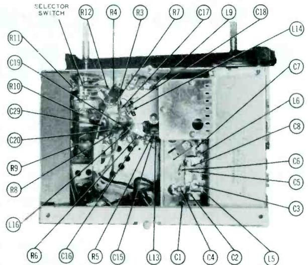
Figure 8. Bottom Chassis View of Mallory UHF Converter. Early Version. (Before Serial #200,000).
