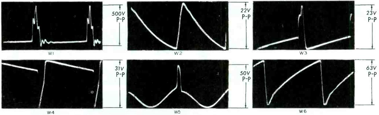
Figure 5. Waveforms Observed in Phase Detector and Multivibrator Circuits of Figure 4. Peak-To-Peak Voltages are Indicated as They Were Found on the Particular Receiver Upon Which These Tests Were Taken. Considerable Variation Will be Found With Different Receivers. (Oscilloscope Sweep Rate is 7875 cps.)
