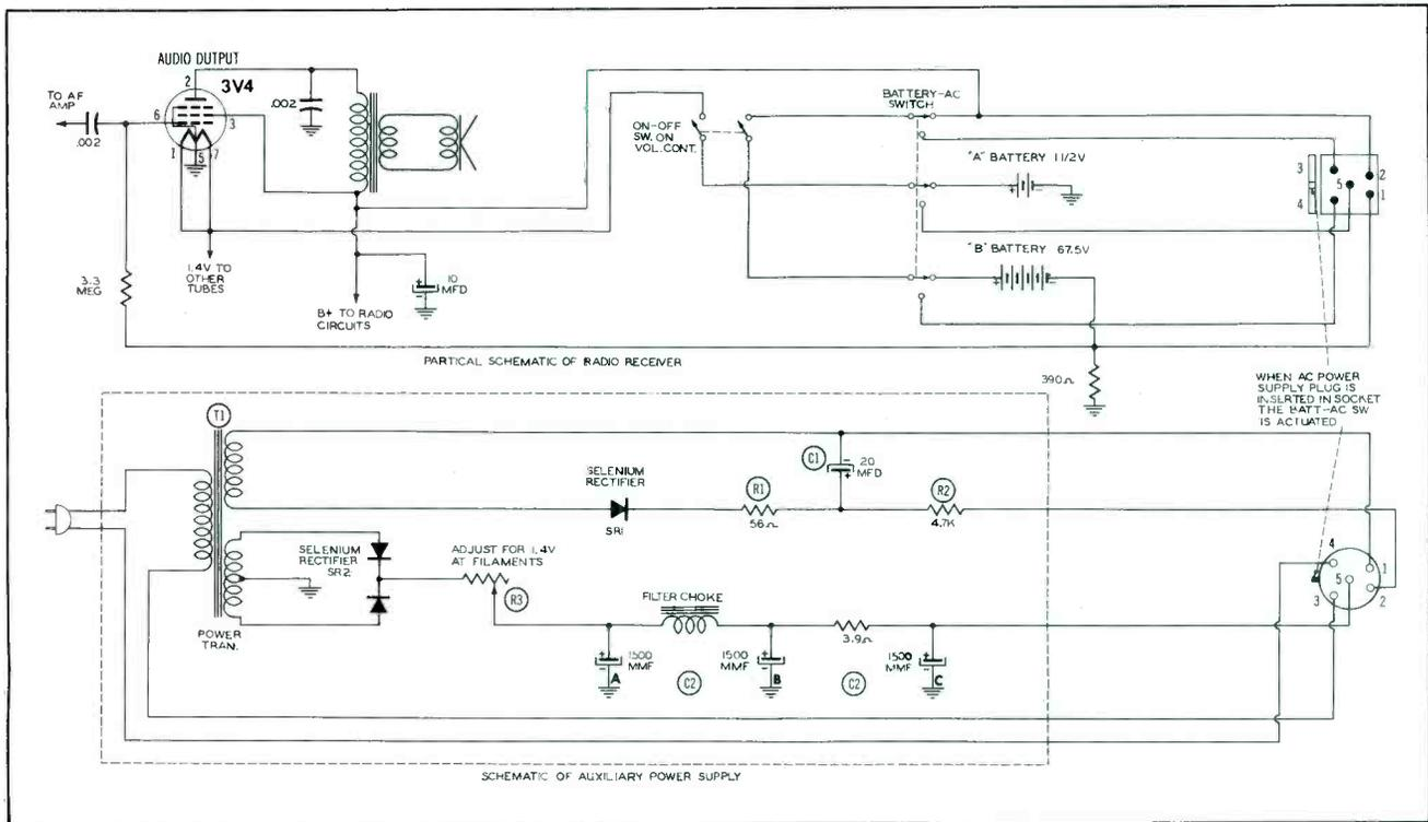
Figure 4. Schematic of Westinghouse Model H-377 Auxiliary Power Supply.
