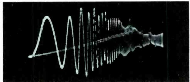
Figure 6. Output of Crystal Cartridge.
