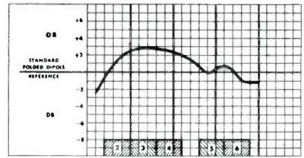
Gain of Amphenoil Model No. 114-005 Antenna over a reference folded dipole, 54 to 88 mc.
