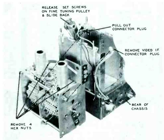
Figure 6. Zenith Tuner Removed From Chassis.
