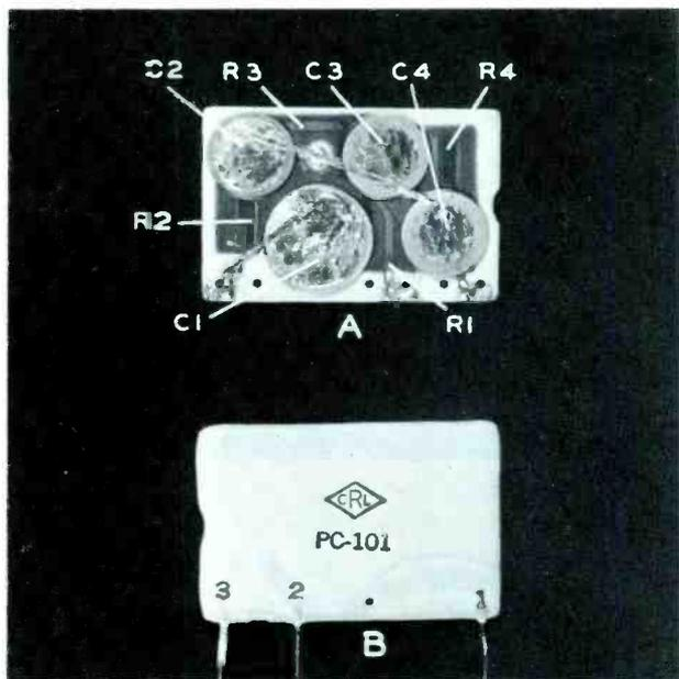
Figure 12. Construction Details of an Integrator Plate Employing Separate Capacitors.
