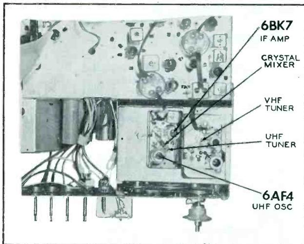
Figure 1. VHF and UHF Tuning Units Employed in Arvin TV Receivers.
