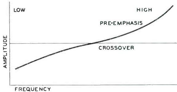
Figure 2. Recording Curve.
