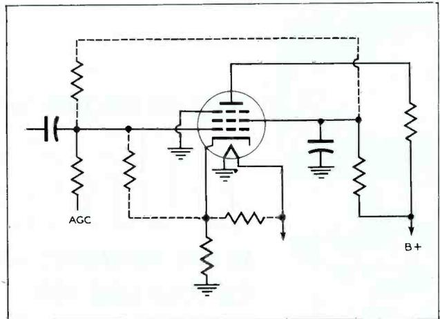
Figure 5. Leakage Paths Which May Exist in a Tube or Tube Socket.
