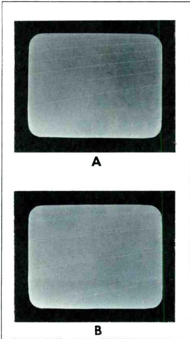
Figure 2. Visible Vertical Retrace Lines Illustrating (A) Good Interlace and (B) Poor Interlace.
