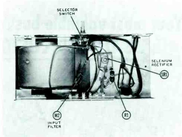
Figure 16. Bottom Chassis View of Regency Converter.
