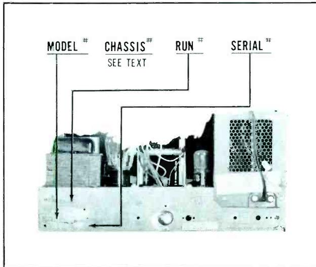
**MODEL NUMBER:** The model number is ink-stamped on the left end of the rear chassis apron and printed on a combination name label and tube layout chart which is affixed to an inner wall of the cabinet.
