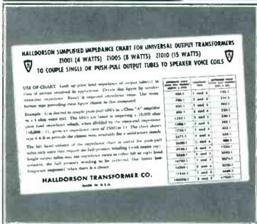
This impedance chart, for example, is a marvel of condensation and simplification. When installing a universal output, I don't have to wade through a lot of useless figures to get the right coupling data. This short-cut saves my time and my temper.
