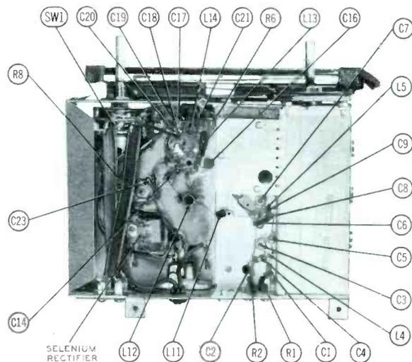
Figure 12. Bottom Chassis View of Mallory Converter, Late Version.
