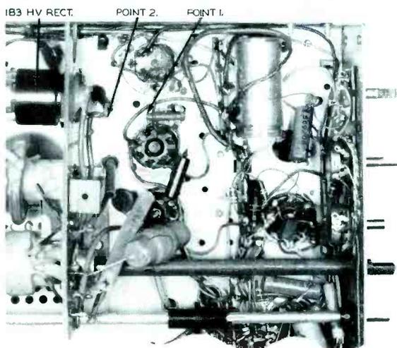
Figure 5. Under-Chassis View of a Corona Problem.
