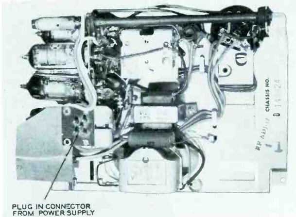
Figure 2. Chassis of Westinghouse Model H-373P4.
