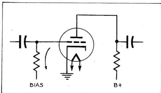
Figure 1. Direction of Grid Current Flow in a Normal Operating Tube When the Grid is Driven Positive by Signal Components.
