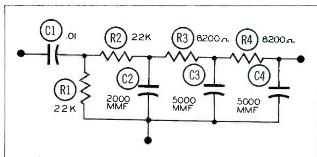
Figure 13. Schematic of Unit Shown in Figure 12.
