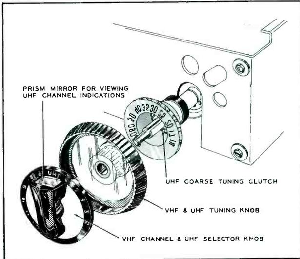
Figure 4. Control Knobs with Prism Mirror For Viewing UHF Channel Markings.
