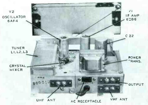
Figure 11. Top Chassis View of Mallory Converter, Late Version. (Serial #200,000 and up.)
