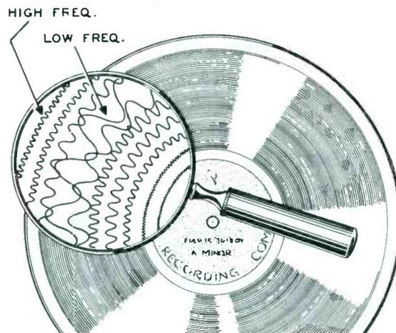
Figure 1. Over-Modulation of Grooves at Low Frequencies.
