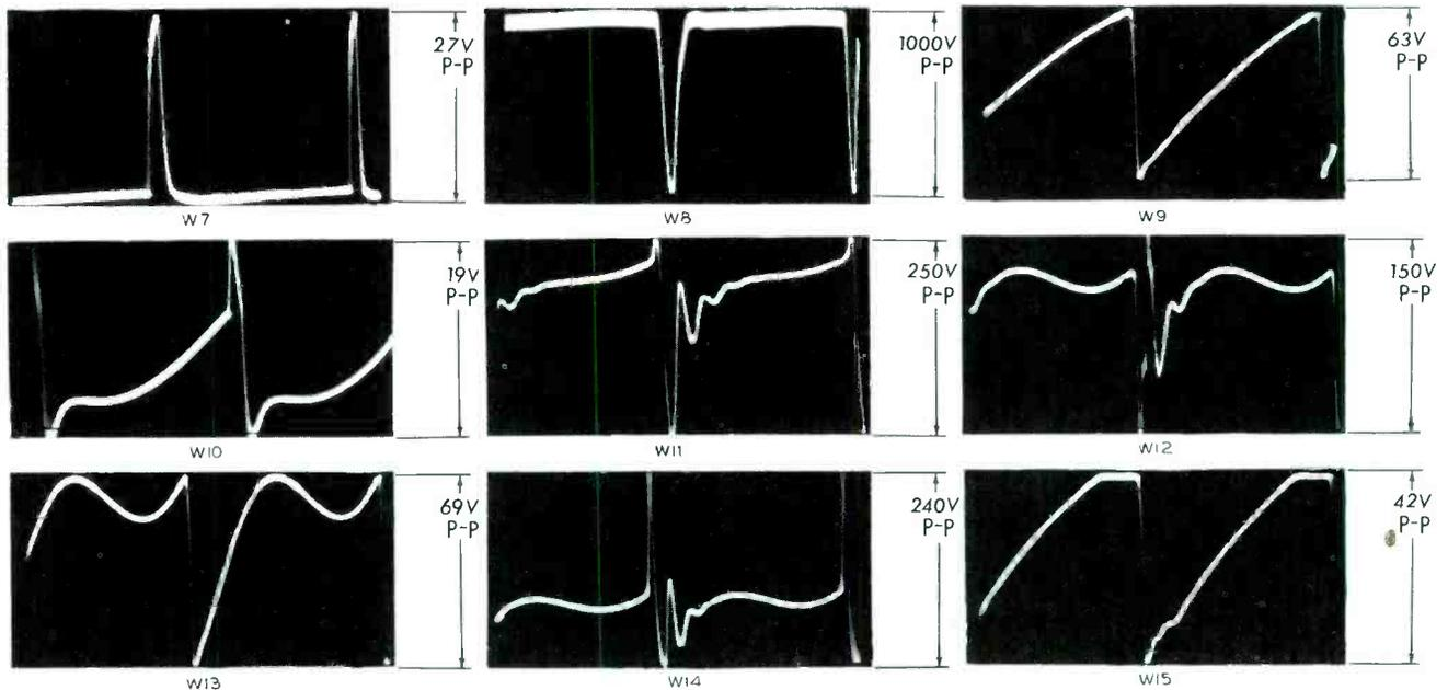
Figure 7. Waveforms Observed in Synchroguide\* Circuit of Figure 6. Peak-To-Peak Voltages are Indicated as They Were Found on the Particular Receiver Upon Which These Tests Were Taken. Considerable Variation Will be Found With Different Receivers. (Oscilloscope Sweep Rate is 7875 cps.)
