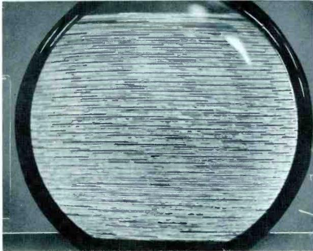
Figure 3. Photograph of CR Tube Image With Horizontal Oscillator Operating at Random Frequencies.
