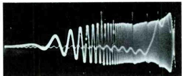
Figure 7. Output of Variable Reluctance Cartridge.
