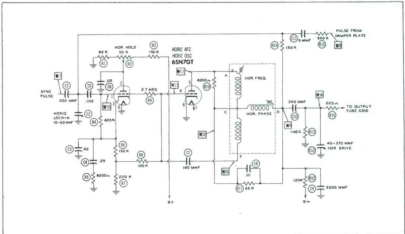
Figure 6. Schematic of Typical Horizontal or AFC System Using Synchroguide\* or Pulse-Width Circuit.
