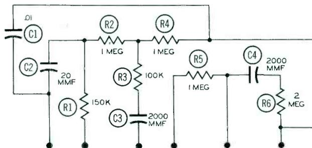
Figure 14. Schematic of Special Audio Compensating Printed Circuit.
