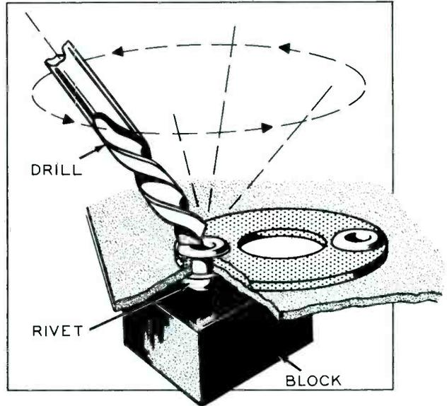
Figure 3. Removing a Rivet by Drilling.
