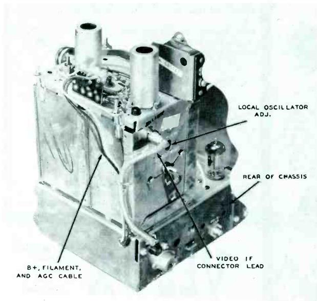
Figure 5. The Zenith Turret Tuner Employed on Chassis 21K20.
