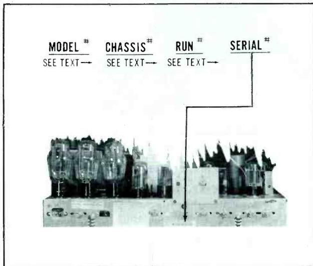
**MODEL NUMBER:** The model number denotes the series and identifies the type of cabinet used. The number is found on the tube layout chart on the inside wall of the cabinet.
