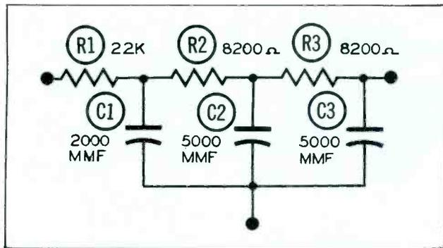
Figure 8. Typical Integrator Network.
