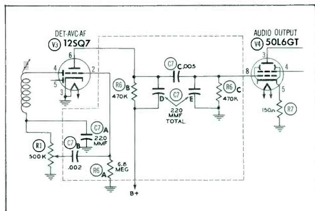
Figure 6. Partial Schematic Showing Incorporation of Printed Coupling Circuit.
