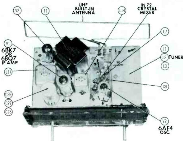
Figure 7. Top Chassis View of Mallory Converter. Early Version. (Before Serial #200,000).
