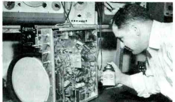
Because of its high dielectric strength, Krylon helps prevent corona. Here technician Bernard Vanella—on the staff of dealer Mort Farr, Philadelphia—"Krylon-izes" high voltage coil and insulation, the socket of the high voltage rectifier, component parts of the rectifier circuit.
