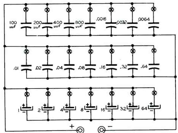
Figure 2. A Suitable Capacitor Substitution Box.
