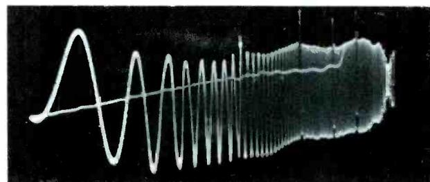
Figure 11. Output of Variable Reluctance Cartridge Through Preamplifier and Control Unit (33-1/3 NARTB).
