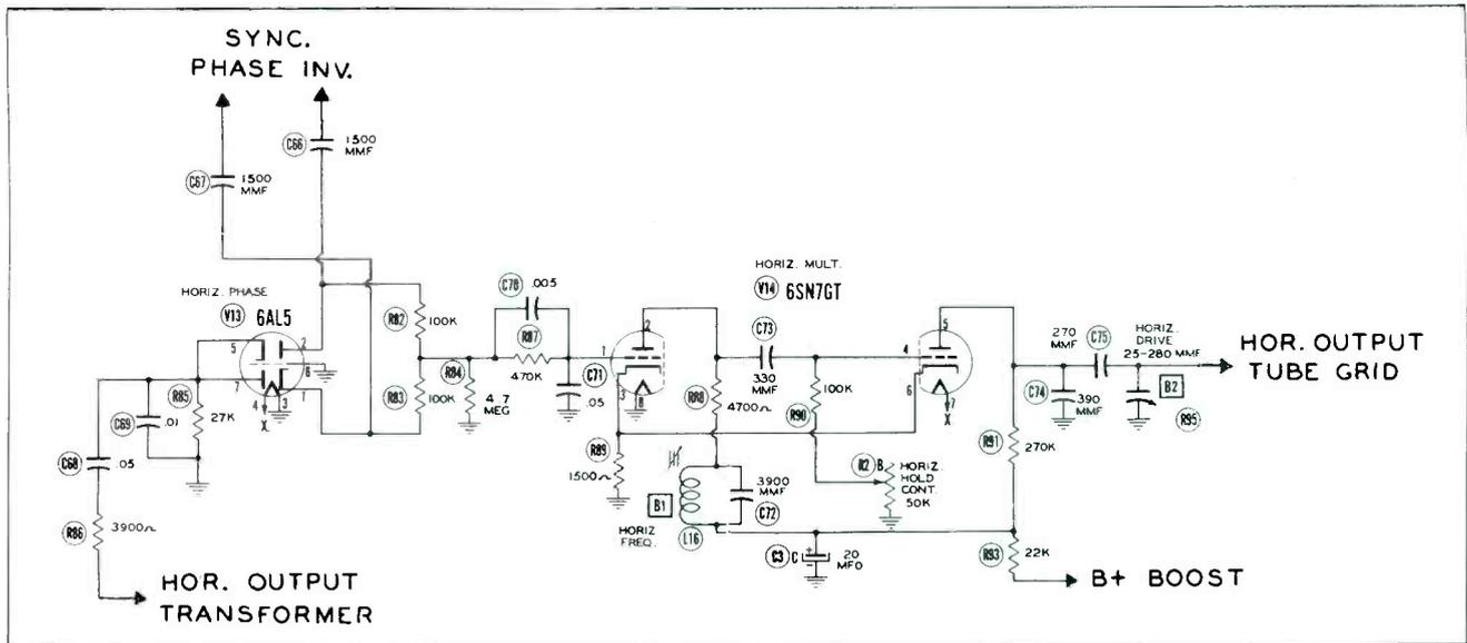
Figure 4. Typical Phase Detector and Multivibrator Horizontal AFC System.
