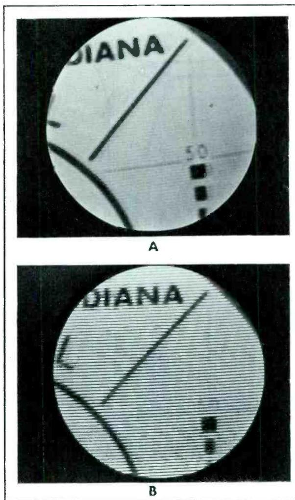
Figure 1. Expanded Partial Photograph of a Test Pattern Illustrating (A) Good Interlace and (B) Poor Interlace.
