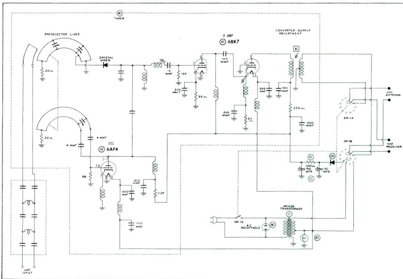
Figure 17. Schematic of Regency Converter.
