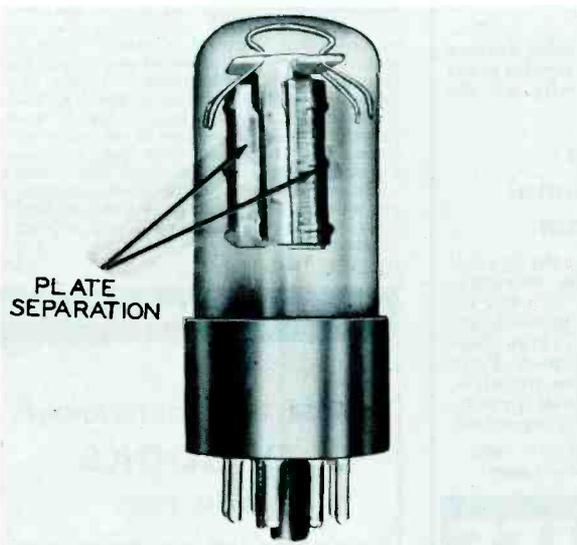
Figure 4. A 6V6GT Tube Defective Because of Broken Welded Bond Due to Excessive Heat Dissipation.
