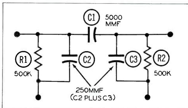
Figure 4. Schematic of Coupling Circuit Shown in Figure 3.
