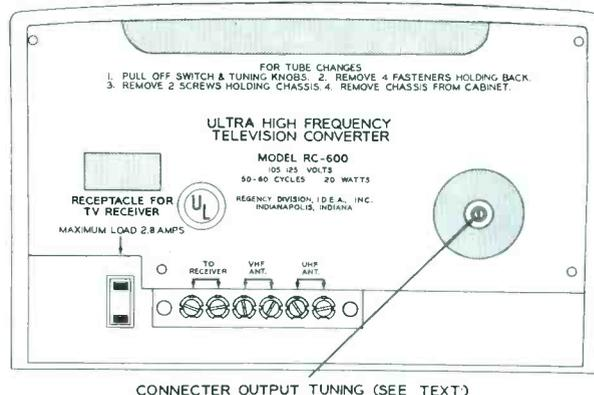
Figure 14. Back of Converter Unit Showing Terminal Strips Power Receptacle and Output Tuning Adjustment.
