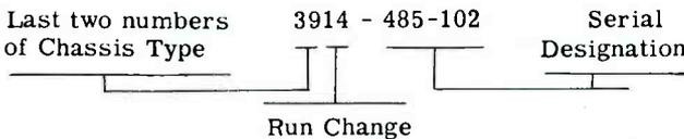
In the example above the serial number represents a 1-139 chassis incorporating all changes through 14.
