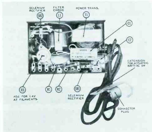
Figure 3. Westinghouse Model H-377 Auxiliary Power Supply (Cover Removed).
