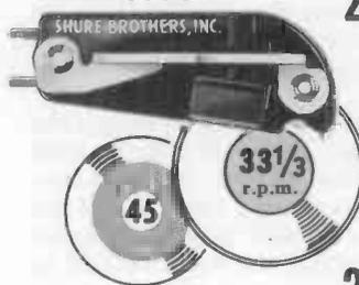
2. This high output (2.1 volts!) "Direct Drive" cartridge was specifically designed for use with all fine-groove records. Universal mounting bracket provides quick, easy installation in RCA-type 45 r.p.m. changers. (Fits 1/2" and 3/8" mounting centers.) Has easy-to-replace needle. For maximum quality, highest output, and low cost, specify Model W31AR at the low list price of only \$6.50.
