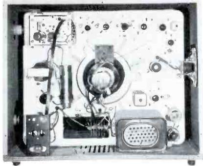
**Fig. 1. Muntz Chassis 47A4 Mounted in Cabinet.**
