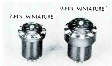
Fig. 12. Test Adapters for Tube Sockets.
