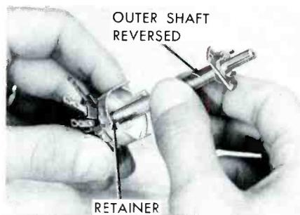
**Fig. 6D. The Outer Shaft Is Used to Seat the Retainer.**
