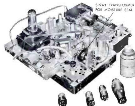
Fig. 2. High-Voltage Area Ready to Be Sprayed With Acrylic Plastic.
