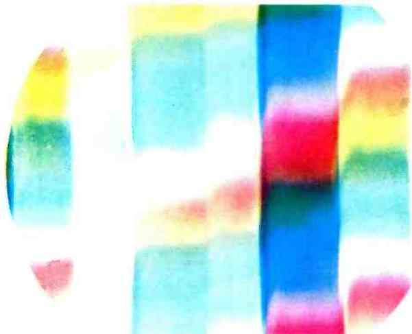
Fig. E1. Color-Bar Pattern Indicating Loss of Color Synchronization.
