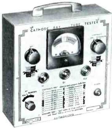
Fig. 3. Authorized Model 101F Cathode-Ray Tube Tester and Rejuvenator.
