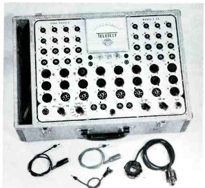
Fig. 4. Another Tube Checker for Rapid Testing.
