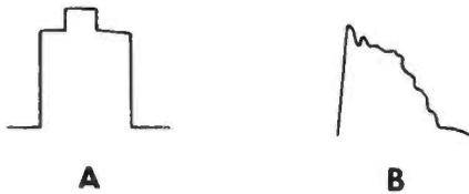
**Fig. 11. Horizontal Blanking Pedestal and Sync Pulse. (A) Normal; (B) Distorted Because of Poor Low-Frequency Response.**
