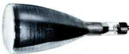
**Fig. 2. Modern 5-Inch Cathode-Ray Tube.**
