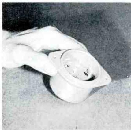
Fig. 1. Tube Socket for High-Voltage Rectifier Employed in Zenith Model X222OR Television Receiver.
