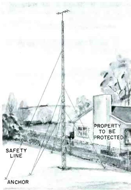
Fig. 2. When Antenna Mast Is Potential Hazard to Adjacent Property, Safety Line Must Be Secured to Mast on Side Away From Endangered Property.
