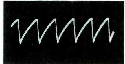
(A) Unmodulated waveform.
