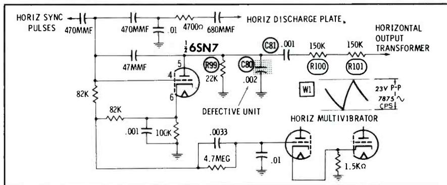
Fig. 2. Triode phase detector for horizontal AFC.
