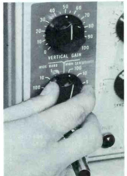
Fig. 1. Wide-Band—High-Sensitivity switch on an oscilloscope.
