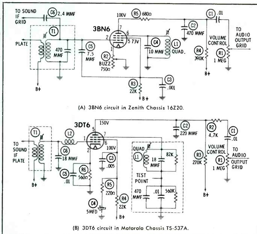
Fig. 2. Schematic diagrams of quadrature-grid detectors.
