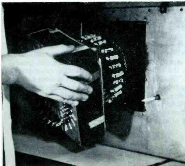
High temperature test ovens are used to check insulation resistance of Sangamo high reliability capacitors under sustained temperatures of 125° C.
