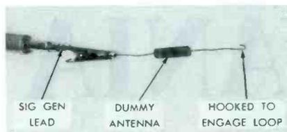
Fig. 2. Hooked lead on dummy antenna.
