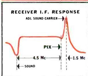
In case shown Receiver AGC is held down by a strong adjacent channel sound carrier. This lowers receiver gain and prevents proper reception of the desired channel. "Beat" or "Herringbone" pattern is predominant on the screen.
