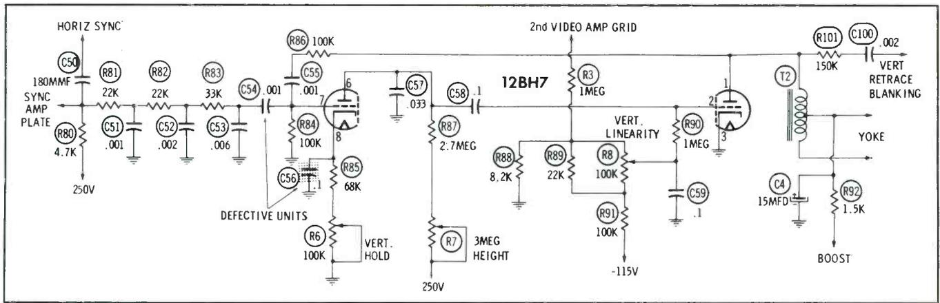
Fig. 3. RC-coupled vertical multivibrator.
