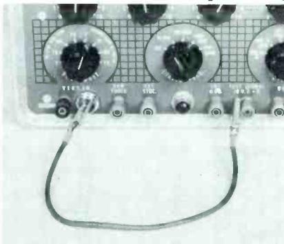
Fig. 3. Calibrating voltage applied to vertical input from test-signal jack.
