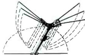
Telrex Labs., Asbury Park, N.J., has introduced the "Quickie," a conical V-beam antenna designed to be low-priced, durable, and easy to install. The antenna is of all-aluminum construction
