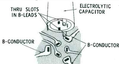
Fig. 4. Metal body of electrolytic filter capacitor used in B— circuit.
