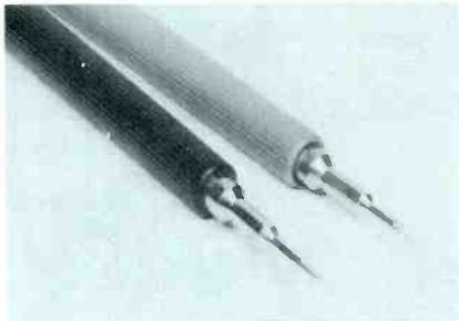
Fig. 3. Needle-pointed test leads.
