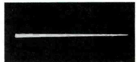
Fig. 7. Oscilloscope trace which exhibits the effect of astigmatism.
