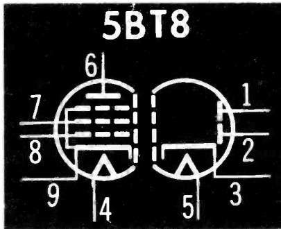
Fig. 7. Basing diagram of 5BT8.
