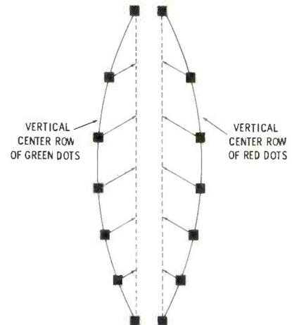
Fig. 4. Appearance of red and green rows when amplitude and tilt controls have been adjusted for maximum displacement at screen center.
