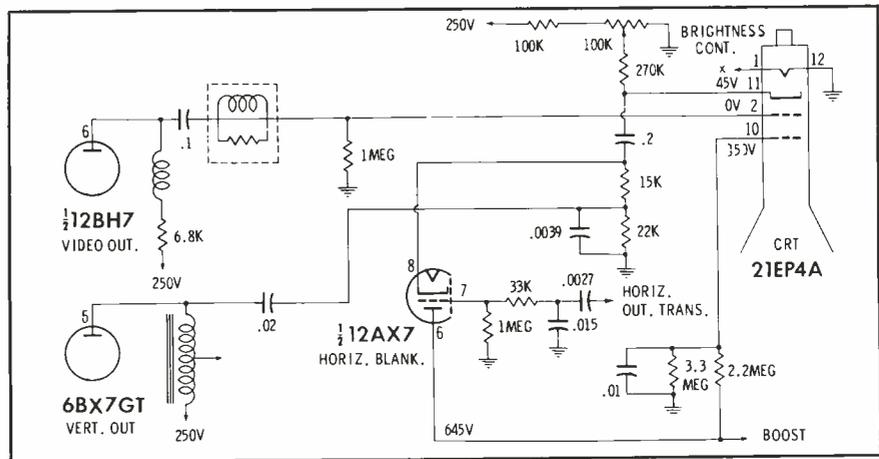
Fig. 4. Blanking-amplifier circuit in GE receiver.
