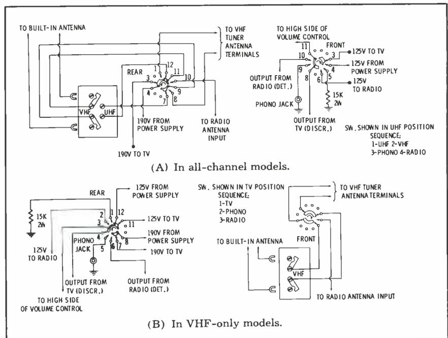
Fig. 6. Function-selector switch in Emerson Port-O-Rama receiver.
