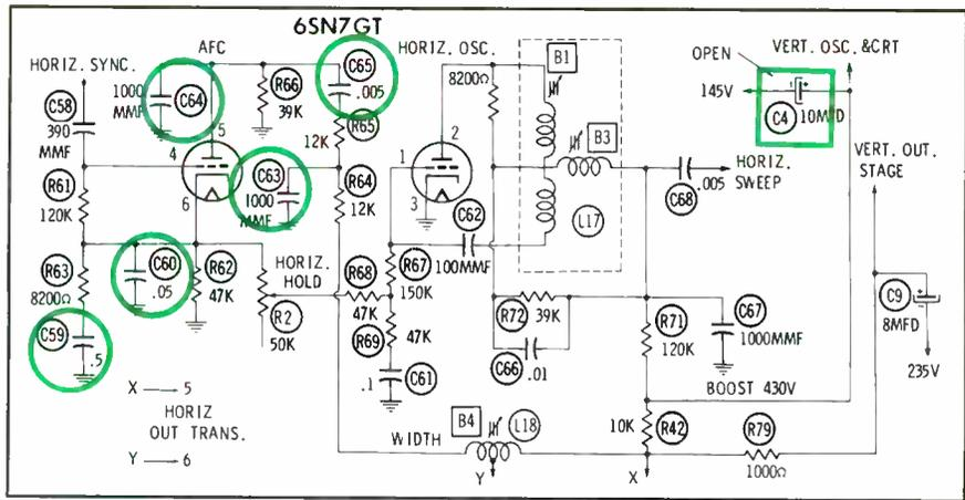
Fig. 4. Horizontal oscillator and AFC in Hallicrafters set.
