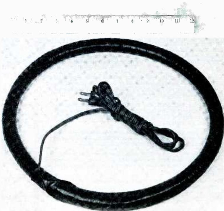
Fig. 1. Degaussing coil to demagnetize color tubes.
