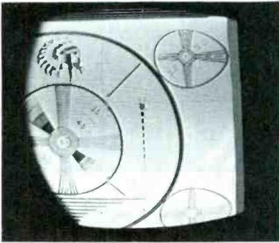
Fig. 5. Raster and picture edges after pulling condition was cured.
