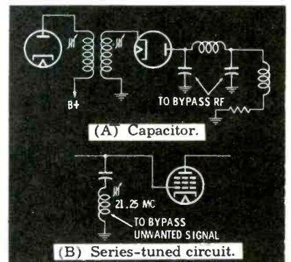
Fig. 2. Frequency bypass devices.
