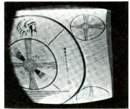
Fig. 2. Horizontal pulling in picture, but not in raster.
