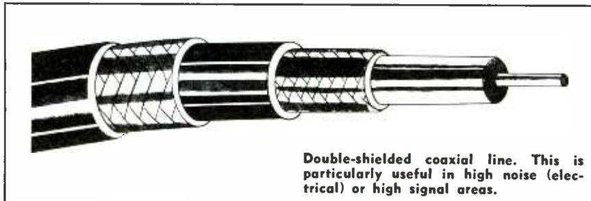
Double-shielded coaxial line. This is particularly useful in high noise (electrical) or high signal areas.
