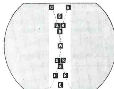
Fig. 3. Relationship between dots in the center row without dynamic correction.
