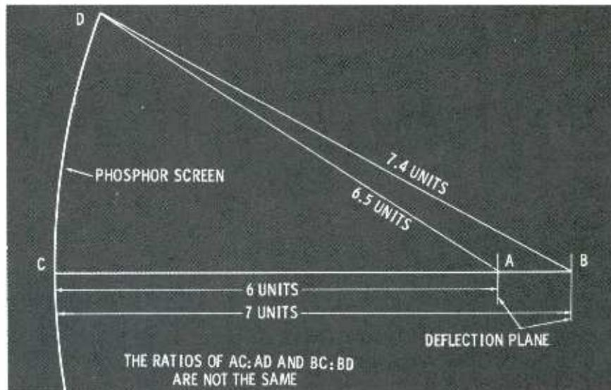
Fig. 2. Geometric drawing showing that a change in the deflection plane of a color picture tube changes the ratio between the distances to the center and to the edge of the screen.
