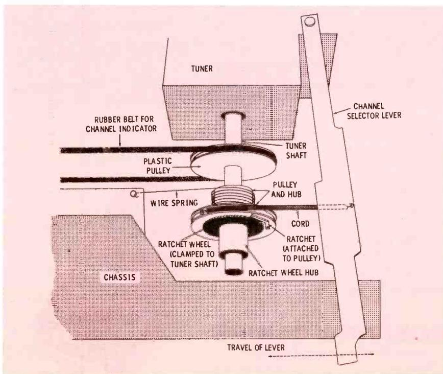
Fig. 2. Lever-operated tuning device in Sylvania Chassis 1-533-7.
