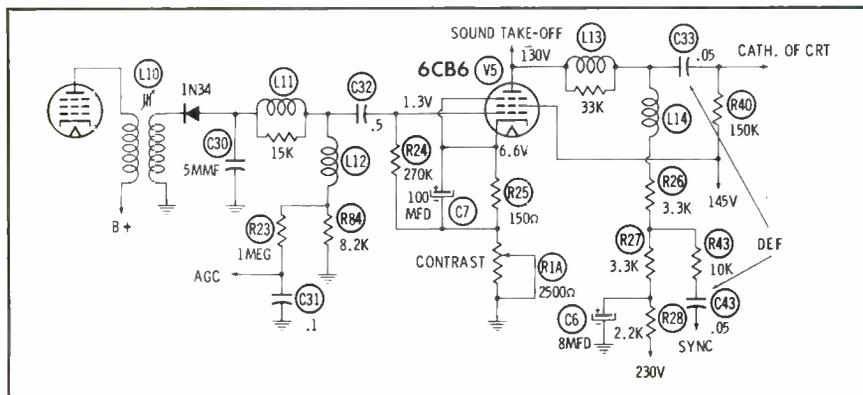
Fig. 3. Video section of Hallicrafters TV receiver.
