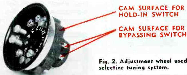
Fig. 2. Adjustment wheel used in Crosley selective tuning system.
