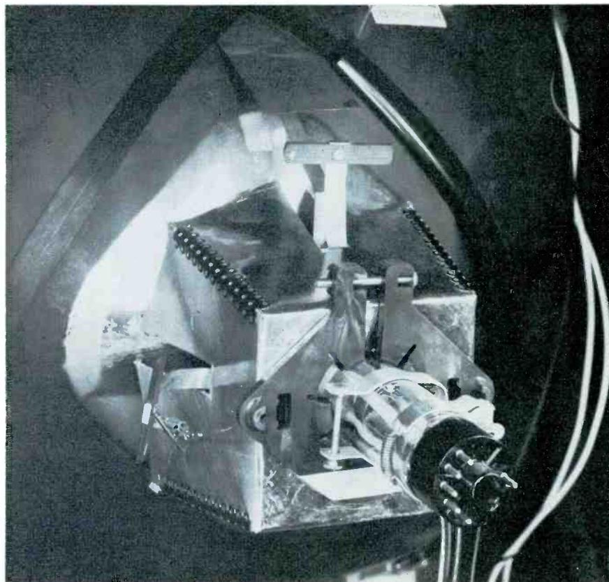
Fig. 1. Shield to cut down yoke radiation in Sylvania Chassis 1-533-7.
