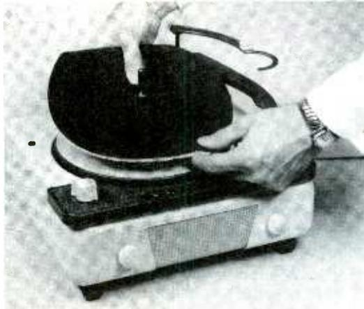
Fig. 1. Installing foam-rubber pad.
