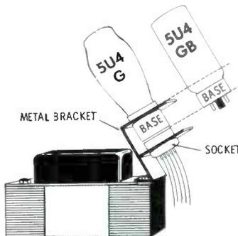
Fig. 6. Mounting of 5U4 tubes in 1954 and 1955 Sylvania receivers.
