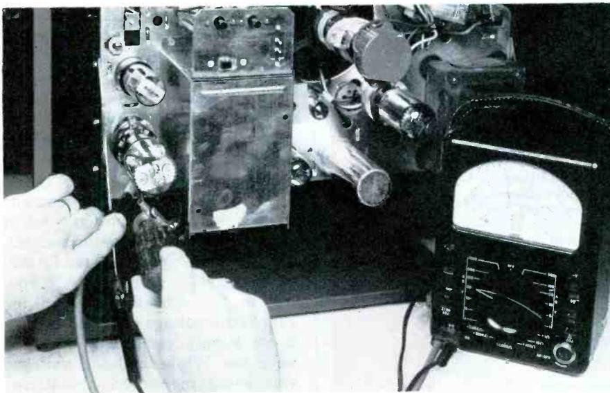
Fig. 1. Adapter socket and VTVM being used to check horizontal-output tube bias.
