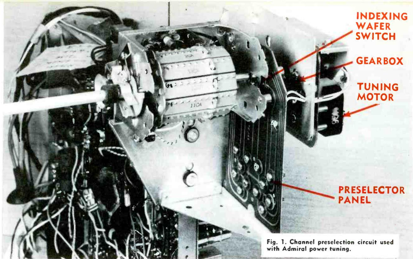
Fig. 1. Channel preselection circuit used with Admiral power tuning.
