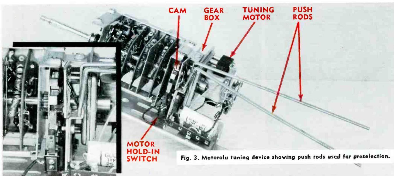
Fig. 3. Motorola tuning device showing push rods used for preselection.
