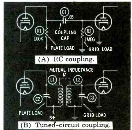
Fig. 1. Types of interstage coupling.
