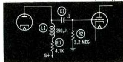
Fig. 3. Frequency peaking circuit.
