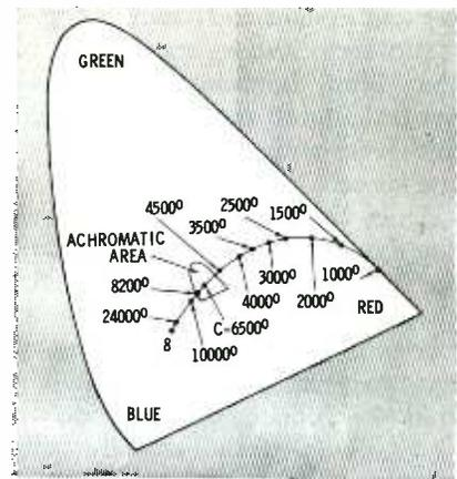
Fig. 6. Temperature gradients plotted on chromaticity diagram.
