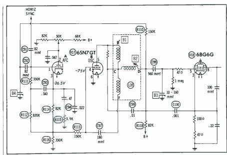
Fig. 14. Schematic of the pulse-width AFC and blocking-oscillator circuits.
