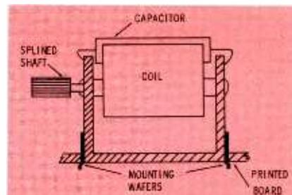
Fig. 3. Mounting details for the horizontal-oscillator coil in Sylvania TV.
