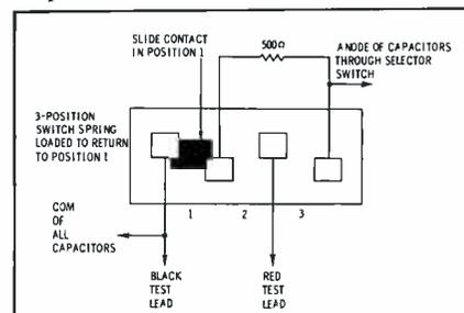
Fig. 5. Slide switch automatically provides surge protection for capacitors.
