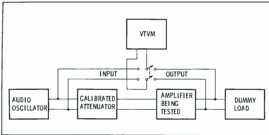
Fig. 3. Setup for testing frequency response employs a calibrated attenuator.
