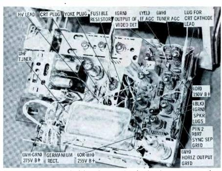
Fig. 3. Topside view of Philco Chassis 9L37 showing important test points.
