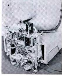
Fig. 2. Chassis can be operated while upended on bench behind the cabinet.
