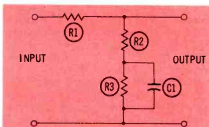
Fig. 1A. Typical bass-boost circuit.
