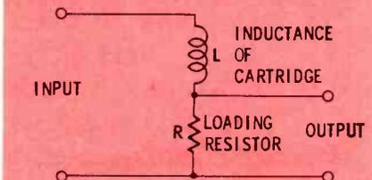
Fig. 1C. Roll-off provided by L and R.
