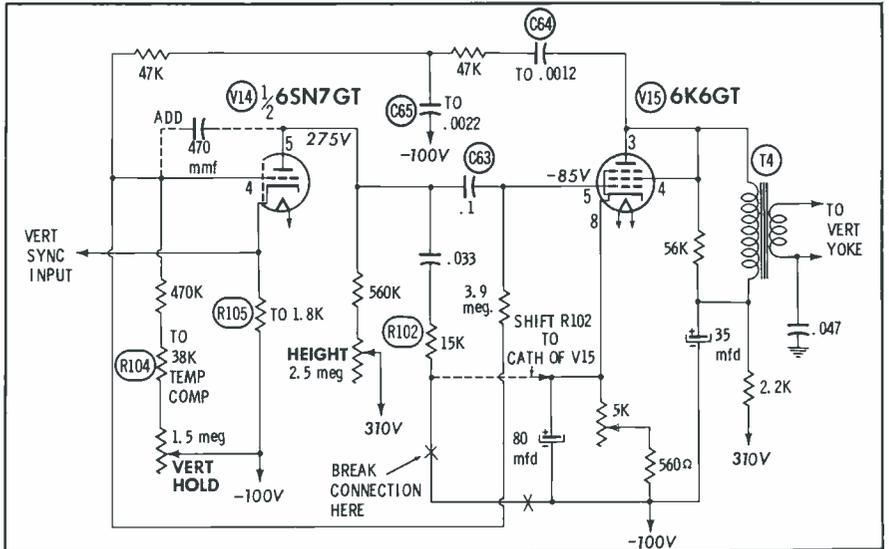
Fig. 5. Schematic of the vertical oscillator and output circuits showing the various changes that should be made to improve operation of the vertical circuit.
