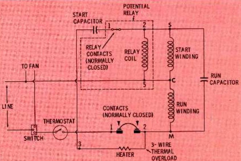
Fig. 5. Alternate circuit using potential relay and 3-terminal overload.
