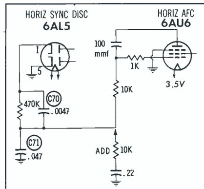
Fig. 11. Horizontal-AFC circuit showing changes to prevent bend in picture.
