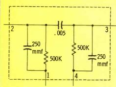
which. A lack of voltage on lead 2 can be caused by a defective tube or an open plate resistor. Check the resistor with an ohmmeter to tell which. If open or increased in value, it can be replaced with an external unit of correct size, providing all other components check good. Apply
