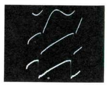
Fig. 16. Key waveforms at oscillator transformer and output control grid.
