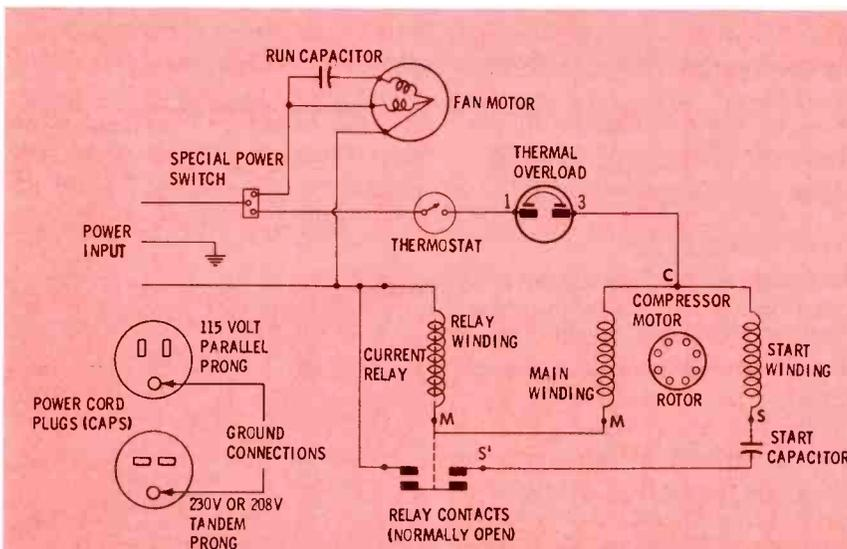
Fig. 2. Electrical circuit for a conventional room air-conditioning unit.
