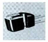
A new Pickering magnetic cartridge, the Stanton 45X45 Stereo Fluxvalve (Model 371) is designed for a tracking force of 3 to 6 gm. Frequency response within the stereo recording range is flat within 2 db when a load resistance of 27K to 47K ohms is used. The unit fits tone arms with ½" mounting centers. Price, including .7-mil diamond stylus, is \$29.85.
