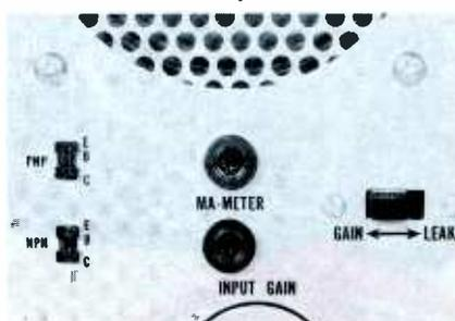
Fig. 3. Front panel provisions of the Hickok tester for checking transistors.
