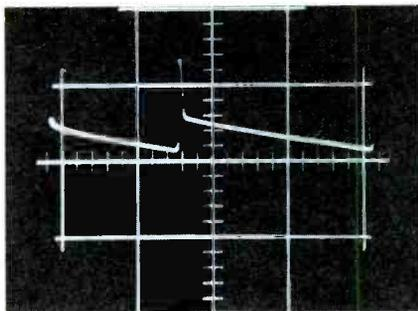
Fig. 8. Vertical-output plate signal should be 1200 volts peak-to-peak.
