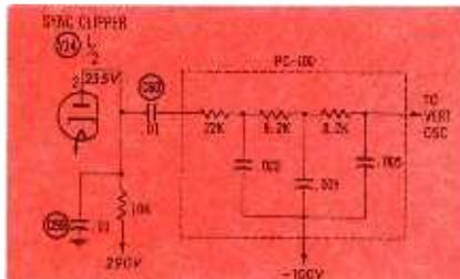
Fig. 2. Partial schematic showing the location of sync coupling capacitor C60.
