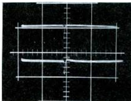
Fig. 3. Lack of separation between waveforms indicates leakage in C60.
