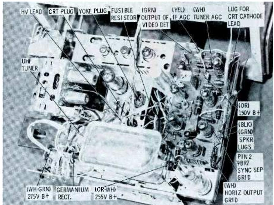
Fig. 3. Topside view of Philco Chassis 9L37 showing important test points.
