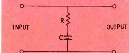
Fig. 1B. Circuit for treble attenuation.
