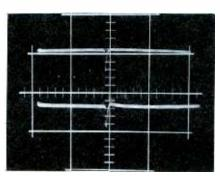
Fig. 3. Lack of separation between waveforms indicates leakage in C60.
