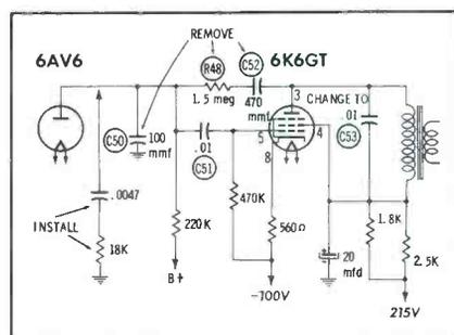
Fig. 9. Schematic of audio circuit showing changes to remove background hiss.
