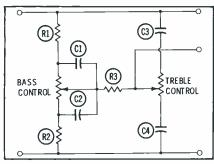
Fig. 4. Tone control circuit provides bass and treble boost and attenuation.
