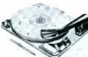
A built-in gauge on the United Audio *Dual-1006* four-speed stereo record changer shows stylus pressure in grams. Records of all sizes from 5" to 12" can be intermixed. Noise produced by spurious vertical stylus motion during monophonic operation is suppressed by the STEREO-MONO switch circuit.
