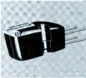
A new Pickering magnetic cartridge, the *Stanton 45X45 Stereo Fluxvalve* (Model 371) is designed for a tracking force of 3 to 6 gm. Frequency response within the stereo recording range is flat within 2 db when a load resistance of 27K to 47K ohms is used. The unit fits tone arms with 1/2" mounting centers. Price, including .7-mil diamond stylus, is \$29.85.
