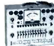
DYNAMIC CONDUCTANCE Tube & Transistor Tester #666
