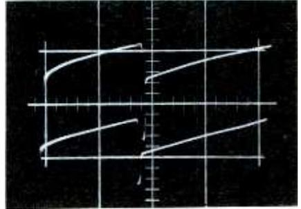
Fig. 7. Normal spacing between the waveforms when C63 has no leakage.
