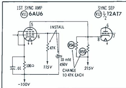
Fig. 12. Schematic showing sync-circuit changes to improve picture stability.
