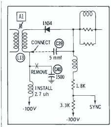
Fig. 10. Video-detector circuit showing changes to prevent harmonic feedback.
