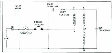
Fig. 6. Permanent split-capacitor motor does not need special start circuit.
