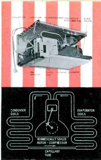
Fig. 1. Diagram showing the flow path of refrigerant used in air-conditioners.
