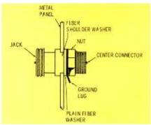
Fig. 1. Installation of miniature microphone connectors improves VTVM value.
