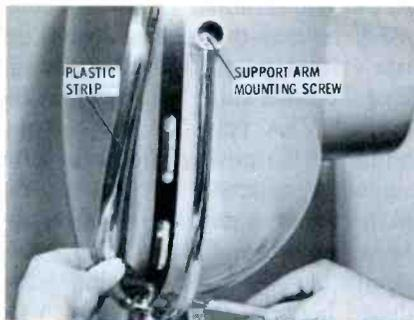
Fig. 5. To disassemble CRT housing, pry off plastic strip around its rim.
