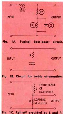
latter case, however, signal amplitude is decreased below its normal level. If C1 is open, the impedance across the output is considerably higher, resulting in greater voltage output, but there is a loss of bass boost. If R3 should open, boost will be excessive and hum level will increase.
