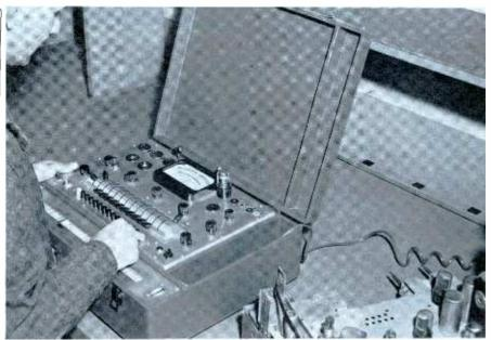
Fig. 4. Making use of Precision's Electronamic tube tester in the laboratory.
