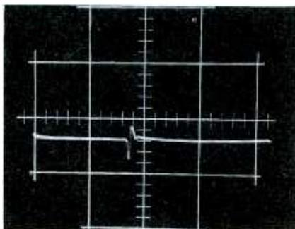
Fig. 1. Defective waveform at the output of the vertical integrator assembly.
