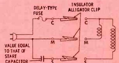
Fig. 4. Test harness for use on standard capacitor start and run circuits.
