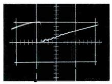
Fig. 17. Expanded waveform at grid of horizontal-output tube shows transients.
