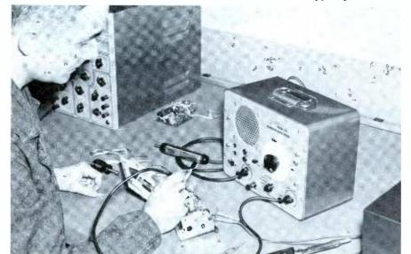
Fig. 1. Signal-tracing, substitution, and alignment of transistor radios is easy with Hickok's Model 810, which also featuers a test circuit for transistors.
