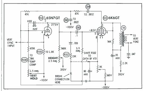
Fig. 5. Schematic of the vertical oscillator and output circuits showing the various changes that should be made to improve operation of the vertical circuit.
