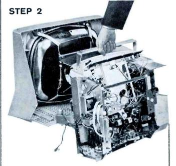
Just two more screws remove the entire chassis! If it ever becomes necessary to pull the chassis, simply remove two more screws and lift it out. The dualette carrying handle becomes a carrying handle for the chassis!
