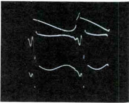
Fig. 15. Simultaneous display of signals in horizontal-AFC and oscillator stages.
