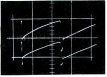
Fig. 6. Spacing of waveforms on either side of C63 indicate leakage in C63.
