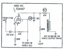
of the signal at the transformer winding was 450 volts p-p. R77 and C53 in series act as a load across this winding; and, since the impedance of C53 at 15,750 cps (in ohms) is equal to only about one-fifth of the ohmic value of R77, about fourfifths of the pulse voltage will appear across the resistor.
