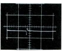
Fig. 1. Defective waveform at the output of the vertical integrator assembly.
