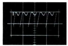
Fig. 19. Setting of the hold control must not affect waveform at terminal C.
