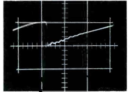
Fig. 17. Expanded waveform at grid of horizontal-output tube shows transients.
