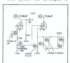
Fig. 13. Schematic showing the changes necessary to update the AGC circuit.
