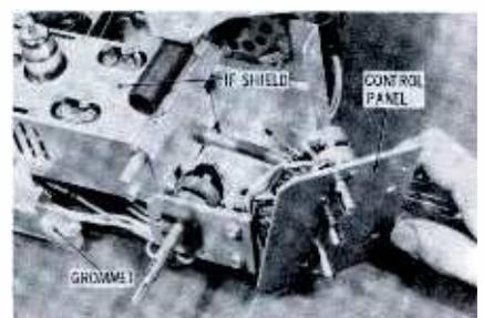
Fig. 4. When removing IF shield, loosen control panel for access to screw.
