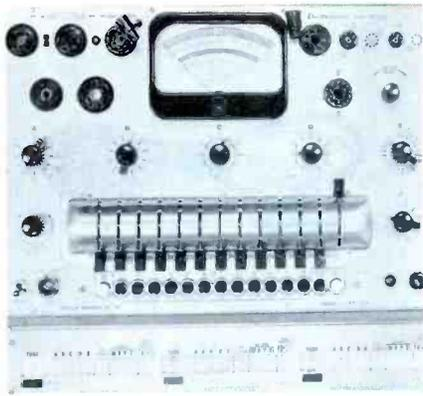
Fig. 5. Model 10-40 panel has easy-to-read meter and 3-window roll chart.
