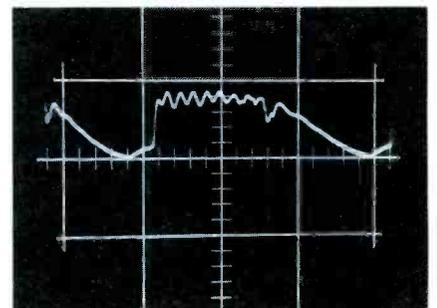
Fig. 18. Transients in the signal at screen grid of horizontal-output tube.
