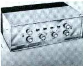
The Arkey CS-28 incorporates dual 14-watt stereo amplifiers and a pair of control preamplifiers, all on a single chassis. A reverse-stereo switch (for interchanging channels) and a balance control are included. Output taps are provided for speaker impedance of 4, 8, 16 and 32 ohms. Price is \$64.95 (kit) or \$99.95 (wired).
