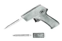
The tool is comprised of a basic trigger-operated handle which accepts the plug-in powerheads, Weller states that integral soldering points have special coating to eliminate corrosion and to assure a life expectancy of 30,000 soldering connections.
