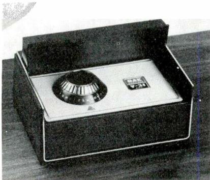
**Features:** Jewel Case V-31 Converter, a varactor unit, eliminates fine tuning by incorporating automatic frequency control (AFC) into the converter itself. Elimination of fine tuning reduces possibility of home owner incorrectly tuning his TV, a prime cause for maintenance calls by the cable system operator. This system offers 31 possible viewing channels spread over the 54-88 MHz and 120-376 MHz ranges.
