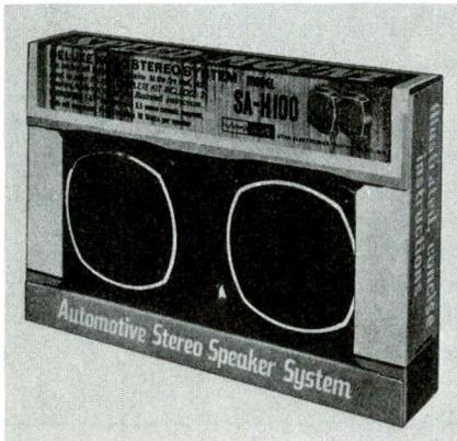
**Features:** 1-3/4-pound ceramic-magnet structures power the 5-1/4-inch high-fidelity speakers which have high-compliance cloth-roll suspension and separate treble cones for full-range music reproduction. Rated at 12 watts, the SA-H100 system includes black, silver-trimmed cases, color-coded wiring, hardware, and illustrated instructions.
