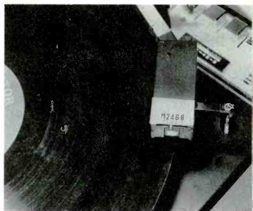
**Step 10** This is the vertical tracking adjustment on a high-quality turntable. You saw a cartridge in Session 1 that needed this adjustment corrected. It looked sideways in its mounting, viewed from the front. The stylus can't seat properly in the groove unless this is right.
