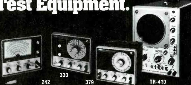
**EICO 242 FET-TVOM.** Peak-to-peak measurements of AC volts and milliamps. 6½" meter. 7 non-skip ranges. High input impedance. Low 1 volt scale. DC/AC Multi-Probe. AC or battery operated. Kit \$79.95, Wired \$109.95.
