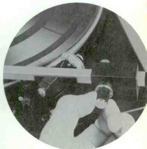
**Step 7** The tone arm shown here has a sliding counterweight moved by a friction knob. The grams knob, the white one on the other side of the mounting post, is typical of medium-price automatics.
