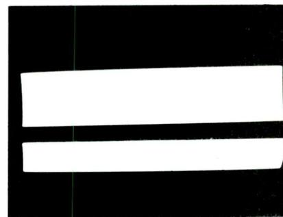
(C) Another way to be sure the oscillator is oscillating is to connect the scope to the oscillator circuit (using a low-impedance point if possible), then noticing how much the amplitude of the scope trace decreases when you touch certain parts of the circuit. The top trace is the normal-amplitude one, while the bottom waveform shows the decrease of amplitude when a finger touched the hot terminal of the oscillator-tuning capacitor.
