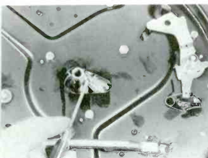
Step 4 In the photo at left is a view of the trip pawl in the tripped position. The turntable platter is off, but you can see its hub in the inset photo. The projection catches on the pawl, dragging the cycling cam into mesh with the gear teeth of the platter hub. You can see, in the photo on the right, the detent lock that holds the cycling cam in place while the record plays; the tug of the trip pawl moves the cam off that detent and into cycle.
