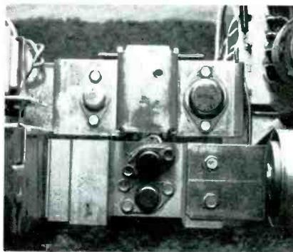
few components, including some in the pin-cushion-correction circuit, are on the PW400 board (usually called the horizontal board), and four transistors plus the remainder of the oscillator and driver stages are on module MAG001B, which plugs edgewise into PW400. Also, the emitter fuse/resistors of the output transistors are on the front side of the chassis, opposite the high-voltage section.
