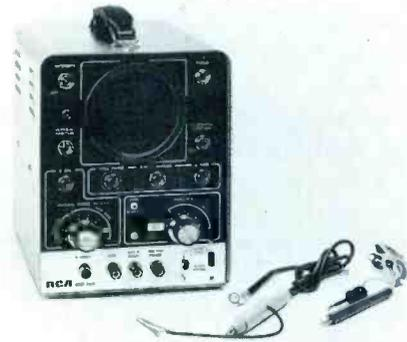
Model WO-33B scope sells for \$229, complete with direct/low-capacitance probe and cable and a special probe for the Quicktracer tests. Probes for signal tracing or RF-demodulation are optional.
