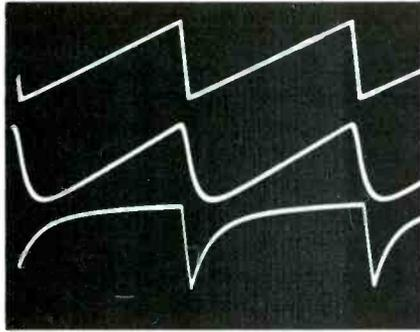
**Fig. 5** Sawtooth waveforms also exhibit some changes because of poor frequency response. The top trace shows the generator sawtooth waveform for reference; in the middle is the result of high-frequency attenuation (the same as in Figure 3E); and the bottom trace is the result of low-frequency attenuation (as in Figure 4D). These waveform changes are not so distinctive as those with square waves.
