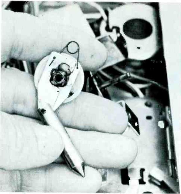
**Step 11.** Power reaching the coil of the solenoid produces a magnetic field that pulls in the plunger. Two spring-loaded pawls (one for pull and one for push) mount on the plunger (sometimes on a lever pulled by the plunger). The two pawls straddle a ratchet gear on the track-change cam assembly.
