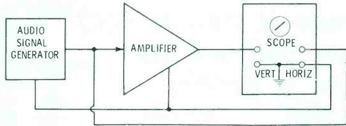
**Fig. 8** Lissajous patterns can be produced by using the same generator signal as input for the amplifier being tested and also as the source of horizontal sweep for the scope. Usually, the vertical and horizontal gains are adjusted for equal deflection, say 4 centimeters each.
