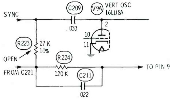
**Symptom**—Linearity stretched at top, insufficient height at bottom
