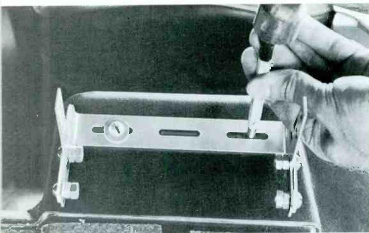
**Fig. 4** Hold the mounting bracket in place while you mark the position for the first mounting screw. After drilling that one, use machine screw, nut, lock washer, and flat washers to secure the bracket as you drill for the second (and third, if needed) screw. This assures that the holes match.
