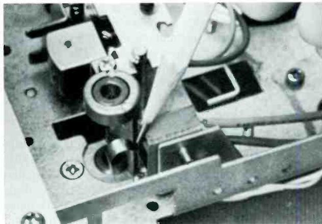
**Step 2.** As the cartridge seats fully into the slot, it presses an actuator which closes a microswitch (leaf switch in some machines), applying power to the motor. The actuator slides in a groove in the capstan housing assembly. The actuator may mount on the chassis or on the microswitch bracket and simply bend against the switch when the cartridge presses on it. I've removed the flywheel so you can see the actuator.
