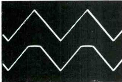
**Fig. 6** Triangular waveforms can be made by severe high-frequency filtering of square waves. Therefore, the high frequencies are very low in amplitude, making this waveform not acceptable for frequency analysis. However, the straight sides and sharp tips are excellent for showing non-linearity (causes slopes to be curved) and clipping, as shown in the trace at the bottom.
