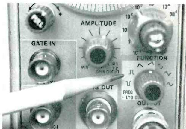
Fig. 8 Sine, triangle, and square waves from .1 Hz to 11 MHz, or ramp and pulses of either polarity from .01 Hz to 1.1 MHz are produced by the FG-502 function generator by Tektronix.
