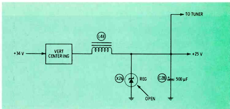
**Fig. 6** High supply voltages can zap tuner transistors. An open X26 zener raised the tuner voltage in this 4B25C19 Zenith chassis.
