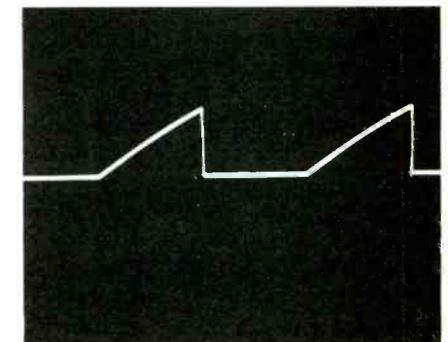
Fig. 15 A sample of Q102's collector current is obtained by R604, which is connected between collector and ground, and used as negative feedback (through the height control) to the collector of Q1. If this 1.8 volt PP signal is missing, locking will be with the hold control at one extreme.
