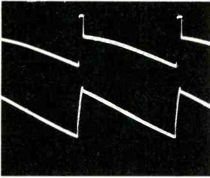
Fig. 9 The 48 volt PP vertical deflection signal from the emitters of Q101 and Q102 is shown by the trace at the top, and the 2.4 volt PP waveform of the bottom trace is the waveform of yoke current, which is obtained by routing the cold end of the yoke through R13 on MAG001B.
