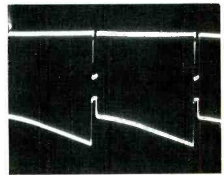
**Fig. 8** Q3, the driver transistor, has these signals: at the base (top trace) there is +.5 volt DC at 1.5 volts PP; and the collector has +35.5 volts DC and 48 volts PP (bottom trace). Because the output transistors are emitter followers, the collector waveform of Q3 is nearly the same as the output signal from Q101 and Q102.
