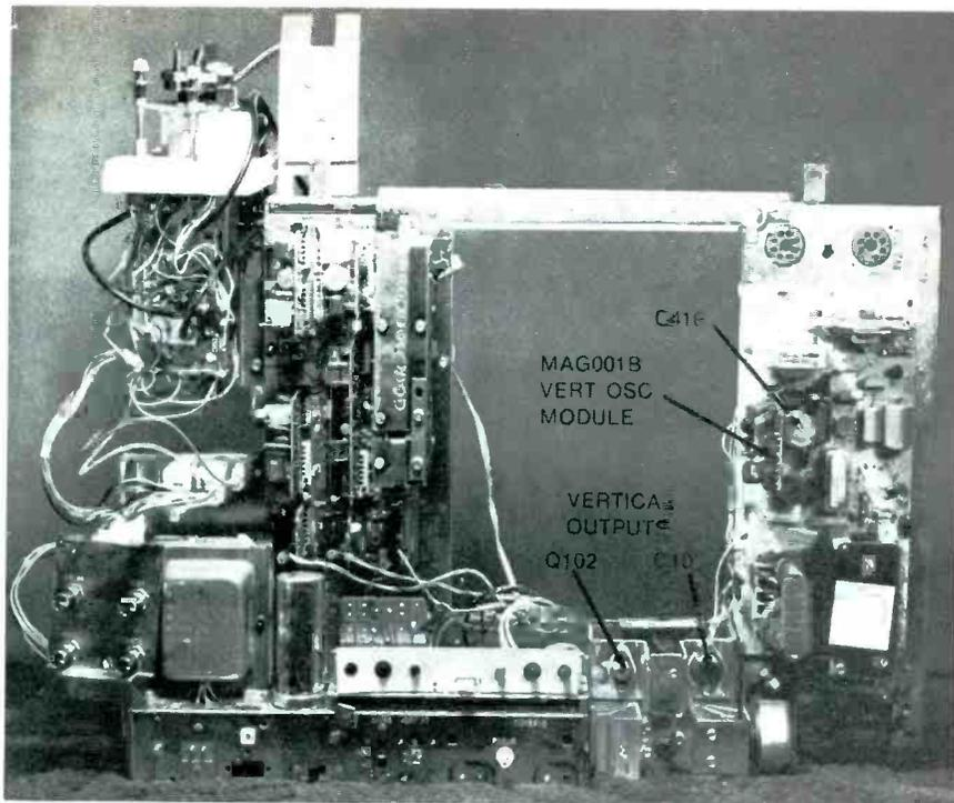
Fig. 1 Components for vertical deflection are located in several areas of the RCA CRC58 chassis.
