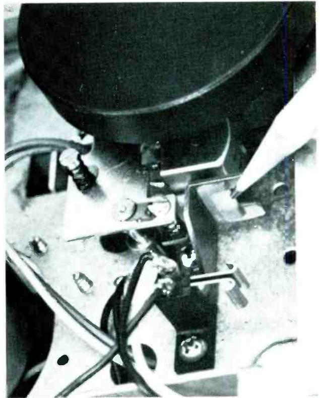
**Step 9.** In operation, as the tape moves across the head, a guide holds the tape at the correct height to match the tracks with the head gaps. To reduce friction, you often find a plastic insert in the slot of the tape guide. Should this insert come loose, tapes wear excessively. Some inserts can be replaced. On other machines, you have to replace the entire tape-guide assembly.
