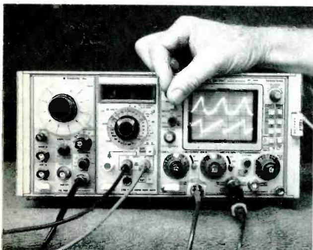
Fig. 9 The new super-bright SC-502 dual-trace 15-MHz scope is on the right, DM-502 digital meter in the center, and the FG-502 function generator is in the left compartment. This combination works well for almost any kind of service, including TV.
