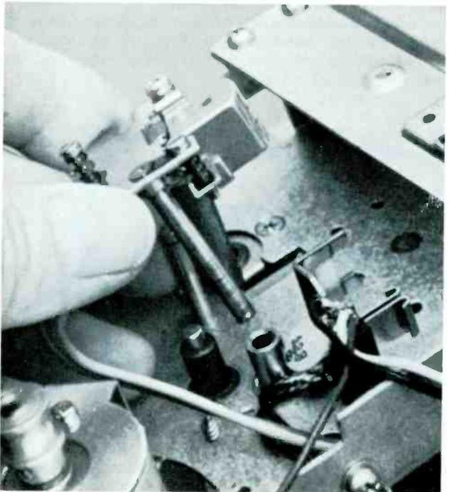
**Step 14.** The head plate mounts at the top end of the lift-rod shaft. Its alignment keeps the head at the proper angle to the tape. If the rod binds, the head can't change tracks properly when the cam rotates. The head-tension spring is another suspect; it might be weak or missing.
