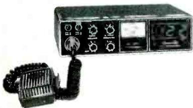
The dual-conversion receiver has three ceramic IF filters, tuned-RF stage, either positive or negative ground, and a meter that shows power during transmitting or signal strength for receiving.
