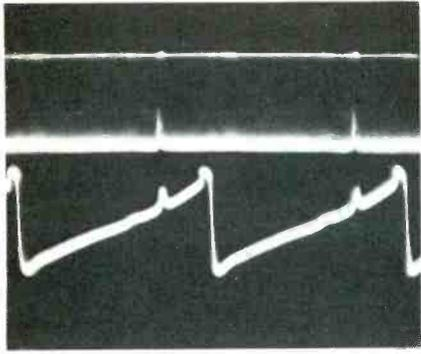
**Fig. 4** At MAG001B pin 12, 28 volts PP of sync enters the module (top trace). After integration of the sync, both it and the positive-feedback signal are applied to the base of Q1. For the lower trace, the vertical was given a slow roll to separate the small sync pulse from the larger feedback signal (2 V PP).
