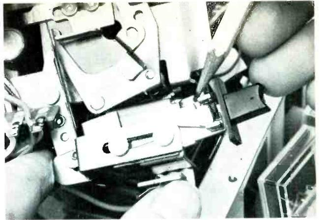
**Step 18.** A latching assembly catches the pause slide and holds it in the pause position. But when you push the Pause button again, the mechanism releases the slide, allowing all assemblies to return to whichever mode the unit was in. If the pause slide doesn't latch or release properly, check the latching assembly. Make sure it's free of caked lubricant and grime, and that its springs haven't slipped out of position or broken.
