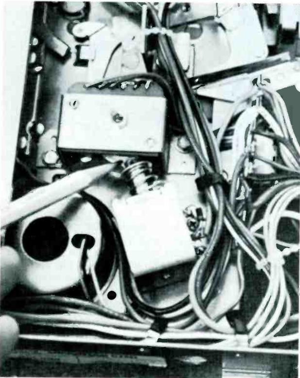
**Step 12.** When the solenoid moves the plunger, one pawl tugs on the ratchet gear, rotating the cam assembly 1/8 turn. Then power ceases to activate the solenoid, and a heavy spring returns the plunger. The other pawl pushes the ratchet gear, rotating the cam assembly 1/8 turn further. If the cam assembly doesn't rotate when you actuate the solenoid electrically or manually, check the ratchet gear and pawls for wear. Make sure they're lubricated. The pawl spring may be weak or even missing.
