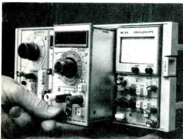
Fig. 7 Modules can be removed or reinstalled in seconds and without tools.
