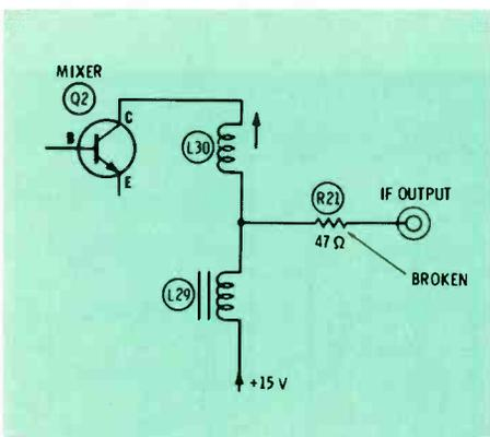
**Fig. 5** A broken resistor decreased the gain of a tuner in an RCA CTC59. It might have broken when the IF cable was removed; use care in handling all cables.
