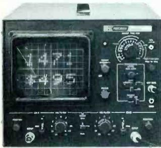
Vertical-deflection sensitivity has 11 ranges between .01 volt-per-centimeter and 20 volts-per centimeter.
