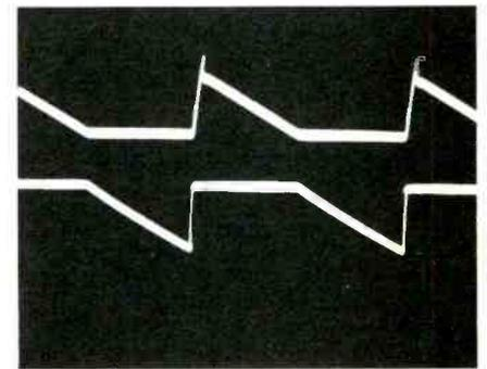
Fig. 14 Voltage drops across the emitter resistors of Q101 (top trace) and Q102 (bottom) show good balance and linearity of the output transistors.
