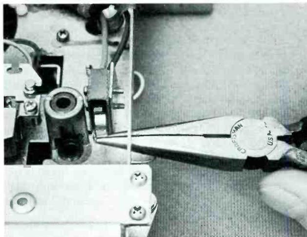
**Step 3.** Regardless of how the actuator mounts, if it gets bent out of shape, it might not close the motor-power switch. Sometimes you can reshape the actuator with long-nose pliers. But it's safer to install a new one. You can check the switch with your VOM to see if the contacts are okay. Push the switch with a pencil eraser to close its contacts. Check for voltage at both terminals.
