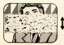
Figure 3 One symptom of a servo problem which allows a video head or capstan to run at erratic speed is a band of noise that either jerks up and down or remains stationary. Servo problems usually show on the TV screen as alternate periods of good or bad video. alternate periods of good and bad video. Therefore, the symptoms are not like luminance and chrominance defects.
