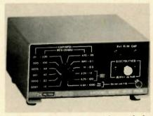
The initial surge is limited by putting a resistor in series with the substitute capacitor. After the capacitor is charged, a switch is moved to the substitute position, removing the resistor from the circuit. For added protection, an overload indicator lamp warns against substitution of a low voltage capacitor when applied voltage is over 75 VDC.
