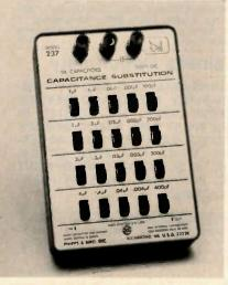
The unit weighs one pound, and is in a metal case. It uses nonpolarized 5% capacitors and features 5-way binding posts. This unit sells for \$95. Circle (34) on Reply Card
