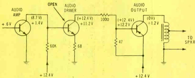
Figure 7 No click or thump could be heard when this inoperative Motorola TM7A was turned on. Usually a power problem or a dead output transistor is responsible.
