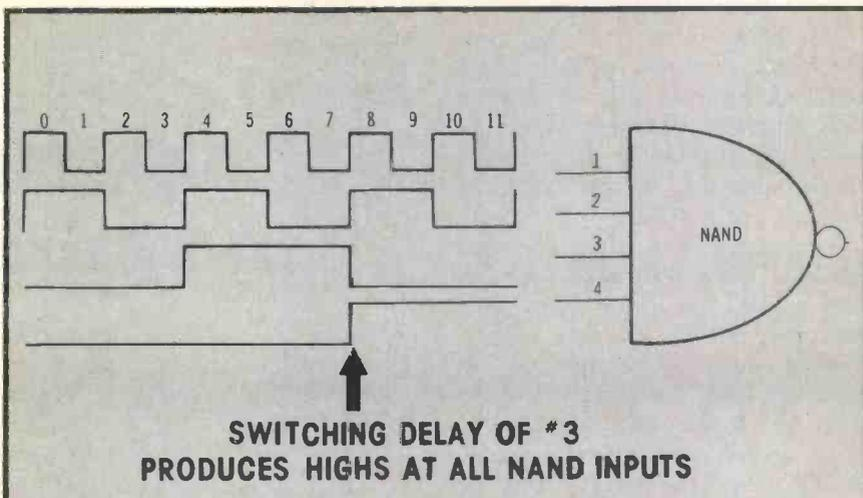
**Figure 6** If the third flip flop signal is slow in dropping to zero at the beginning of the eighth count, all NAND inputs will have highs for a very brief time. However, this is long enough to produce a negative-going glitch at the NAND output, and it stops the count prematurely.
