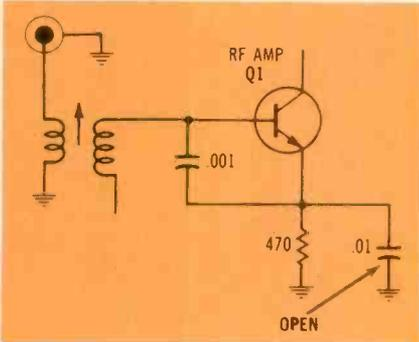
**Figure 3** Intermittently, the model 2HT1413 American Motors radio would become very weak. Only two stations could be heard.
