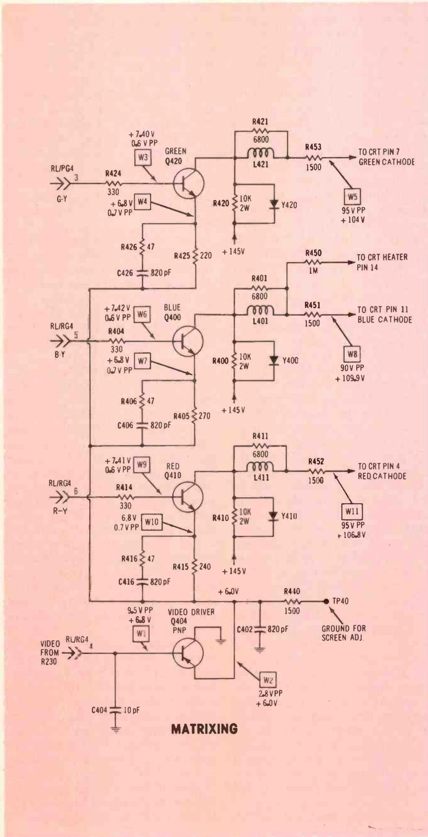
Figure 9 Luminance video and demodulated chroma signals are matrixed inside Q420, Q400 and Q410. Chroma signals are applied to the bases, and luminance signals are applied to the emitters. These four transistors are mounted on the CRT-socket module of Figure 3. Voltages and waveforms were measured during reception of a generator B&W signal, therefore, no chroma signals were there.
