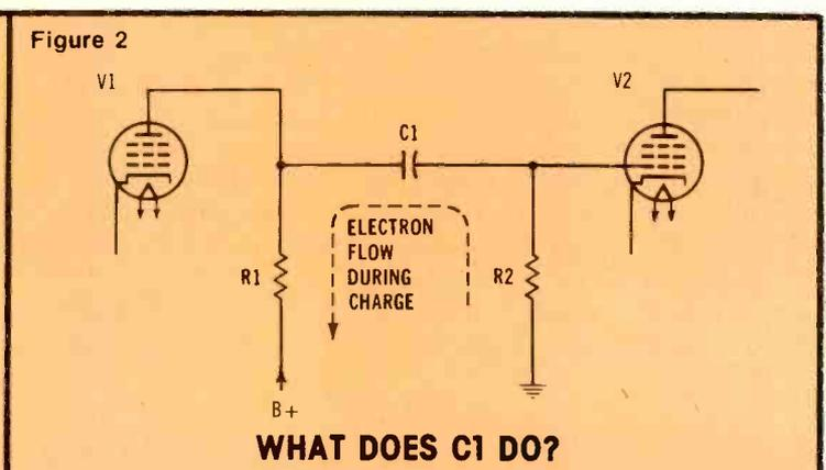
Figure 2 C1 is called a coupling or blocking capacitor. What does it actually do?
