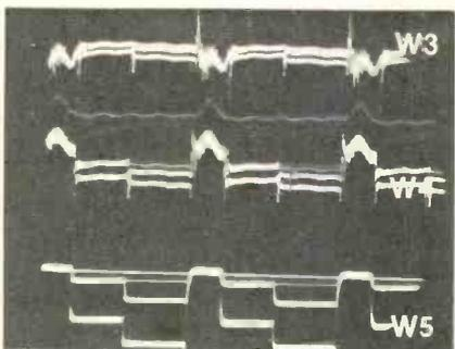
**Figure 10** These waveforms were made when a video generator supplied the signal. The W numbers correspond to those of the Figure 9 schematic.
