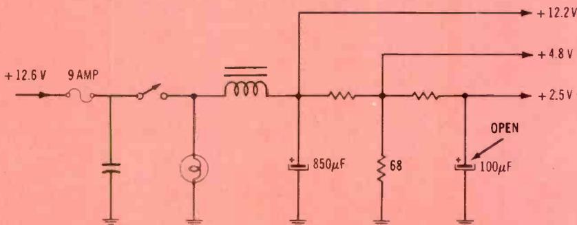
**Figure 12** Motorboating commonly is caused by open filters. This was true of the model 01BP2 Delco radio. Several capacitors were in one can, so the can was replaced, rather than just the one bad section.
