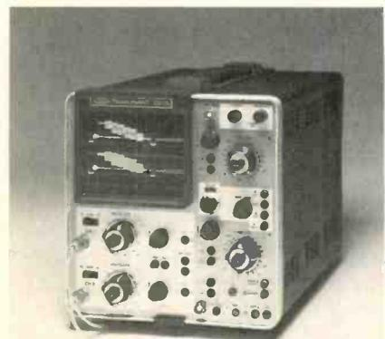
Maximum sensitivity of each vertical channel is 10 mV, and minimum sensitivity is 50 V per division. Bandwidth is from dc to above 15 MHz.
