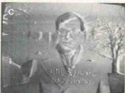
Figure 8 A serious picture degradation occurs when diode Y220 shorts. In A, the top trace is the normal generator video at the Y220 anode. Lower trace shows the distortion caused by a shorted Y220. TV picture B is a normal one, while picture C shows the same TV picture after Y220 was shorted. There is a compression of most shades of brightness plus a trailing smear and the picture was much darker.
