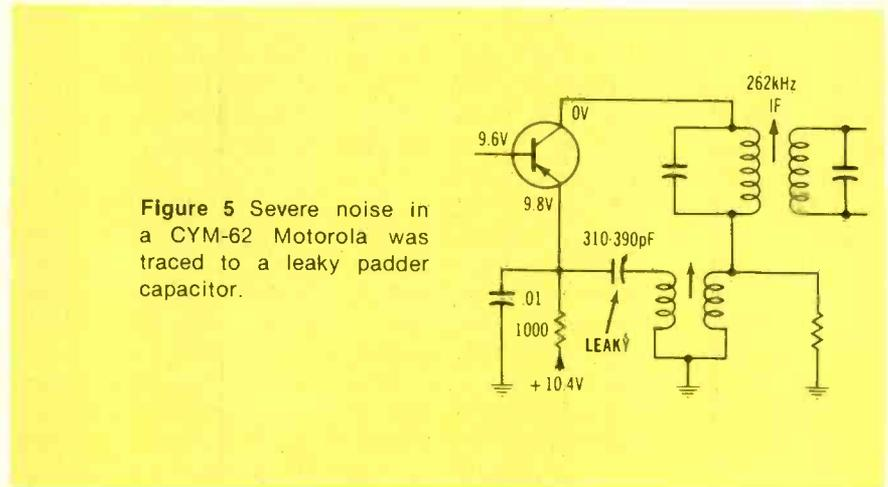
Figure 5 Severe noise in a CYM-62 Motorola was traced to a leaky padder capacitor.
