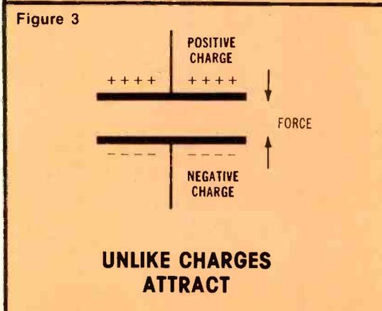
Figure 3 A charged capacitor has opposite charges at the plates. These attract; therefore, work is required to move the plates apart. This work accounts for the increased voltage that occurs when the plates are separated more widely.
