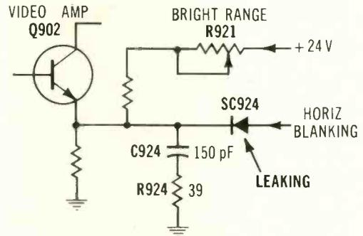
**Symptom**—Horizontal tearing which is changed by brightness
