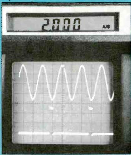
**Figure 10** A 2:1 frequency ratio was measured for these two signals. Two separate generators were adjusted carefully to obtain this condition.
