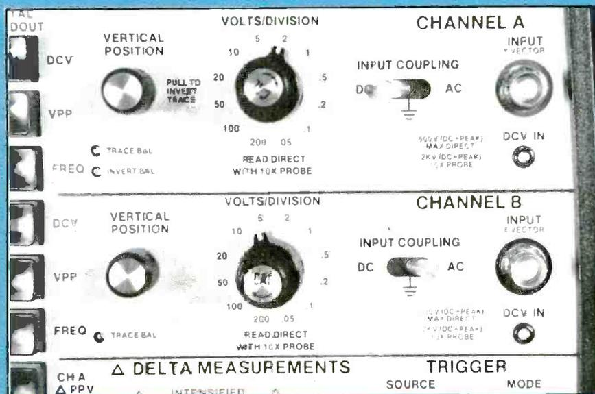
Figure 3 Layout of the vertical-channel controls is shown in this photograph.
