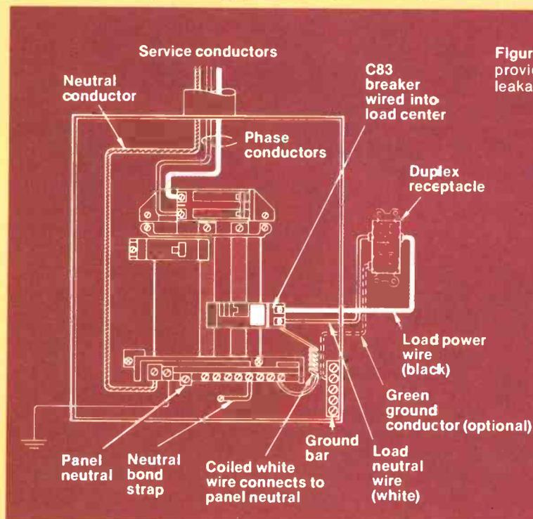
Figure 1a. A ground-fault circuit breaker provides overcurrent protection and leakage current hazard protection.
