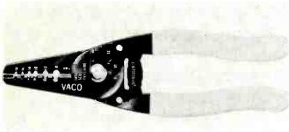
cuts wires, cuts three popular bolt sizes, features a serrated plier nose for pulling wire and has holes for looping and bending wire.
