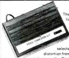
The SWD-1 Video Converter is utilized on cable TV systems to remove the KHz's signal from a distorted video (channel 3 in/out) and also pass thru the normal undistorted/detected audio signal. Rocker switch selects operating mode to remove KHz's distortion from the video or pass all other channels normally. Simple to assemble—less than 30 minutes. Pre-tuned. Input/output Channel 3. Impedance 75 ohms. 117VAC.
