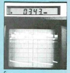
Figure 9 Digital readouts were made of the bottom-trace vertical-output-tube plate waveform. (A) Vertical repetition rate measured 59.94Hz (a reading that is difficult to obtain with some frequency counters). (B) The amplitude measured 1207VPP. (C) The plate voltage measured +343Vdc. No higher accuracy should ever be needed for these circuits.
