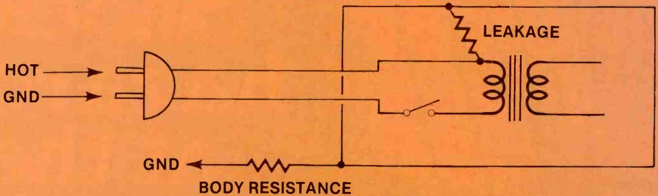
Figure 1. In a 2-wire device with leakage problems, the switch is in the neutral leg; the leakage hazard will exist even if the switch is turned off.
