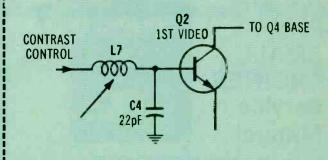
Symptom - Loss of luminance, but color is normal Cure - Check peaking coil L7 and replace if open
