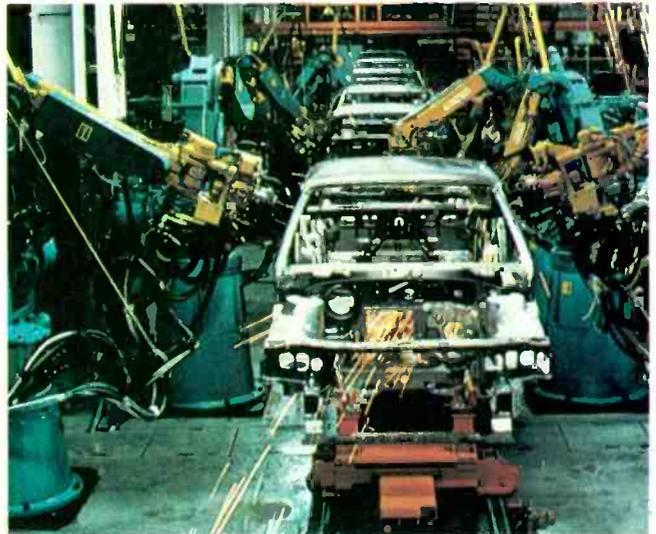
**At General Motors Assembly Division plant in South Gate, CA, fourteen Cincinnati Milacron robots spot weld J-car bodies at a rate of 72 bodies per hour. Robots spot an average of 400 welds on each body.**
