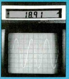
Figure 13 A sinewave was used frather than square waves or pulses) to make more clear the process of measuring rise time by Delta-time mode. The amplitude of a locked waveform is adjusted to the 0% and 100% graticule lines, the waveform rise time is horizontally expanded, then the Delta-time mode is selected and the 10% to 90% slope is covered by rotation of the begin and end controls that make this slope brighter. The LCD readout shows a time that needs no processing or calculations.
