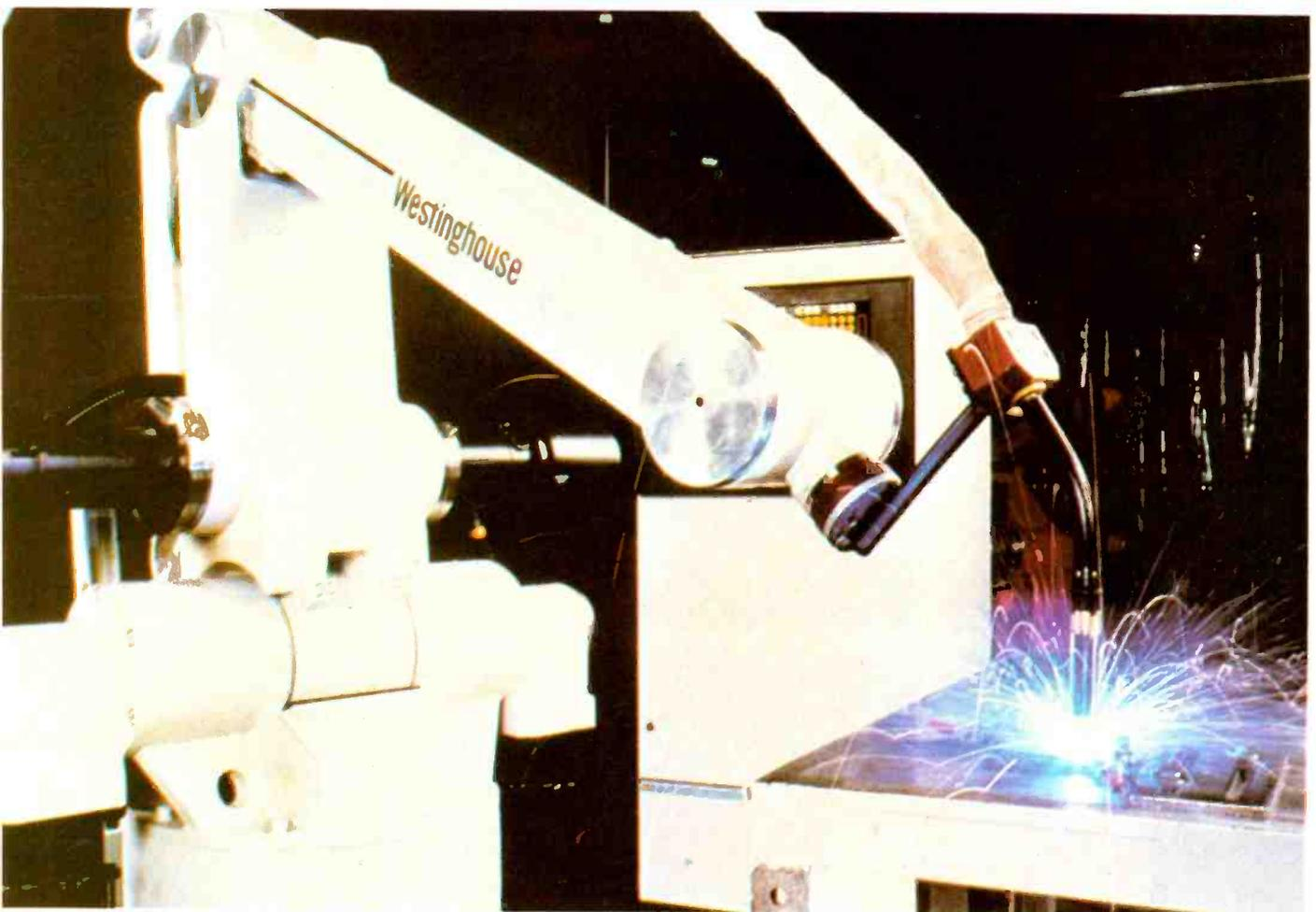
**The Series 4000** by Westinghouse is a low-cost, precision, robotic welding system that uses a pulsed gas-metal-arc welding power source. The four major parts of the system are an electric, servo-controlled, arc-welding robot; a computerized robot control; a pulsed-current welding power source; and a wire feeder.
