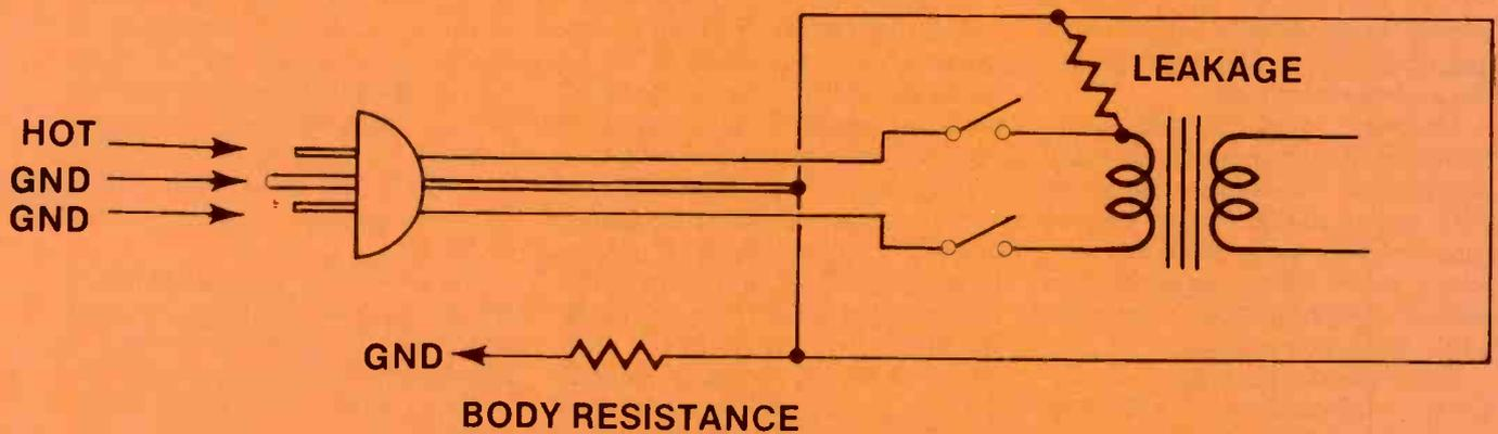
Figure 3. The 3-wire grounding system allows plugging into the receptacle only one way, and provides a grounding path for leakage current.
