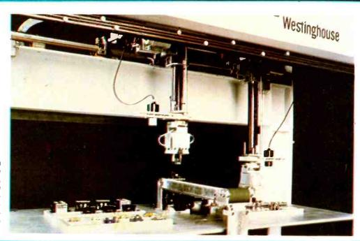
The Series 5000 robot system by Westinghouse is available with one, two or three arms, and can be used to assemble electrical relays and breakers, complex integrated circuit boards, automotive components and complex office machines.
