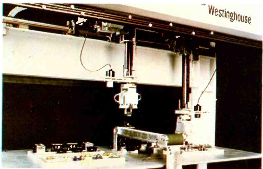
**The Series 5000 robot system** by Westinghouse is available with one, two or three arms, and can be used to assemble electrical relays and breakers, complex integrated circuit boards, automotive components and complex office machines.
