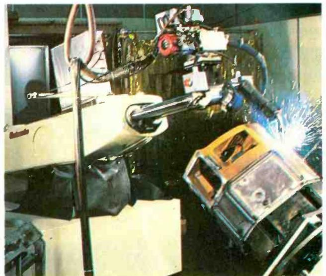
**An example of continuous-path welding** by a Unimate robot at Air Research.
