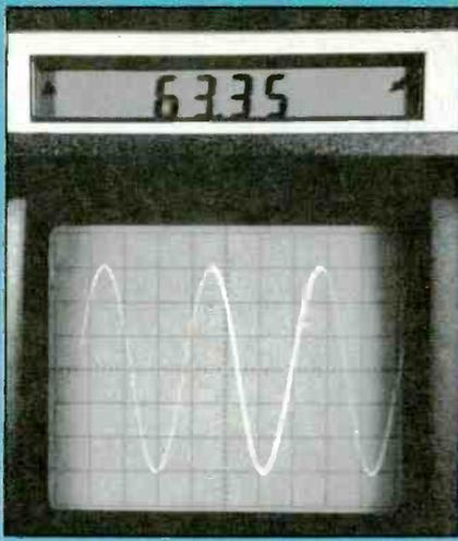
**Figure 12** A sinewave having approximately the frequency of horizontal sweep measured  $63.35\mu\text{s}$  by Delta-time reading. The 1/Delta-time button then gave the calculated frequency as  $15,770\text{Hz}$ , which compared favorably with the counter direct reading of  $15,737\text{Hz}$ .
