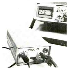
new Fotec C200 uses an external voltmeter to display the results of the measurement.
