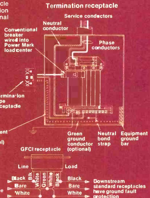
Figure 2a. This ground-fault receptacle features ground-fault protection in a unit that fits a standard receptacle box.
