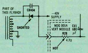
Symptom – No height; new MDG001A vertical module does not help, and resistor R28 on module is too hot Cure – Check diode CR404 and replace with fast-recovery type if shorted
