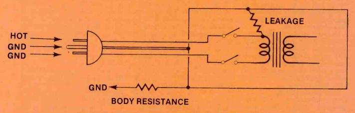
Figure 3. The 3-wire grounding system allows plugging into the receptacle only one way, and provides a grounding path for leakage current.
