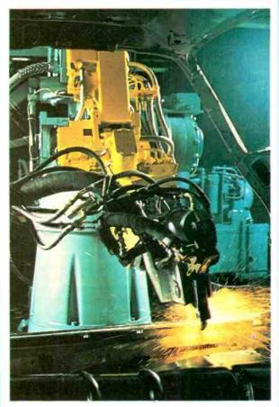
A computer-controlled robot, the T3-586 by Cincinnati Milacron, places spot welds on a car body as it moves past on a conveyor. The tracking capability enables the robot to spot welds without stopping the line.
