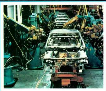
At General Motors Assembly Division plant in South Gate, CA, fourteen Cincinnati Milacron robots spot weld J-car bodies at a rate of 72 bodies per hour. Robots spot an average of 400 welds on each body.
