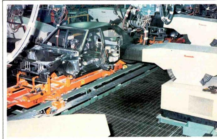
Auto spot welding by a Unimate robot. (Photo courtesy of Unimation.)
