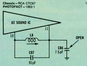
Symptom – Distortion and low sound volume on channel; normal noise off channel
