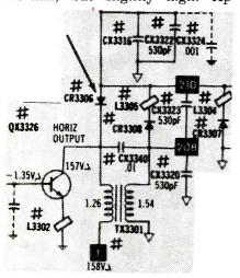
parently, the shutdown circuit was operating to eliminate all scan-rectified power, or there was no horizontal drive to the output transistor.
