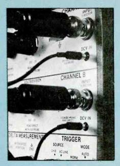
Figure 7 Below each probe socket on the SC61 front panel is a small banana plug that receives dc voltages from the probe. An optional dc-voltage probe can be plugged in, if the scope probe is not desired (for lower-loading measurements).
