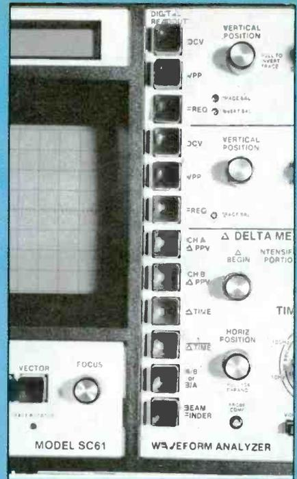
**Figure 6** A vertical line of push-buttons is located at about the horizontal center of the front panel. The top six allow digital Vdc, PPac and frequency readouts from the two vertical channels. Four of the lower six buttons are for the Delta-time measurements, one is the frequency-ratio button and the bottom one activates the beamfinder.
