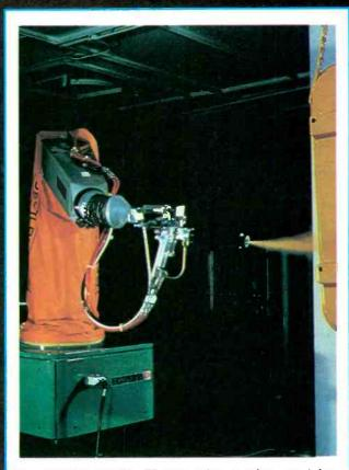
The DeVilbiss/Trallfa TR-3000 robct is often used for spraying paint and other elements involved in manufacturing. Here, the unit sprays a vehicle component with EH8 airless electrostatic.
