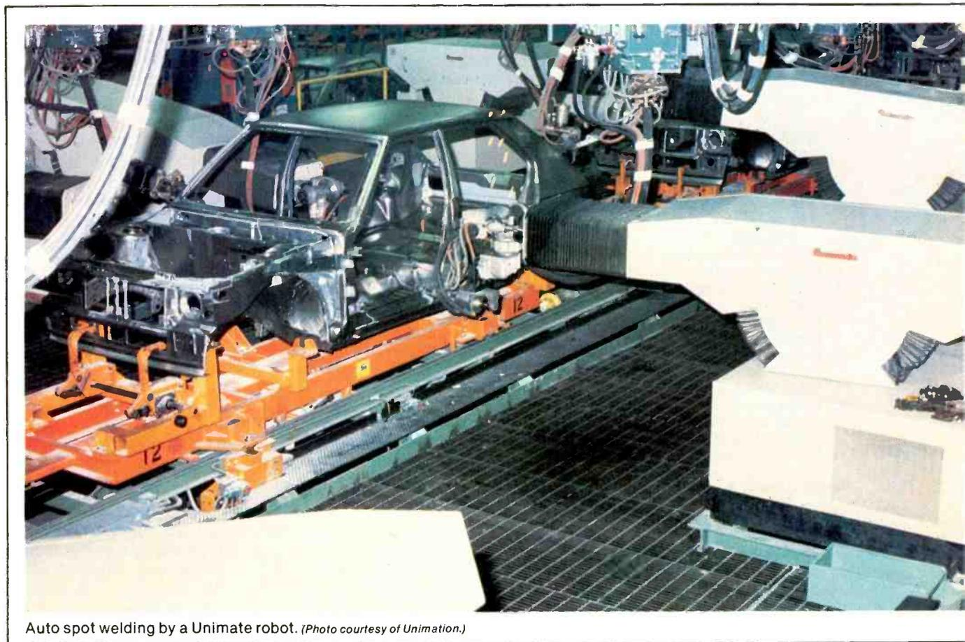
Auto spot welding by a Unimate robot. (Photo courtesy of Unimation.)
