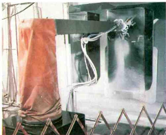
**Refrigerators are only one of hundreds of items being manufactured with the help of robots. This DeVilbiss TRL-3000 is spraying a refrigerator liner with powder coating.**
