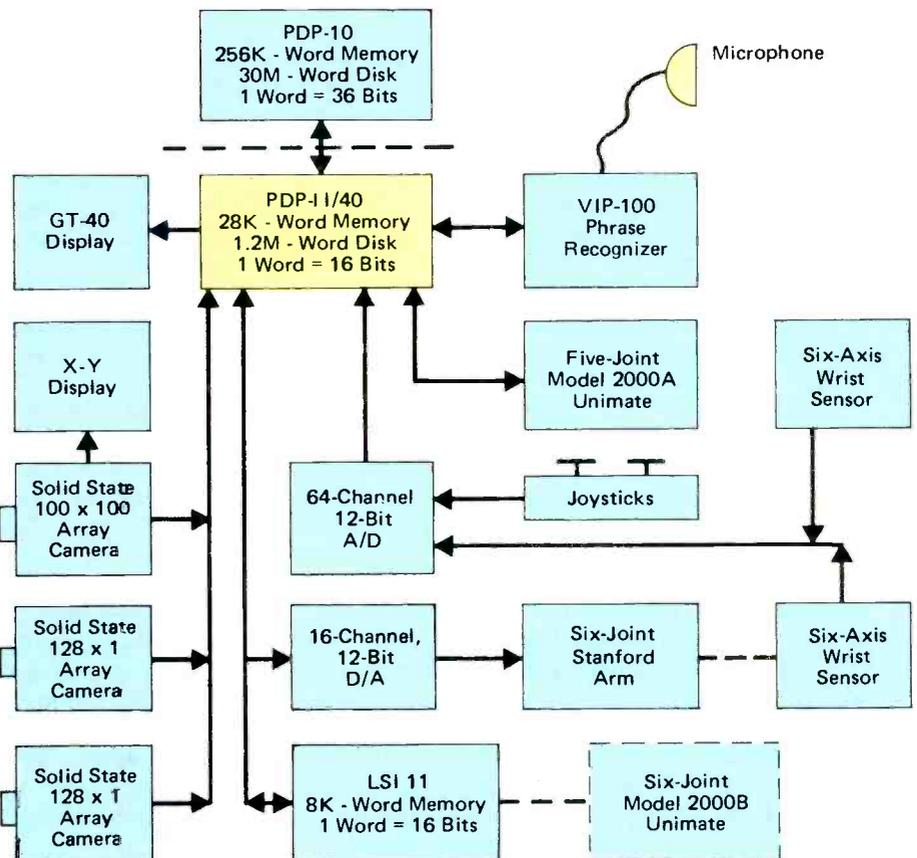
**Figure 5.** A diagram of a laboratory setup for evaluating robot sensory perception and manipulator dynamics.
