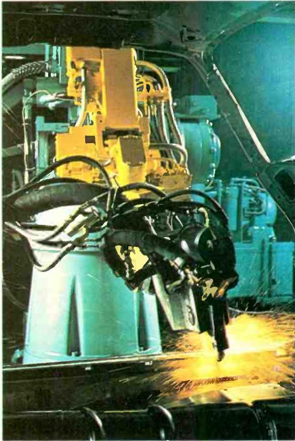
**A computer-controlled robot, the T-586 by Cincinnati Milacron, places spot welds on a car body as it moves past on a conveyor. The tracking capability enables the robot to spot welds without stopping the line.**
