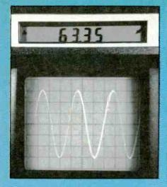
Figure 12 A sinewave having approximately the frequency of horizontal sweep measured 63.35µS by Delta-time reading. The 1/Delta-time button then gave the calculated frequency as 15,770Hz, which compared favorably with the counter direct reading of 15,737Hz.
