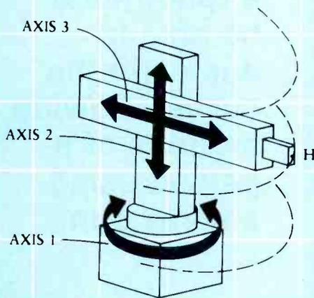
Figure 2. A cylindrical-coordinate robot.
