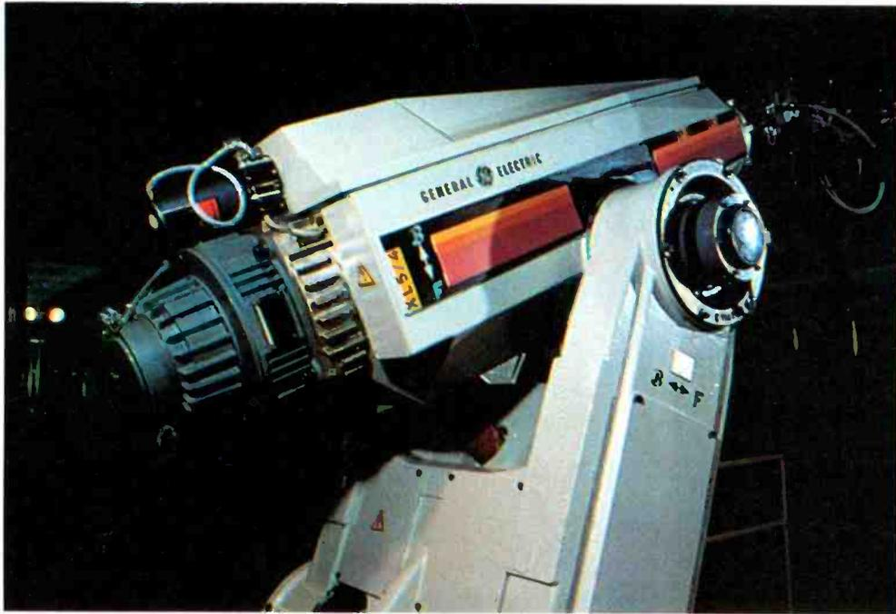
Driven by electric servo motors, the GE robot, GP 132, is a 7-axis, single-arm robot designed for general-purpose material handling.
