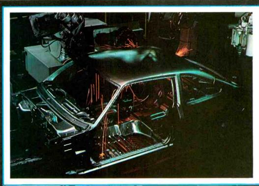
**Unimate robots** by Unimation perform spot welds on an auto body.
