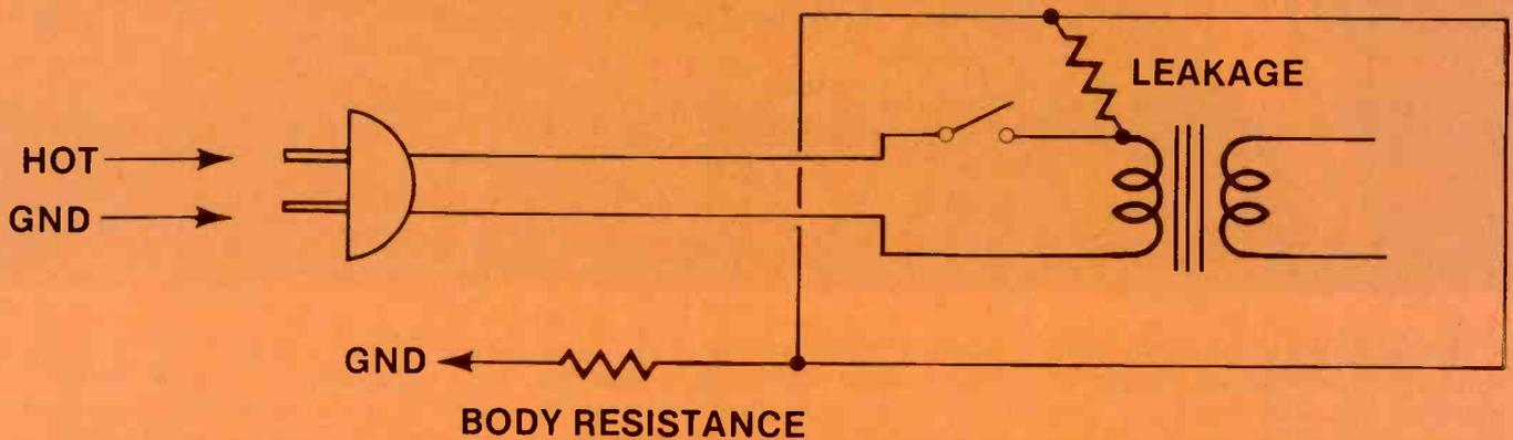
Figure 2. If the switch is in the hot leg, the leakage hazard is removed when the switch is opened.
