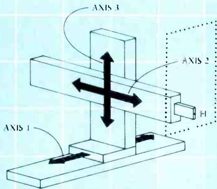
Figure 1. A rectangular-coordinate robot.
