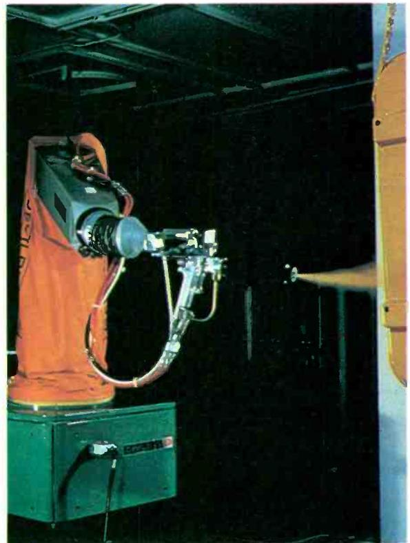
**The DeVilbiss/Trallfa TR-3000 robot is often used for spraying paint and other elements involved in manufacturing. Here, the unit sprays a vehicle component with EH8 airless electrostatic.**
