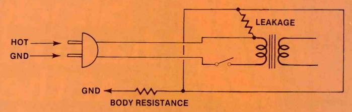
Figure 1. In a 2-wire device with leakage problems, the switch is in the neutral leg; the leakage hazard will exist even if the switch is turned off.
