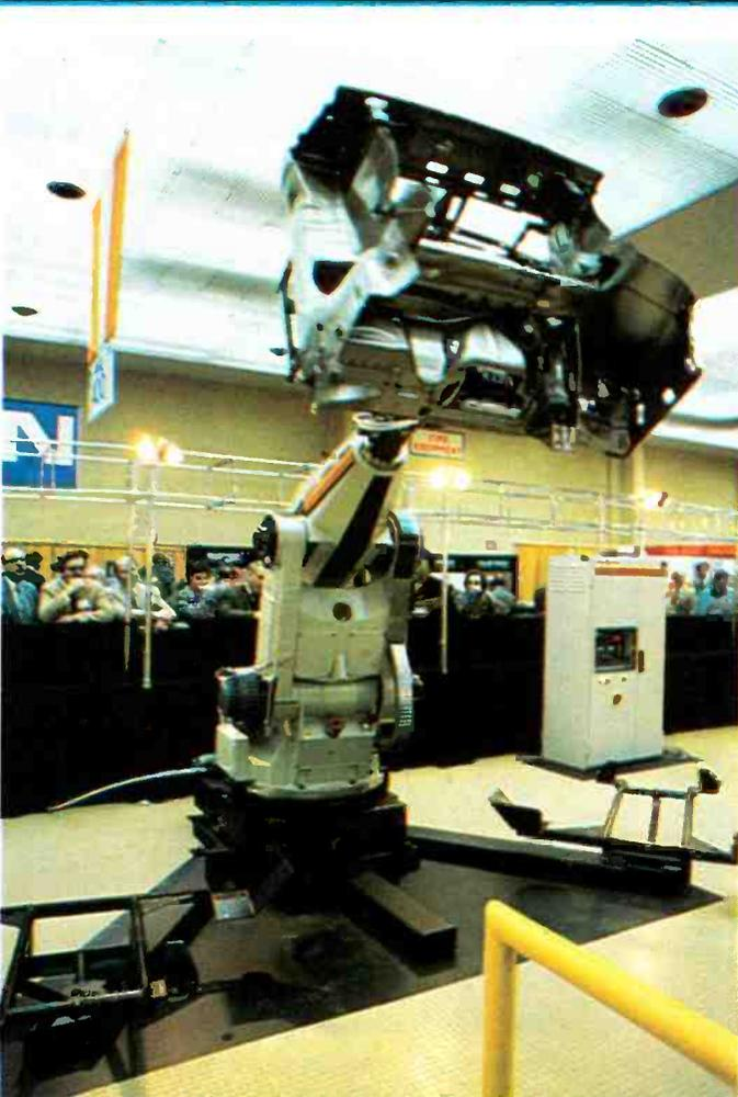
With a payload capacity of 132 pounds, the GP 132, by GE, is suitable for loading and unloading large workpieces.
