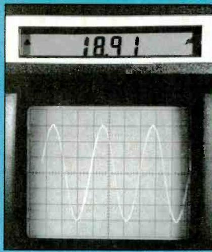
**Figure 13** A sinewave was used (rather than square waves or pulses) to make more clear the process of measuring rise time by Delta-time mode. The amplitude of a locked waveform is adjusted to the 0% and 100% graticule lines, the waveform rise time is horizontally expanded, then the Delta-time mode is selected and the 10% to 90% slope is covered by rotation of the begin and end controls that make this slope brighter. The LCD readout shows a time that needs no processing or calculations.
