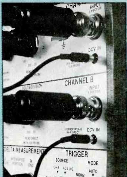
**Figure 7** Below each probe socket on the SC61 front panel is a small banana plug that receives dc voltages from the probe. An optional dc-voltage probe can be plugged in, if the scope probe is not desired (for lower-loading measurements).
