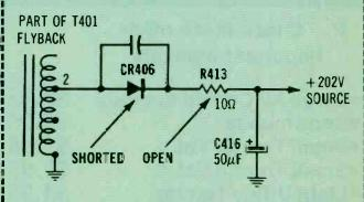
Symptom – Excessive brightness with retrace lines; may shutdown after several seconds
