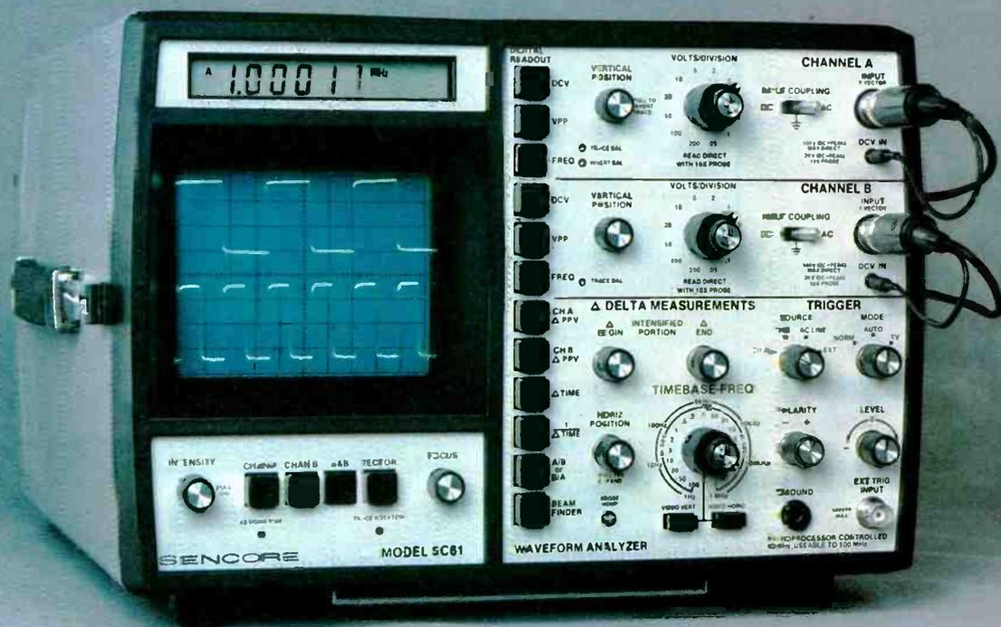
**Figure 1** In addition to many wideband scope features, the Sencore model SC61 has an LCD digital readout that provides two general classes of measurements. Most digital readouts are obtained by pressing one button for each, following the normal scope-waveform adjustments.
