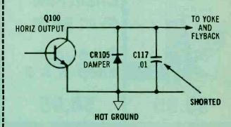
Symptom – Line fuse blows; Q100 output appears to be shorted Cure – Check retrace-tuning capacitor C117 and replace with original type if shorted
