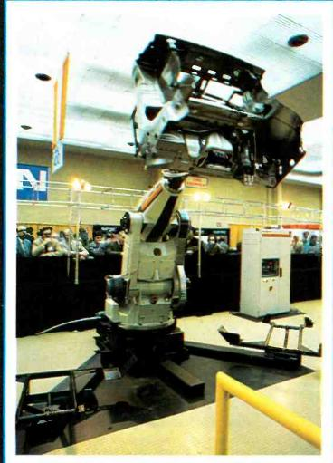
With a payload capacity of 132 pounds, the GP 132, by GE, is suitable for loading and unloading large workpieces.
