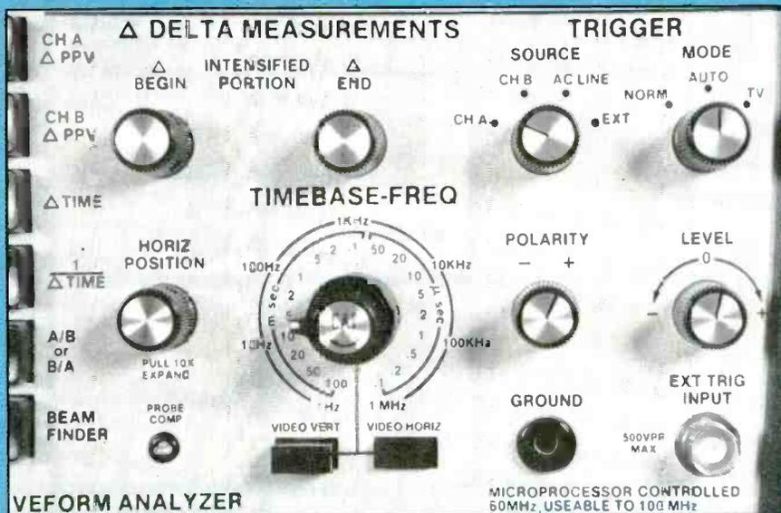
Figure 4 Horizontal-sweep time and triggering controls on the SC61 panel are grouped for easy access.
