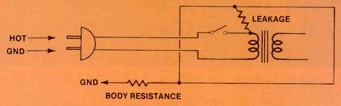
Figure 2. If the switch is in the hot leg, the leakage hazard is removed when the switch is opened.
