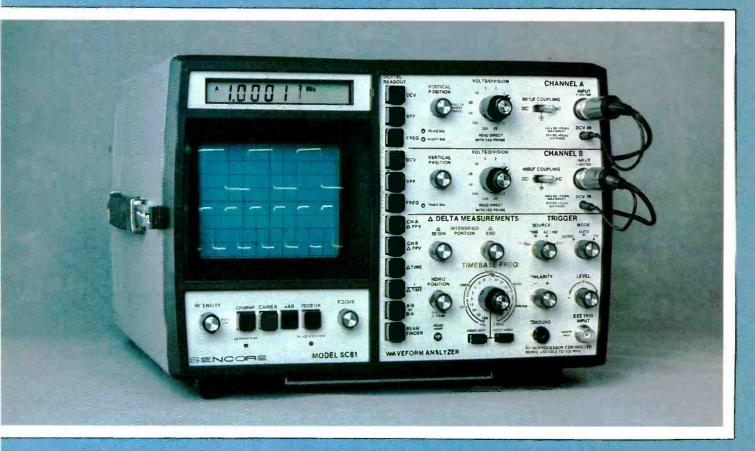
Figure 1 in addition to many wideband scope features, the Sencore model SC61 has an LCD digital readout that provides two general classes of measurements. Most digital readouts are obtained by pressing one button for each, following the normal scope-waveform adjustments.
