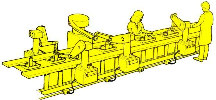
Figure 7. The introduction of robot arms into a conventional indexing assembly line.
