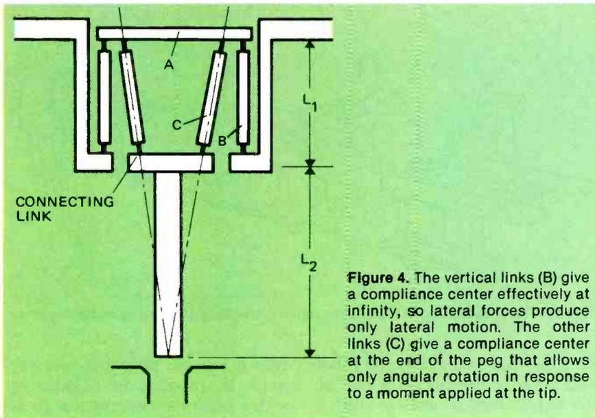
**Figure 4.** The vertical links (B) give a compliance center effectively at infinity, so lateral forces produce only lateral motion. The other links (C) give a compliance center at the end of the peg that allows only angular rotation in response to a moment applied at the tip.
