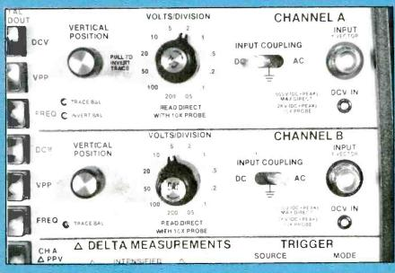
Figure 3 Layout of the vertical-channel controls is shown in this photograph.
