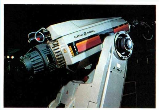
Driven by electric servo motors, the GE robot, GP 132, is a 7-axis, single-arm robot designed for general-purpose material handling.
