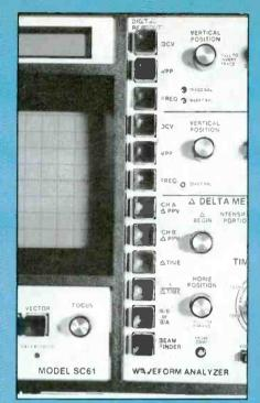
Figure 6 A vertical line of push-buttons is located at about the horizontal center of the front panel. The top six allow digital Vdc, PPac and frequency readouts from the two vertical channels. Four of the lower six buttons are for the Delta-time measurements, one is the frequency-ratio button and the bottom one activates the beamfinder.
