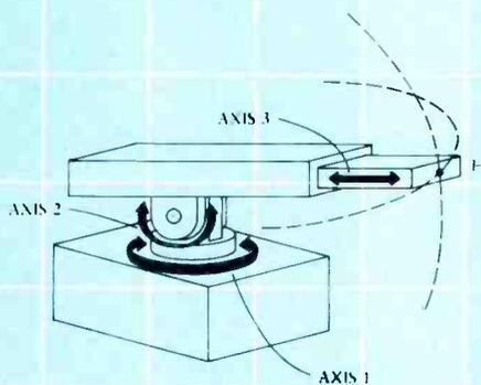
Figure 3. A spherical-coordinate robot.
