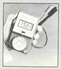
A new addition to its "true hand-size" DMM line, the Triplett model 3400, type 2, 3½-digit, 24-range digital multimeter features improved basic dc accuracy to 0.15%; ac dc voltage measurement to 1000V; 500-hour typical battery life and improved overload protection on all volt and ohm ranges to 1000V without fuse blow, plus protection to 600V on all current ranges.
