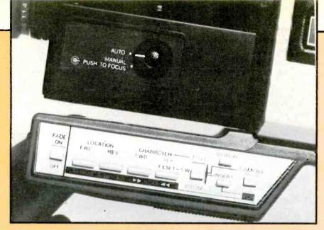
Figure 8 This is a closeup photograph of the operating controls on the 1CVC3035E GE color camera. Functions of fades, character generator and stopwatch are controlled by push-buttons. The portable VCR can be started and stopped from the camera.
