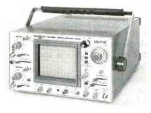
even the most complex signals. With 500µV sensitivity, extremely low level signals can easily be observed. A channel-one output is available on the rear panel to drive other less-sensitive instruments, such as a frequency counter with an input level as low as 500 µV. The dual-time base permits accurate observation and time interval measurements of complex waveforms.
