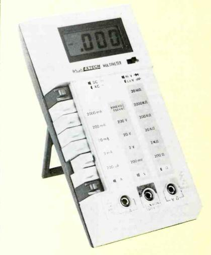
A new hand-held, LCD-display, precision digital multimeter has been introduced by Extech International.
