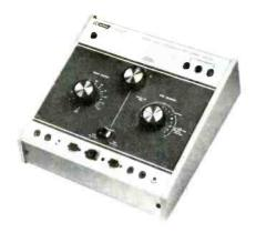
instrument can be used to evaluate bipolar and FET transistors, diodes, SCRs, diacs, triacs and other devices.
