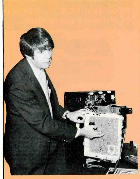
Figure 11 Allen Nelson demonstrated many serviceability features of the new GE PC chassis. The color receiver is shown on its side, with the chassis in the convenient service position.
