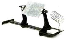
laboratory, prototype and repair work, as well as light production applications. The self-locking end support slides easily to suit board width, and board holders are spring loaded for easy board removal and replacement without re-adjustment. The board may be rotated 360 degrees for access to both sides, and may be locked at any angle for optimum operator efficiency. The unit includes a soldering-iron holder and a tipcleaning sponge.
