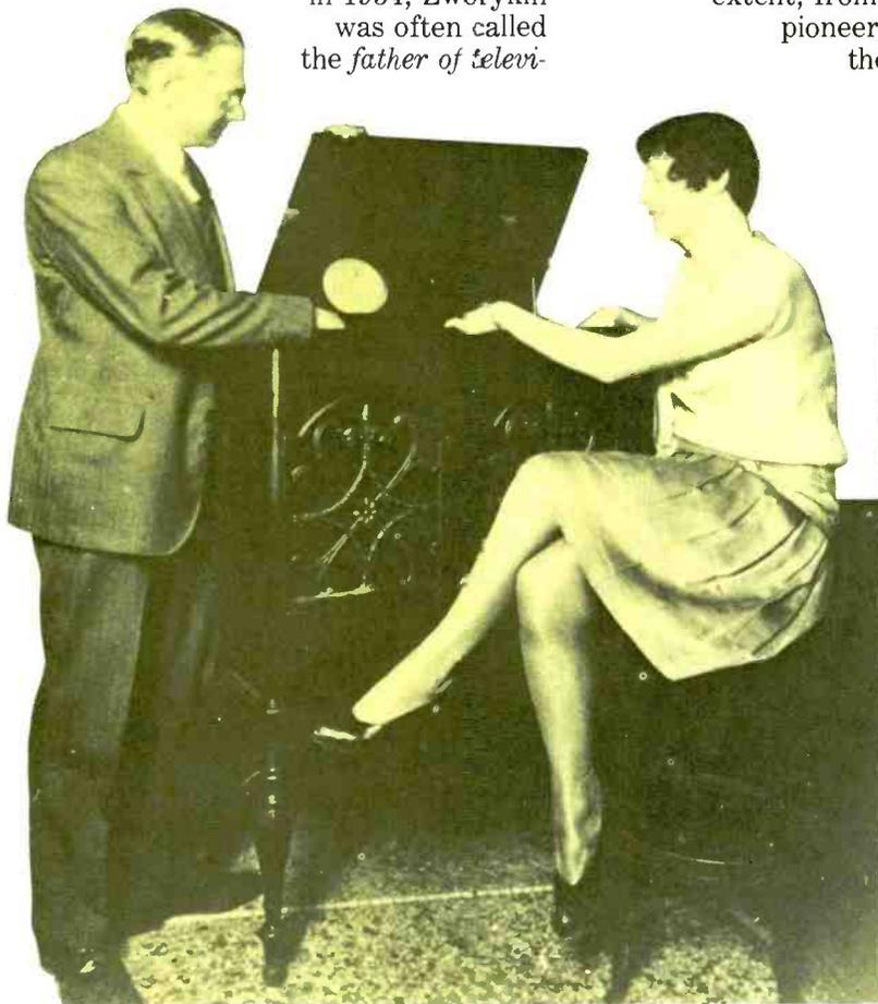
In 1929 Zworykin demonstrated an early electronic TV receiver using the kinescope picture tube.
