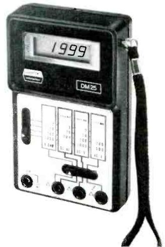
and low-battery indication. An automatic limiter circuit will allow up to 140Vac to be applied on all OHMS ranges without blowing the fuse.
