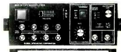
tors and will accept signals of  $\pm 5V$  (10p-p) with a frequency response that is flat to 12MHz, -3db at 20MHz. Input impedance is 1M $\Omega$ .
