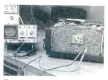
Figure 10. A scope or other instrument that tests capacitors and diodes by the current-versus-voltage method can be used for rapid in-circuit tests to find defective components. A Hameg scope is shown.
