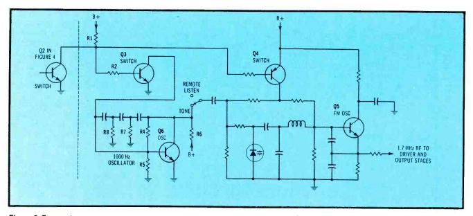
Figure 5. Two actions are necessary when a ringing signal reaches the base station: the 1000Hz oscillator is started and used to modulate the FM carrier that is broadcast to the remote unit; and the transmitter reactance and oscillator stages receive bias. See text for details.
