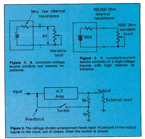
open-loop gain approaches the closed-loop gain. This tells you that you must use an amplifier with a high open-loop gain if you intend to wind up with a reasonably high closed-loop gain.
