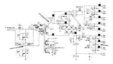
Evidently, an overload was loading down the power transformer. Why didn't the circuit breaker trip? Instead of installing another F3, I temporarily connected a 5A circuit breaker as a substitute. The tubes lighted and all B + voltages were very low. In addition, R254 and R253 were operating so hot that they smoked. I disconnected the three loads at C1A and tested each leg for leakage. Resistance tests proved C1B had a leakage of about 2500 $\Omega$ .
