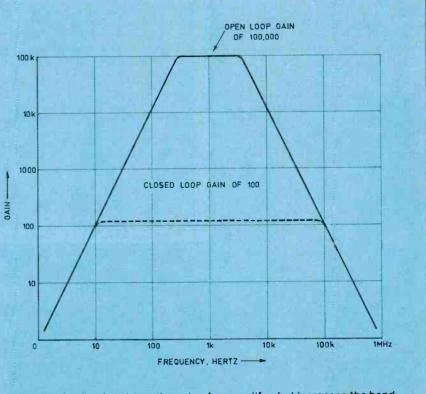
Negative feedback reduces the gain of an amplifer, but increases the bandwidth
