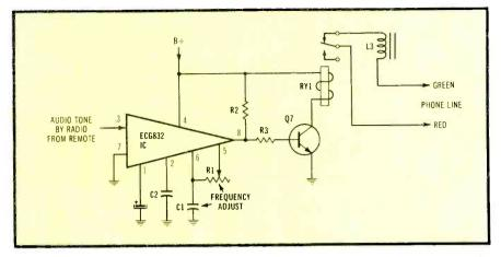
**Figure 6.** Capturing (locking) a phone line for an outgoing call from the remote unit requires inductance L3 to be connected across the phone line. An audio tone is transmitted from the remote unit to the base station.
