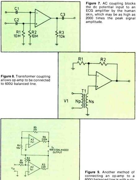
$600\Omega$  balanced line is with a circuit such as this.
