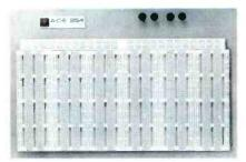
The ACE 245 features a universal matrix of 4488 solderless plugin tie-points, and is composed of 640 separate 5-tie-point terminals, 40 vertical distribution buses, and 4 horizontal buses. For larger projects, the ACE 254 combines the plug-in ease of a 0.1" x 0.1" solderless matrix with the convenience of 768 separate distribution buses of 5-tie-points each, plus 4 horizontal buses.
