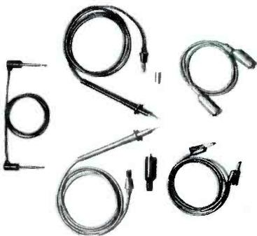
The test prods have molded flanges for protection against electrical shock, anti-slip ribs for better grip, and tips that are threaded to accept spade lugs or alligator clips. The meter input end of the test prods have shrouded standard banana plugs for maximum protection, and tapered back ends and anti-slip ribs for a good gripping
