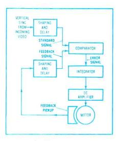
Figure 2. This block diagram demonstrates the operation of a typical VCR servo. The conditions shown are for head-cylinder speed control during recording, but a change of the standard-signal source or the feedback-signal source allows it to operate equally well during playback, or as a capstan servo. Notice the similarities to the horizontal phase detector in a color receiver, and to phase-locked loops (PLLs).
