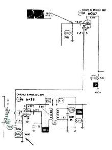
These replacements restored normal brightness, giving a good picture. Now the blanker grid measured -81V and the common cathodes reading was +2.8V. These voltages were within normal tolerance. This repair shows the importance of understanding how the horizontal-blanking pulses are applied to the -Y amplifier grids, where they are rectified to produce negative grid bias, and which affects the brightness. Also, the same grid pulses produce negative-going blanking pulses at the CRT grids.
