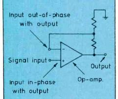
An op-amp is a low cost versatile amplifier with the advantage that the input and the feedback may be isolated from one another.
