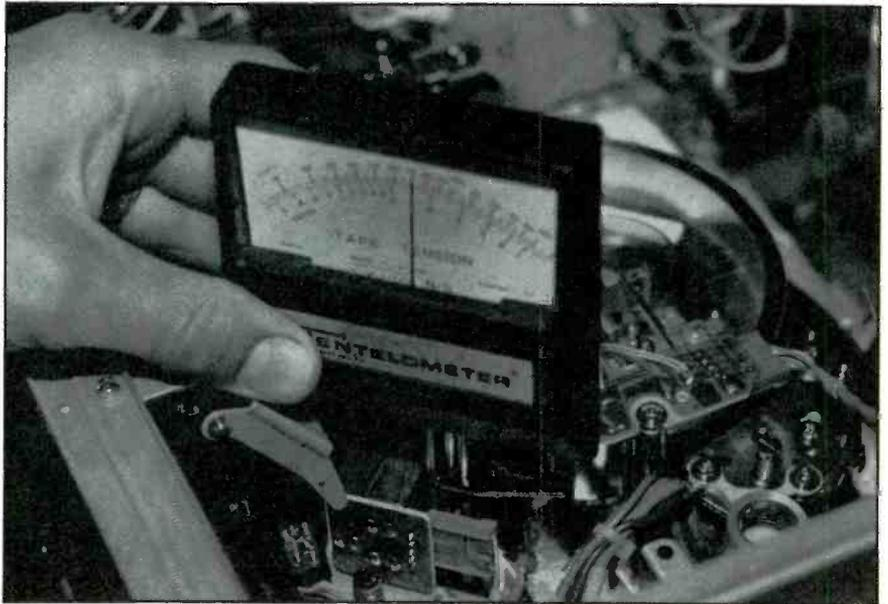
Adjusting tape tension on a Sony U-matic Type V unit. (Photo courtesy of Tentel.)
