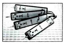
(HTL, DTL, TTL, CMOS) to detect common digital faults such as open circuits, tri-state modes, nodes stuck at high or low, intermittent and/or normal pulse activity. The probes afford pulse detecting capability of 10ns with memory and pulse hold, high speed testing capability of 100MHz, buffered inputs and outputs for reverse polarity and high voltage protection, stainless steel probe tips and dual-threshold operation.
