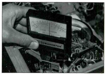
Adjusting tape tension on a Sony U-matic Type V unit. (Photo courtesy of Tentel.)
