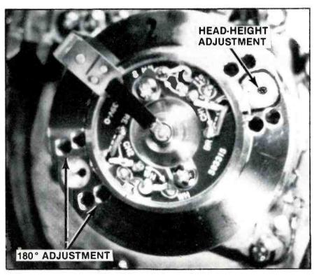
Hole on top of head is used for head-height adjustment. Holes on either side of head are used for 180° adjustment. It is important to mark the head you are adjusting in order to avoid confusion.
