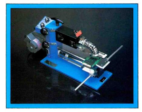
tube when the machine is turned on. Components adjacent to the failed component are not susceptible to degradation or damage because the removal temperature used does not exceed the reflow temperature used during the manufacturing process.
