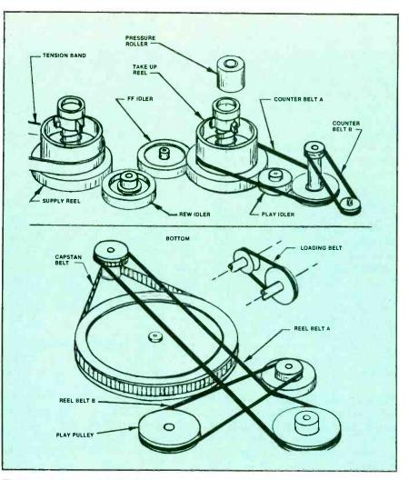
**Figure 1.** In the early VCR designs, the functions of *rewind*, *fast forward* and *play* were done by a series of main and intermediate idlers. This more costly scheme spread the stress over a greater number of components.
