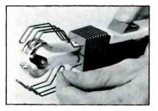
The unit incorporates quartz encapsulated heating elements that open and close like a thumb and forefinger, to encircle the work piece with instant infrared heat, variable in temperature up to 1500°F. The interchangeable plugin elements are gold plated to focus heat toward the center of the work piece. They are available in 1-inch, 2-inch, 3-inch and now, in the new ½-inch diameters that are suitable for small work pieces. Circle (75) on Reply Card
