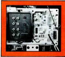
Figure 7. An arrow shows where J23 is located. The digital *high* and *lows* for J23 are produced by the A/V off and A/V on positions. One control voltage always should be zero and the other about + 11.8V. These control voltages simultaneously supply switching for video and audio signals. If J23 is removed, the TV sound is missing and there apparently is AGC overload.
