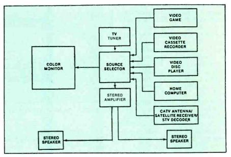
Figure 2. Combined video/audio systems. (Courtesy Zenith Radio Corp.)
