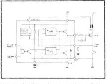
**Figure 1.** The circuit design of the TDA8140 has been simplified, yet current dissipation has been reduced. Control/protection functions are built in.
