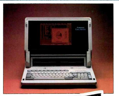
ing costs and size restrictions of ac gas-plasma displays have prevented their use in most microcomputer applications. Panasonic overcame major plasma technological and manufacturing challenges in order to incorporate a plasma display with its new Exec. Partner. Although it is only 2-inches thick, the 11-inch (CRT equivalent) screen displays 25 lines by 80 columns of high-resolution viewing.
