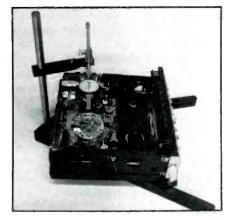
Head protrusion gauge, HPG-1, with accessory stand for checking head protrusion on a portable VHS deck. (Photo courtesy of Tentel.)
