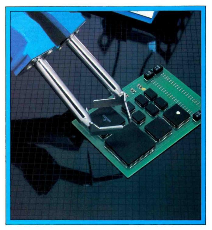
component by lingering too long on the component with the heated probe.
