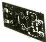
**NEW MM-40A** — The ideal single line termination filter for use at set or converter having separate terminals for UHF and VHF. Patented\* printed circuit.
