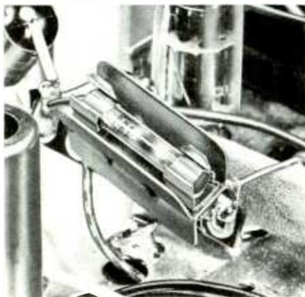
Fig. 2. Snap-on Fuse Holder
