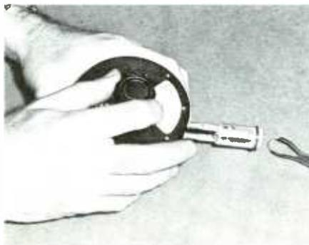
Fig. 1. Grid-Dip Meter Being Used to Measure Electrical Length of Transmission Line.
